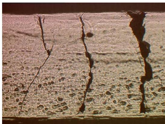
Figure 7: Magnified image of transverse cracks along an edge of a cross-ply laminate.
