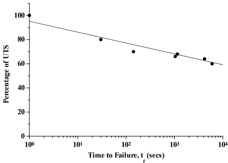
Figure 24: Stress rupture of 3 mm wide unidirectional E-glass/F922 in air.
