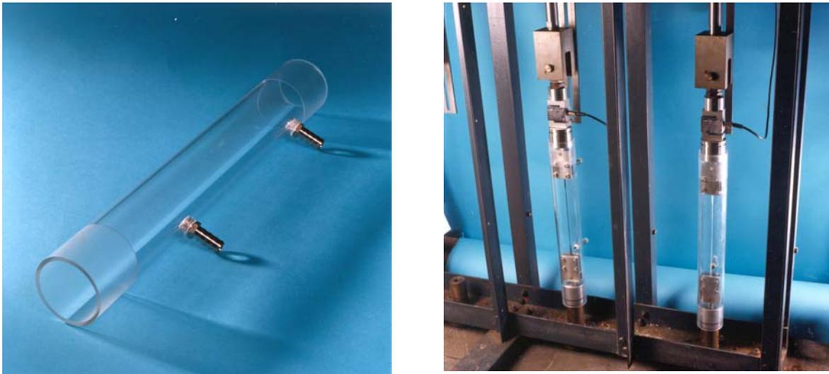
**Figure 21: Long-term environmental fatigue apparatus.**
