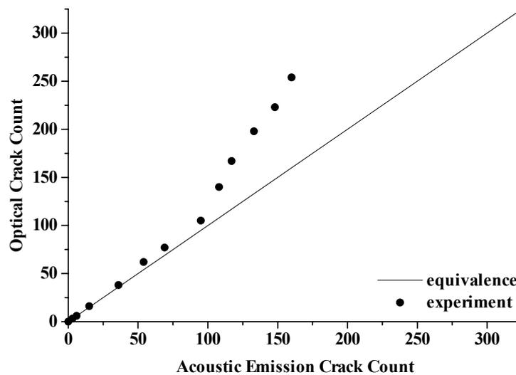
Figure 10: Comparison of optical and AE crack count data for  $[0/90_4]_s$  E-glass/F922.
