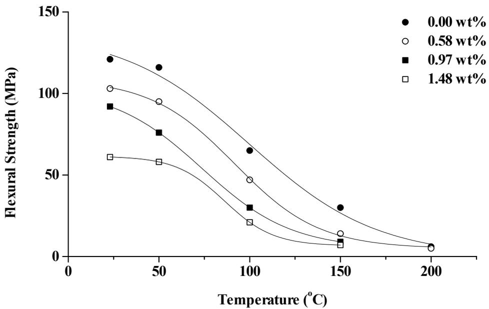
Figure A2: Transverse flexural properties of conditioned E-glass/913 with temperature.
