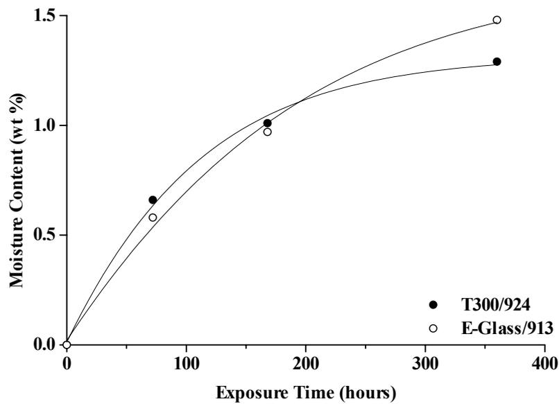
Figure 16: Moisture absorption of longitudinal E-glass/913 and T300/924 specimens.
