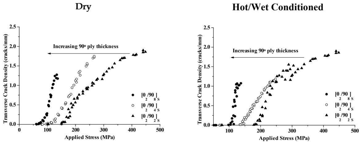
**Figure 12: Crack density as a function of applied stress for E-glass/F922 laminates.**
