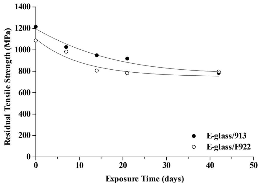
Figure 4: Longitudinal tensile strength of hot/wet conditioned glass/epoxy laminates.
