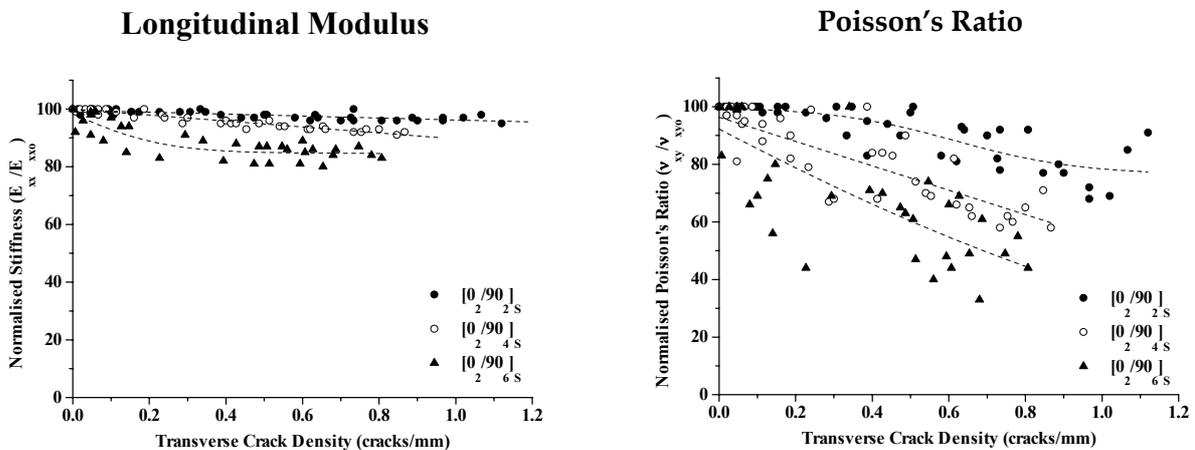
**Figure 15: Elastic property reduction in HTA/F922 laminates. (lines added as a visual aid to show trends)**
