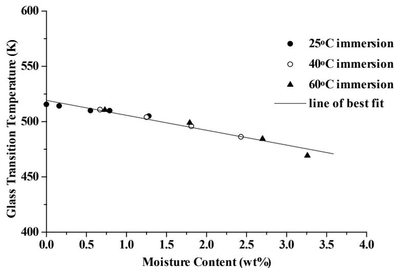
Figure 3: Glass transition temperature of F922 as a function of moisture content.
