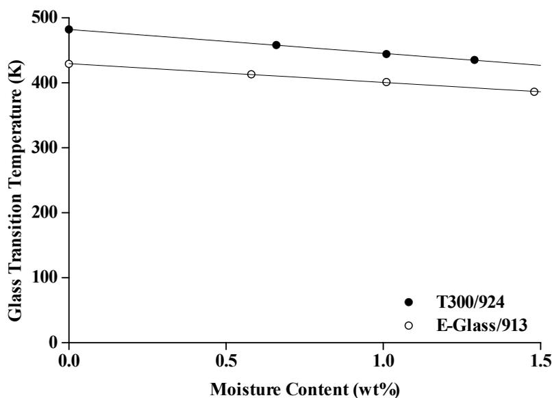
Figure 17: Glass transition temperature for hot/wet conditioned E-glass/913 and T300/924.
