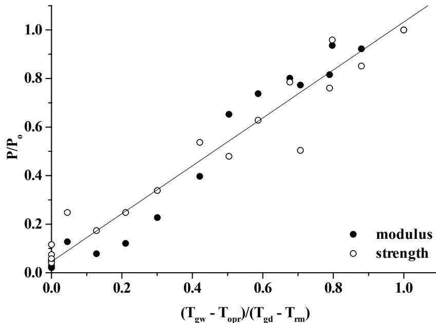
Figure 18: Transverse flexure properties of unidirectional E-glass/913.
