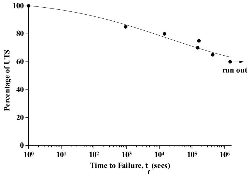
Figure 23: Stress rupture of unconditioned cross-ply E-glass/913 in air.
