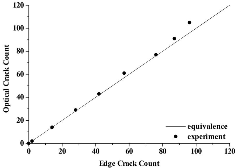
Figure 8: Comparison of edge crack and optical crack counts for  $[0/90_2]_s$  E-glass/F922.
