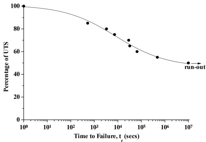
**Figure 22: Stress rupture of unconditioned unidirectional E-glass/F922 in air.**
