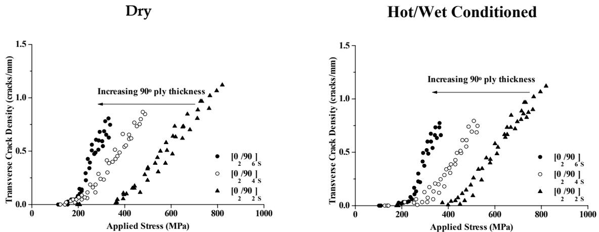
**Figure 13: Crack density as a function of applied stress for HTA/F922 laminates.**
