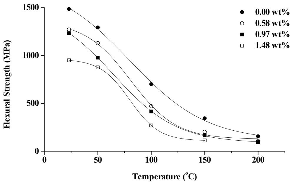
Figure A1: Longitudinal flexural properties of conditioned E-glass/913 with temperature.
