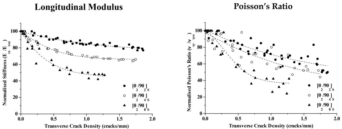
**Figure 14: Elastic property reduction in E-glass/F922 laminates. (lines added as a visual aid to show trends)**
