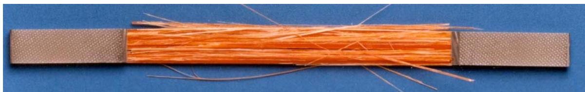
**Figure 5: Typical tensile failure for unidirectional E-glass/913 laminate.**
