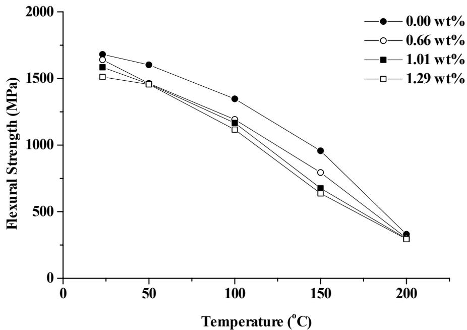
Figure A3: Longitudinal flexural properties of conditioned T300/924 with temperature.
