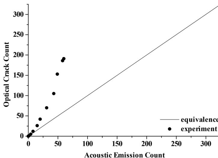
Figure 11: Comparison of optical and AE crack count data for  $[0/90_8]_s$  E-glass/F922.
