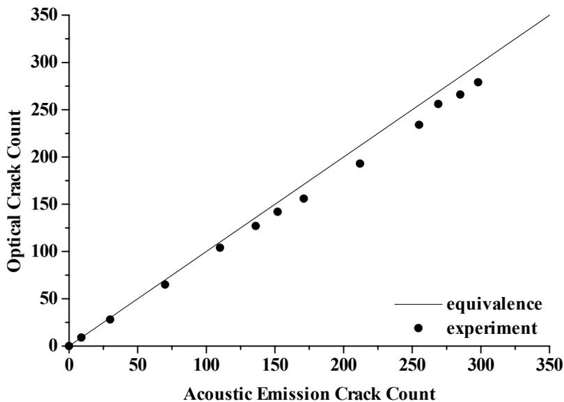
Figure 9: Comparison of optical and AE crack count data for  $[0/90_2]_s$  E-glass/F922.
