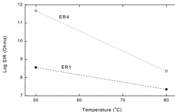
Figure 15: A comparison of the predicted log SIR behaviour of encapsulants ER1 and ER4 on a flexible substrate as a function of temperature under humid conditions.
