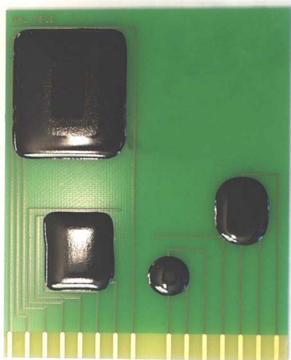
Figure 2 : An example of a urethane based glob top dispensed on to a ceramic board coated with solder resist. Note that the glob tops not only cover the double comb areas but also their immediate vicinity i.e. the solder resist coated ceramic.
