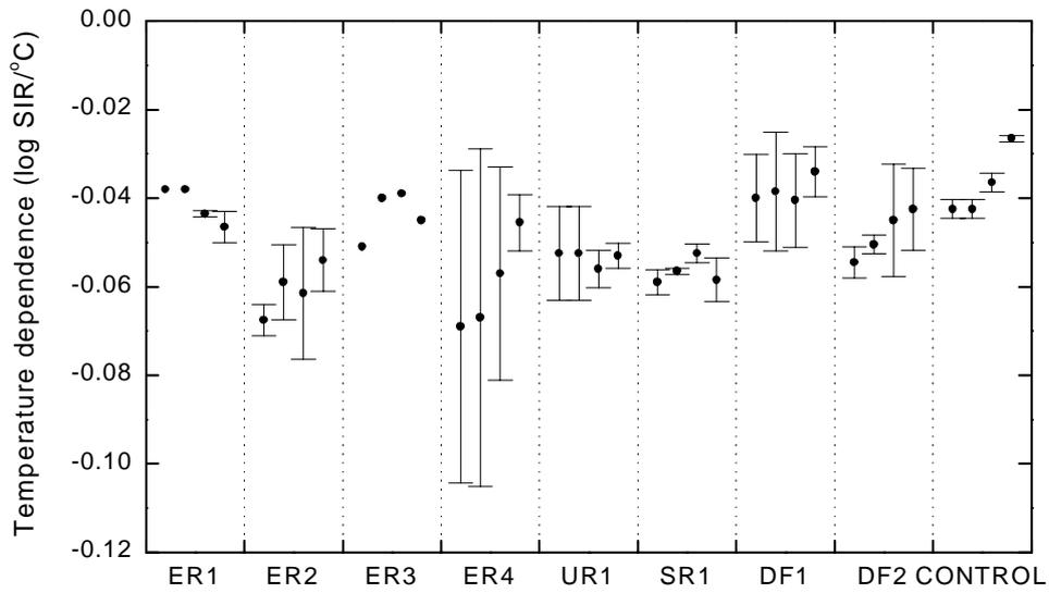
Figure A3 : The temperature dependence of log SIR under damp conditions for **resist coated FR-4** (the control). The key to the data is given in the legend to Figure 8.
