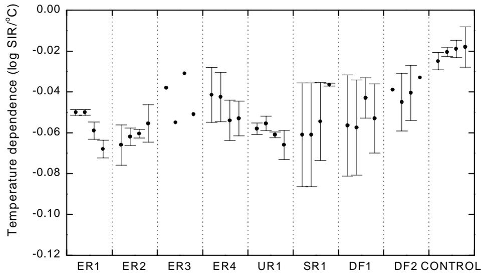
Figure A4 : The temperature dependence of log SIR under damp conditions for **resist coated ceramic** (the control). The key to the data is given in the legend to Figure 8.
