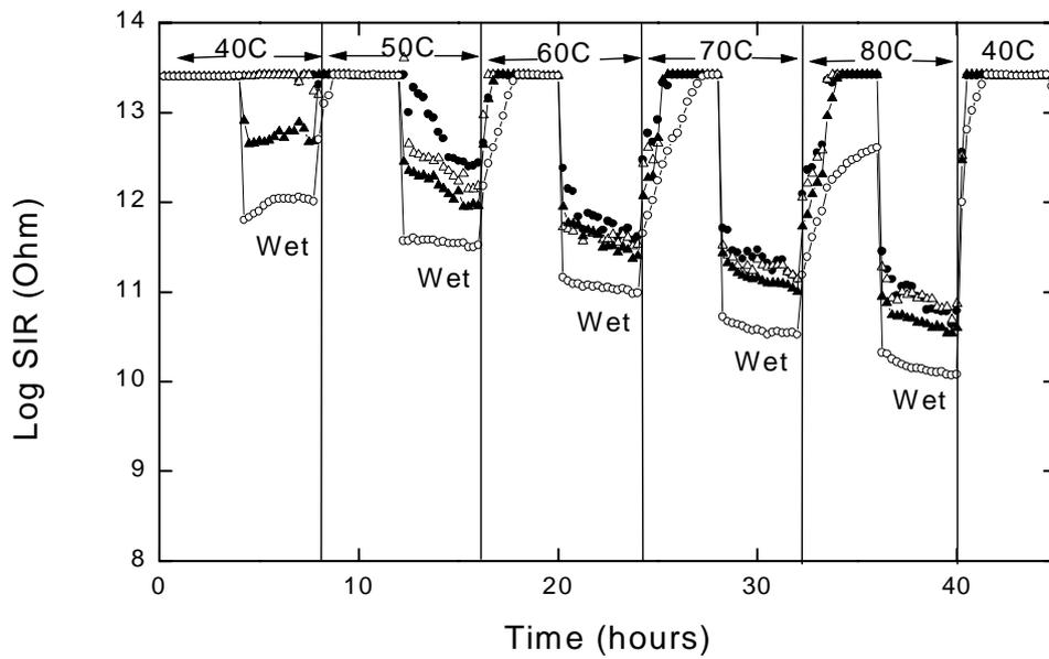
Figure 5 : Log SIR for bare double combs deposited on to FR-4 reflects the changes in humidity that occur with each temperature increment. The magnitude of log SIR depends on the area of the double comb (○ = pattern 1, ▲ = pattern 2, △ = pattern 3, ● = pattern 4).
