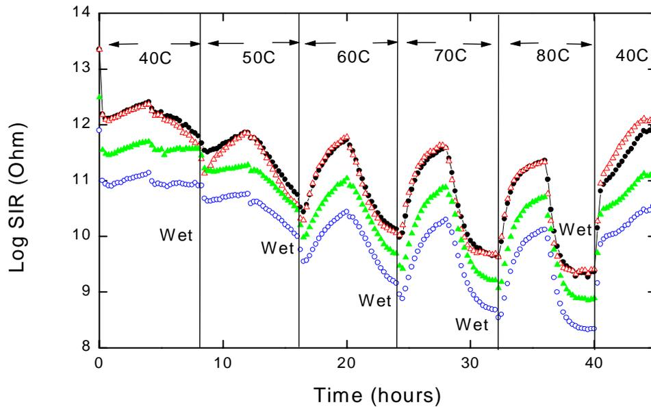
Figure 18 : UR1 deposited on ceramic behaves as a ‘semipermeable’ material becoming increasingly sensitive to changes in humidity with increasing temperature. (○ = pattern 1, ▲ = pattern 2, △ = pattern 3, ● = pattern 4).
