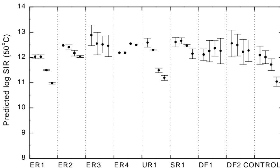
Figure 9 : A plot of the predicted value for log SIR at 50°C for different types of encapsulant deposited on to FR-4 substrate (the control). The four points per material represent the data from combs 4 to 1 in this sequence. Each datum is an average value from two identical patterns on different boards.
