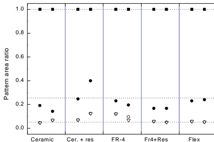
Figure 14: A comparison of the pattern ratios based on the predicted values of log SIR at 50 °C for bare patterns on different substrates. (■ = pattern 1, ● = pattern 2, ▽ = pattern 3, ○ = pattern 4).
