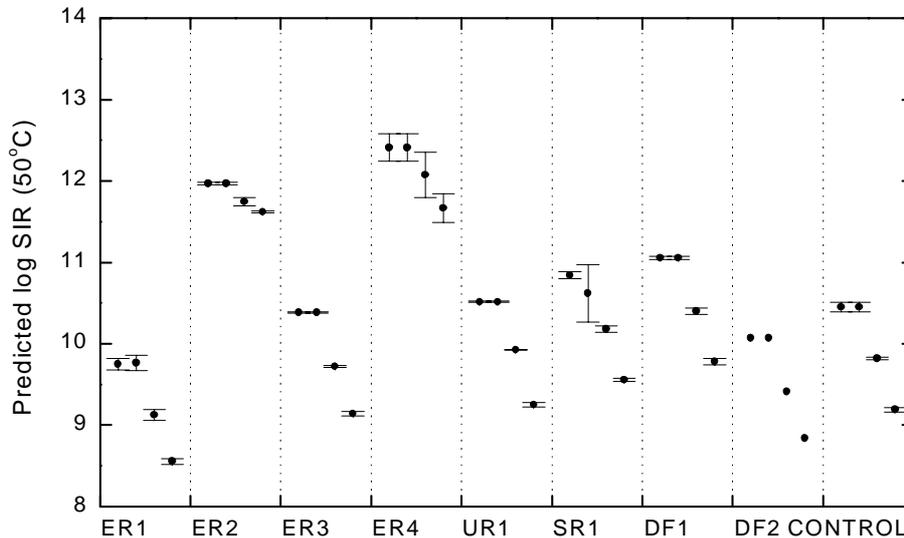
Figure 10 : A plot of the predicted value for log SIR at 50°C for different types of encapsulant deposited on to a flexible substrate (the control). The four points per material represent the data from combs 4 to 1 in this sequence. Each datum is an average value from two identical patterns on different boards.
