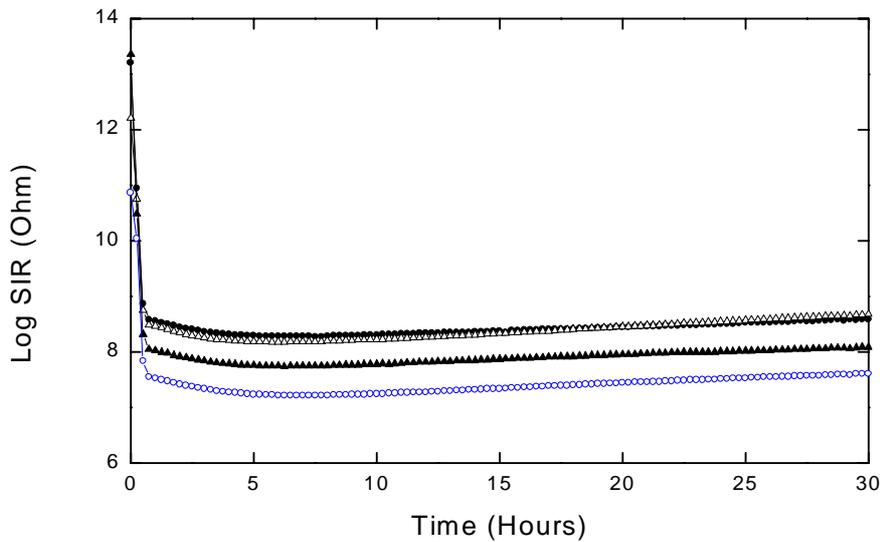
Figure 17 : The SIR of the ER1 deposited on to ceramic rapidly reaches a stable value within approximately 1 hour after exposure to 85 %R.H. and 85°C. ( $\circ$  = pattern 1,  $\blacktriangle$  = pattern 2,  $\triangle$  = pattern 3,  $\bullet$  = pattern 4).
