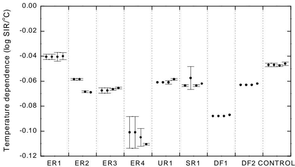
Figure 13. The temperature dependence of log SIR for flexible polyimide (the control) under damp conditions. These are linked with the predicted log SIR values shown in figure 10.
