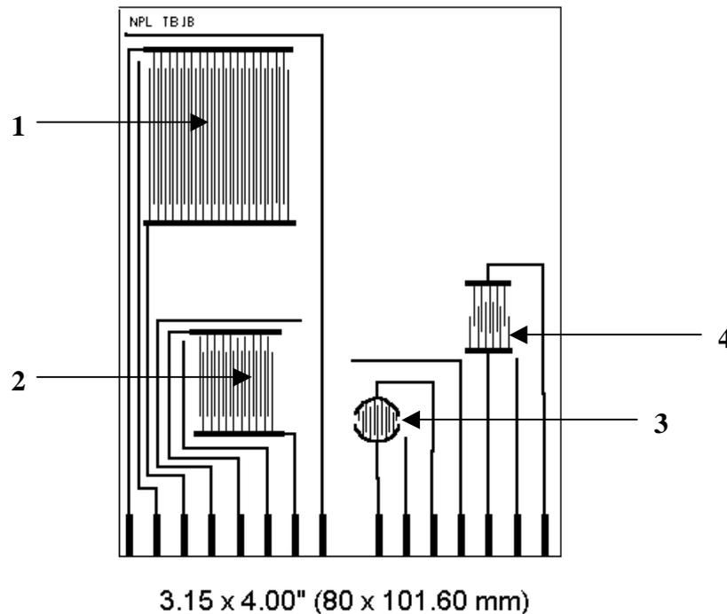
Figure 1: The test board comprises of four double comb patterns labelled 1 to 4.
