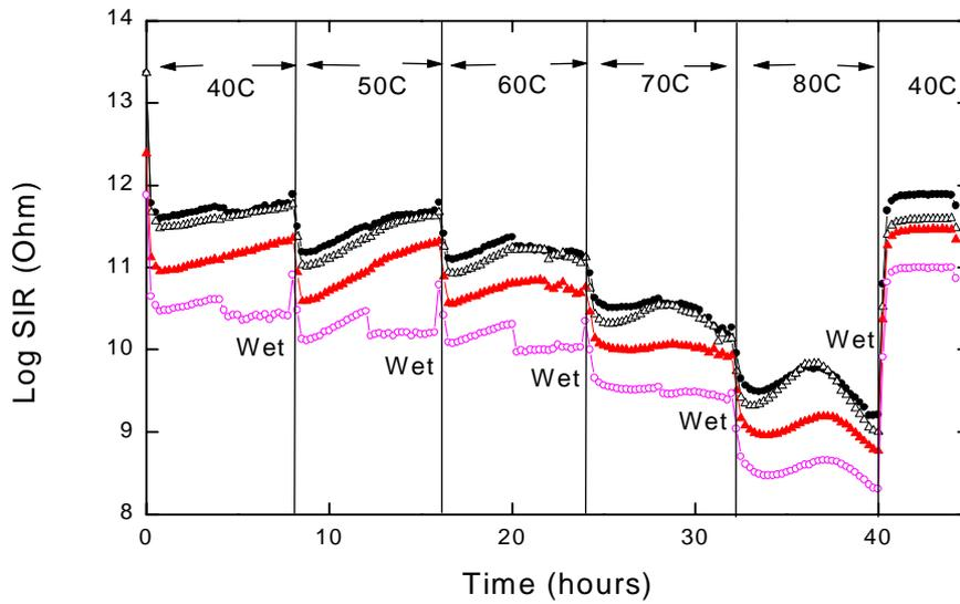
Figure 16 : ER1 deposited on to ceramic appears to be ‘moisture resistant’ i.e insensitive to changes in humidity over a relatively wide temperature range. ( $\circ$  = pattern 1,  $\blacktriangle$  = pattern 2,  $\triangle$  = pattern 3,  $\bullet$  = pattern 4).
