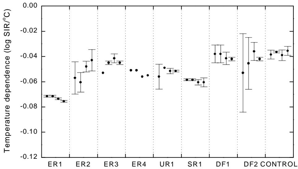
Figure 11. The temperature dependence of log SIR for FR-4 board (the control) under damp conditions. These are linked with the predicted log SIR values shown in figure 9
