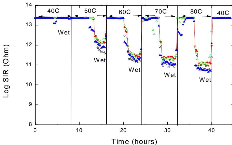
Figure 7: A typical plot of log SIR versus time obtained for a glob top (epoxy based) deposited on to a ceramic board. The environmental conditions are indicated on the figure. The humidity cycles between 10% RH (the first two hours at each temperature) and 90% RH (shown as 'wet'). (○ = pattern 1, ▲ = pattern 2, △ = pattern 3, ● = pattern 4).
