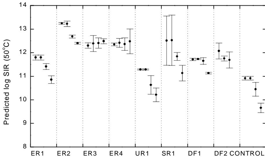
Figure 8 : A plot of the predicted value for log SIR at 50°C for different types of encapsulant deposited on to a ceramic substrate (the control). The four points per material represent the data from combs 4 to 1 in this sequence. Each datum is an average value from two identical patterns on different boards.
