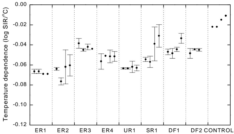
Figure 12. The temperature dependence of log SIR for ceramic board (the control) under damp conditions. These are linked with the predicted log SIR values shown in figure 8
