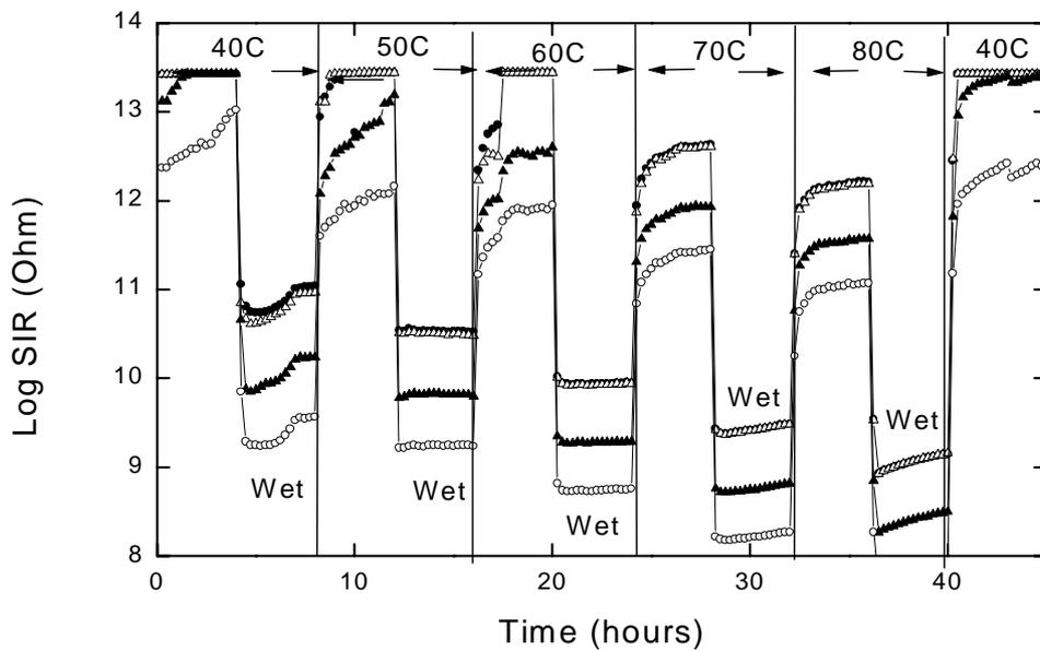
Figure 6 : Log SIR for bare double combs deposited on to flex (polyimide) reflects the changes in humidity that occur with each temperature increment. The magnitude of log SIR depends on the area of the double comb (○ = pattern 1, ▲ = pattern 2, △ = pattern 3, ● = pattern 4).
