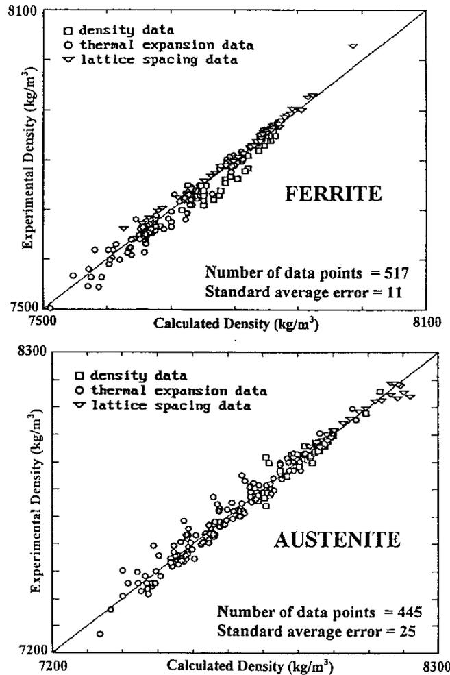
Figure 4 Fit of experimental data for the density of ferritic and austenitic steels by Miettinen
