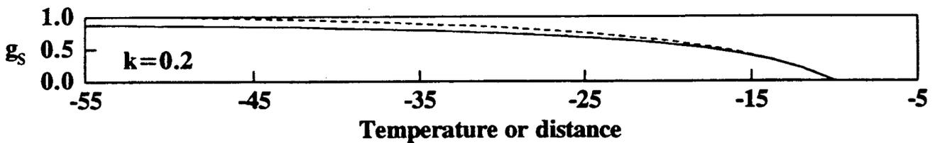
Fig A2 Plot of fraction solid as a function of temperature/distance assuming the Scheil equation (filled line) and the lever rule (dotted line).
