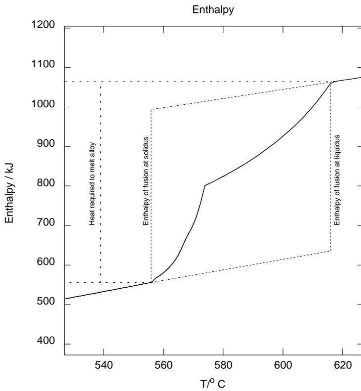
Figure 2 Calculated enthalpy curve associated with the fusion of a multicomponent alloy
