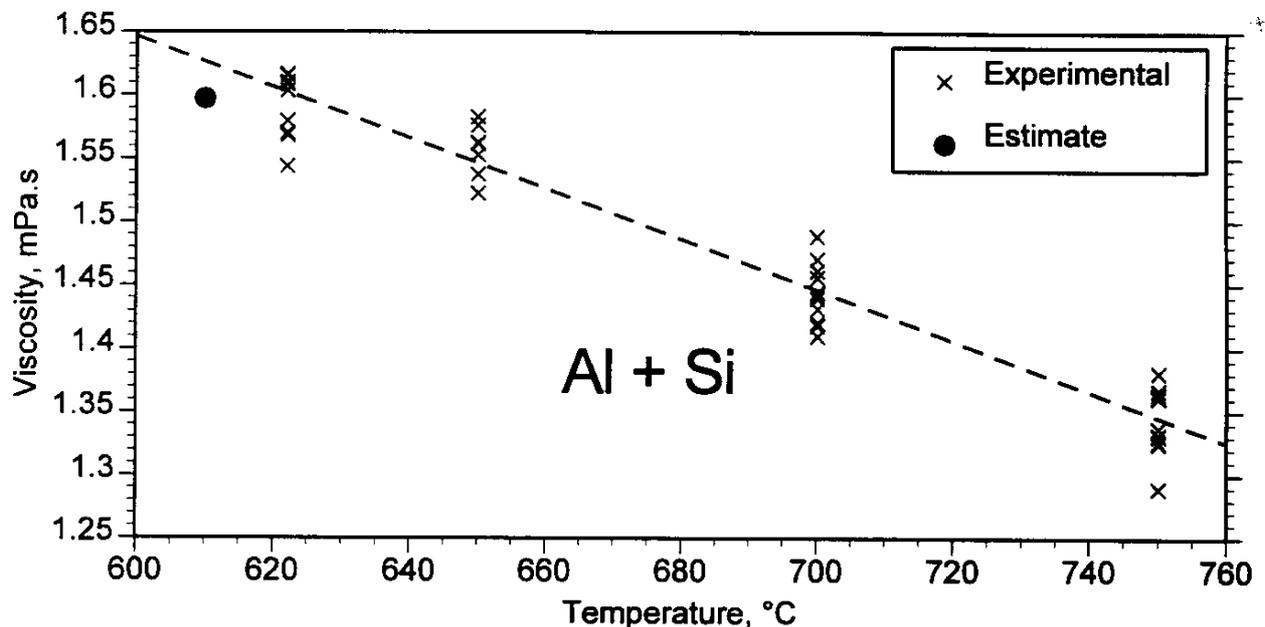
Figure 5 Viscosities of Al+Si alloy as a function of temperature
