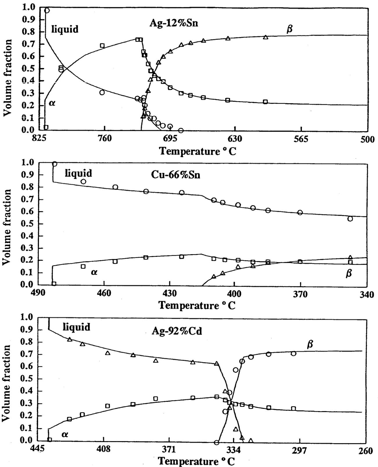
Fig A8 Experimental fraction of the phases shown in figure 5 (points) to be compared with those calculated using "Alloy" [4] (lines).
