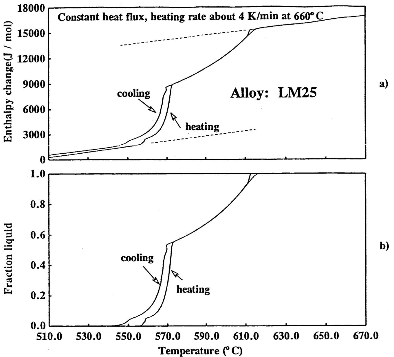
Fig A6 Results for LM25 measured using a single-pan DSC [15] a) Measured enthalpies. b) Estimated fraction solid.
