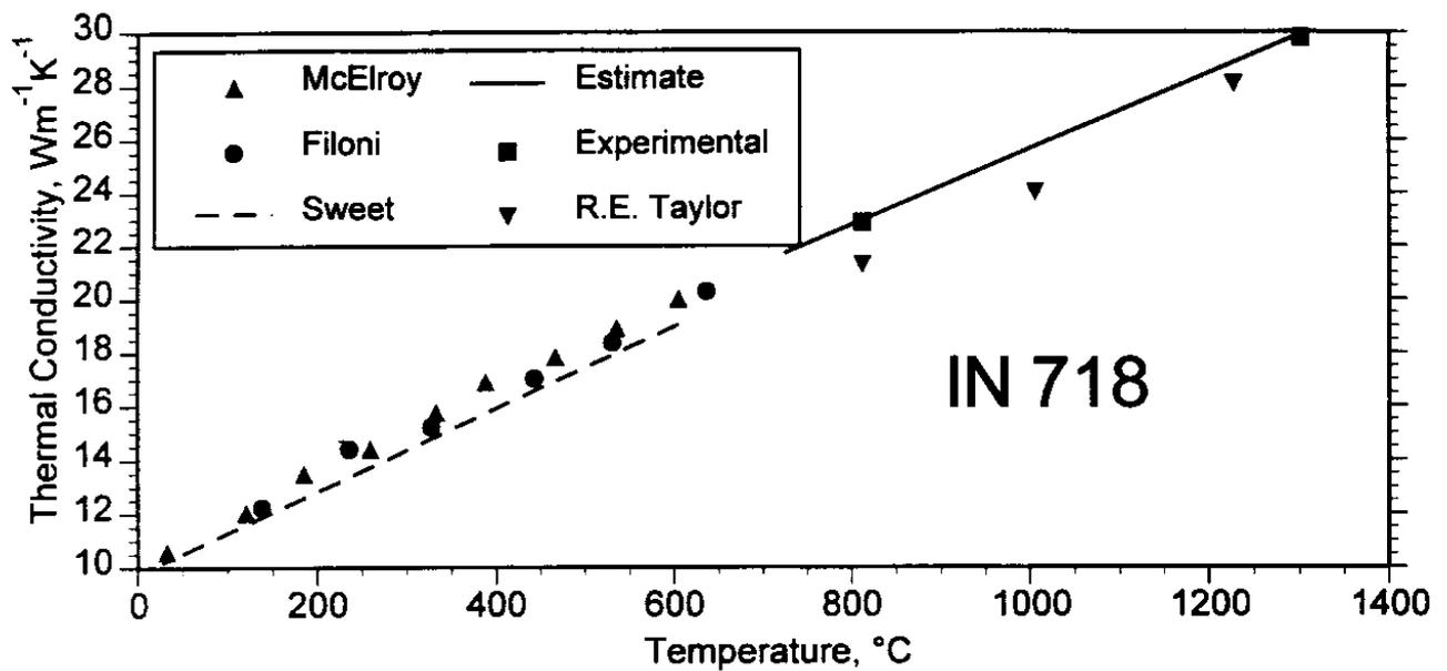
Figure 9 Thermal conductivities of Ni-based superalloy IN718 as a function of temperature with experimental points superimposed
