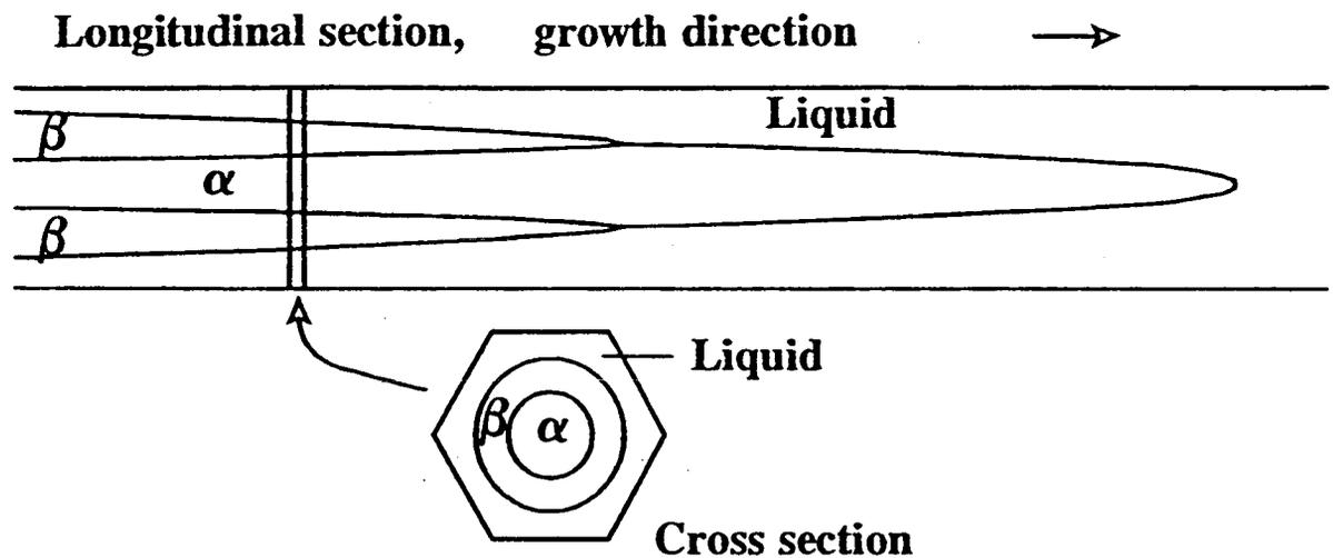
Fig A7 Schematic diagram showing section treated in the numerical model.
