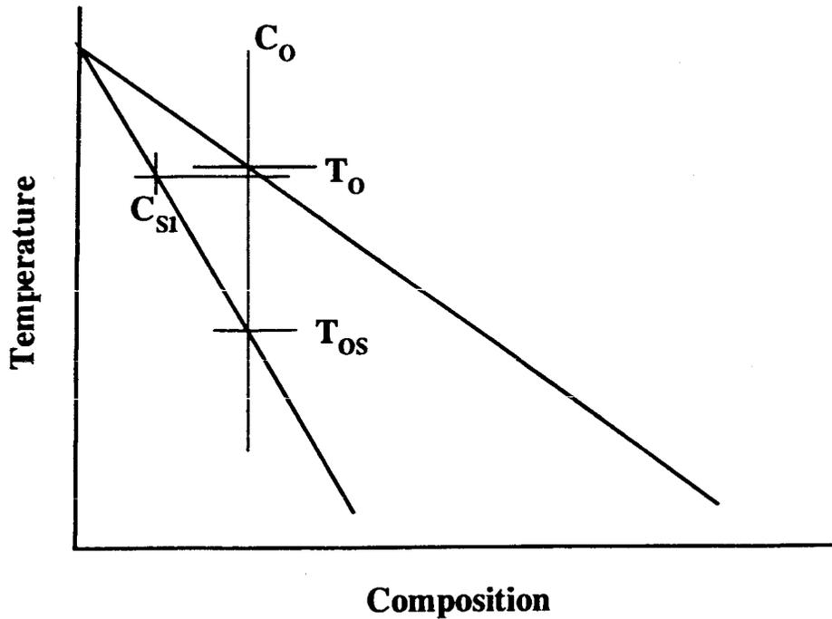
Fig A1 Schematic phase diagram showing liquidus  $T_0$ , solidus  $T_{OS}$  for composition  $C_0$ .
