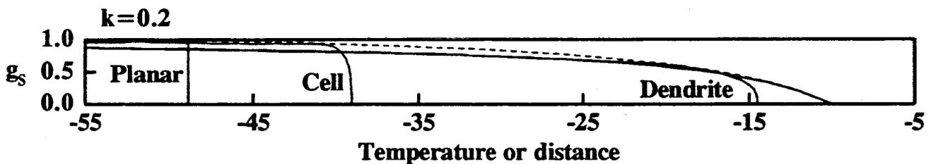
Fig A3 Plot of fraction solid as a function of temperature/distance assuming no diffusion in the solid for the Scheil equation, a dendrite, a cell and a planar front.
