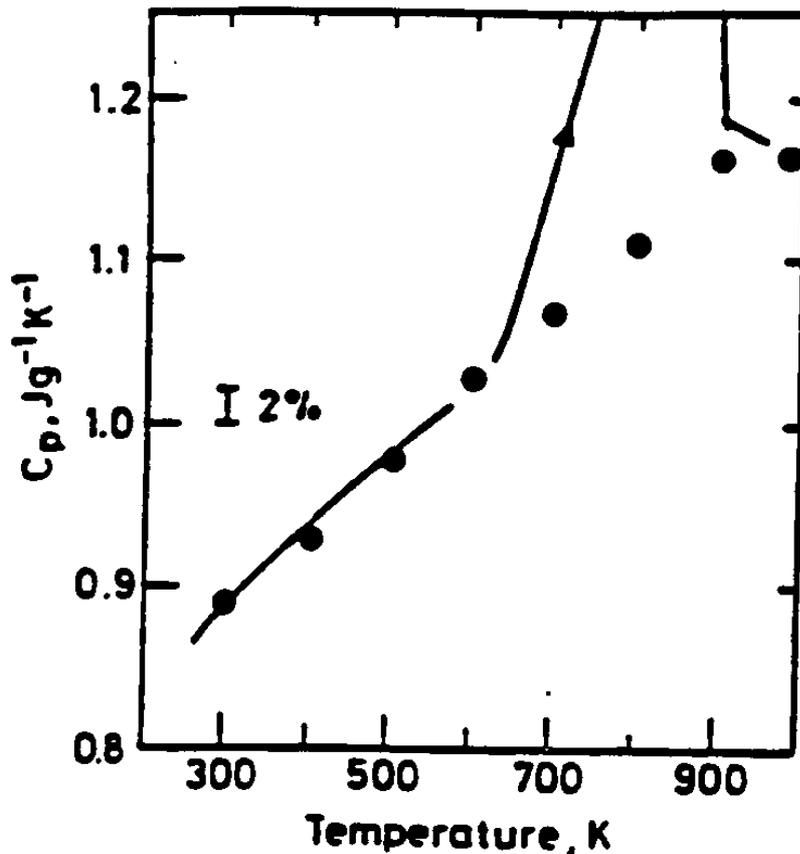
Figure 1 Heat capacity of Al + Si alloy as function of temperature; The symbols indicate measured values, the solid curve indicates estimated values.
