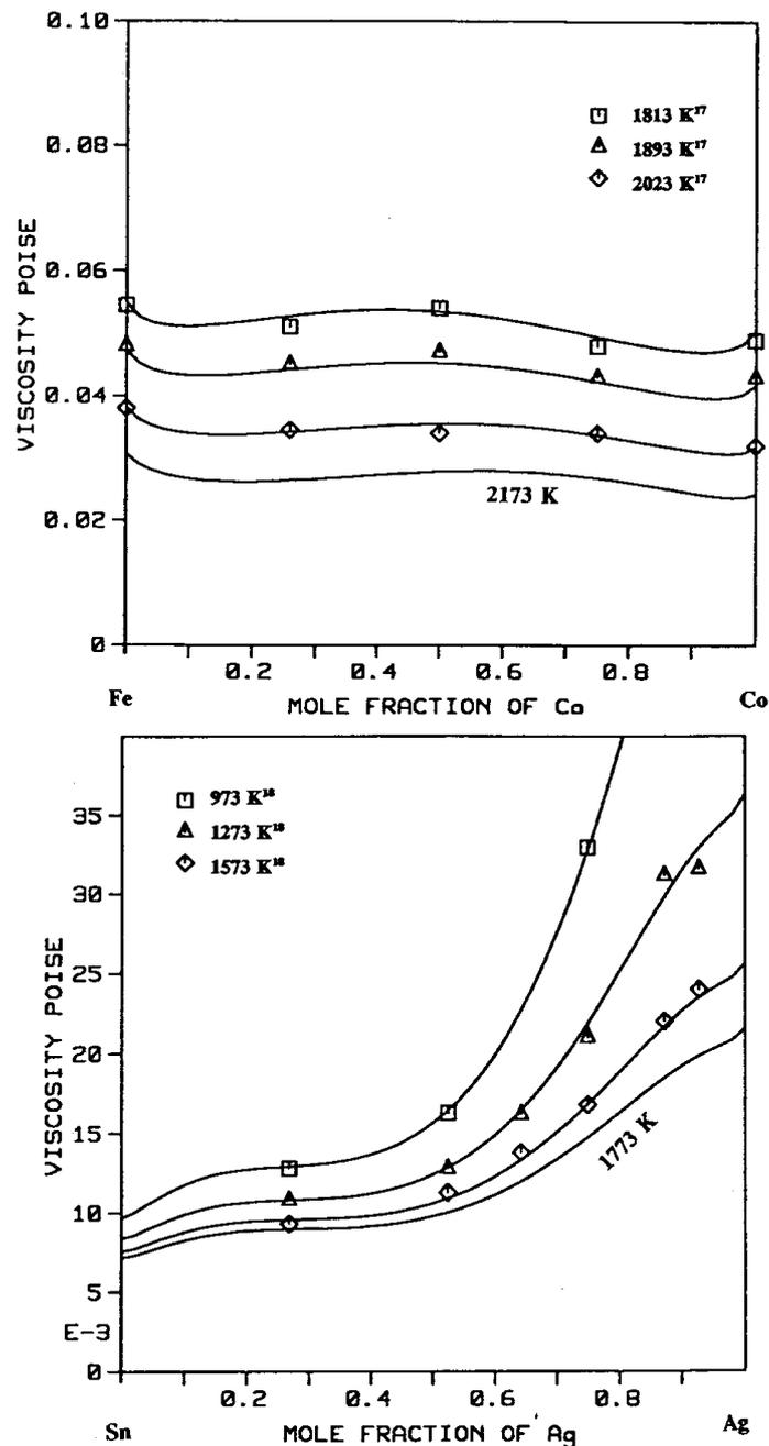
Figure 6. A comparison between calculated and experimental viscosities for the Co-Fe and Ag-Sn systems from Seetharaman et al (94see/du).
