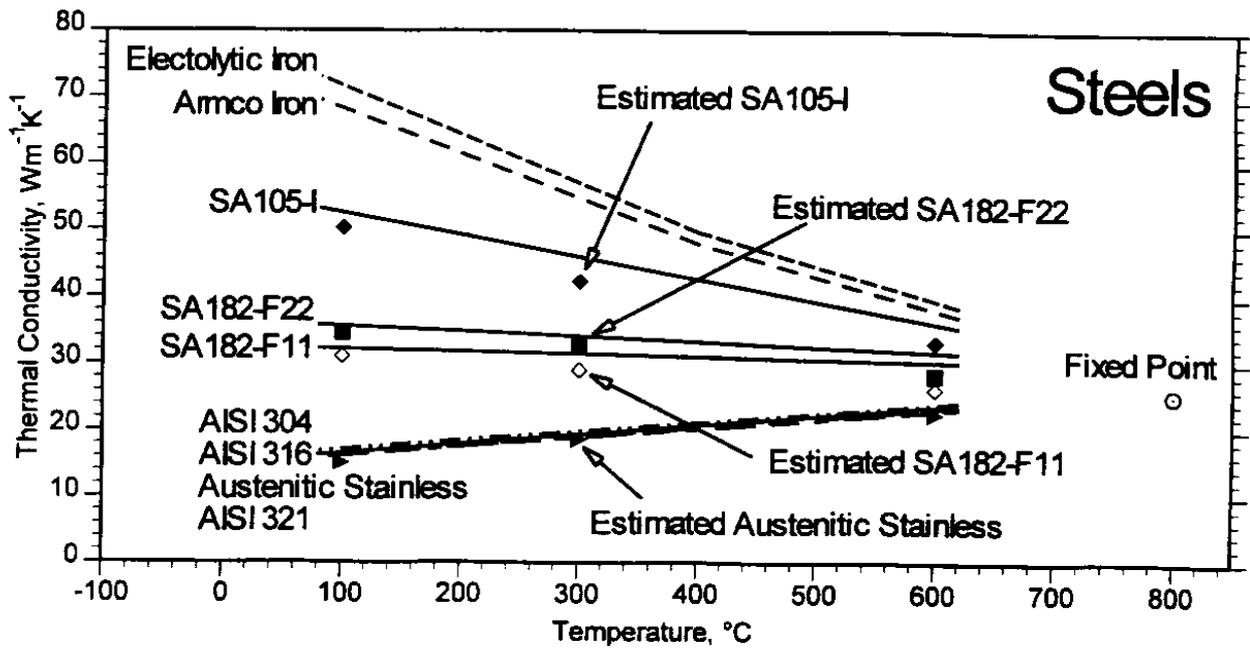
Figure 8 Thermal conductivities of steels as a function of temperature with experimental points superimposed
