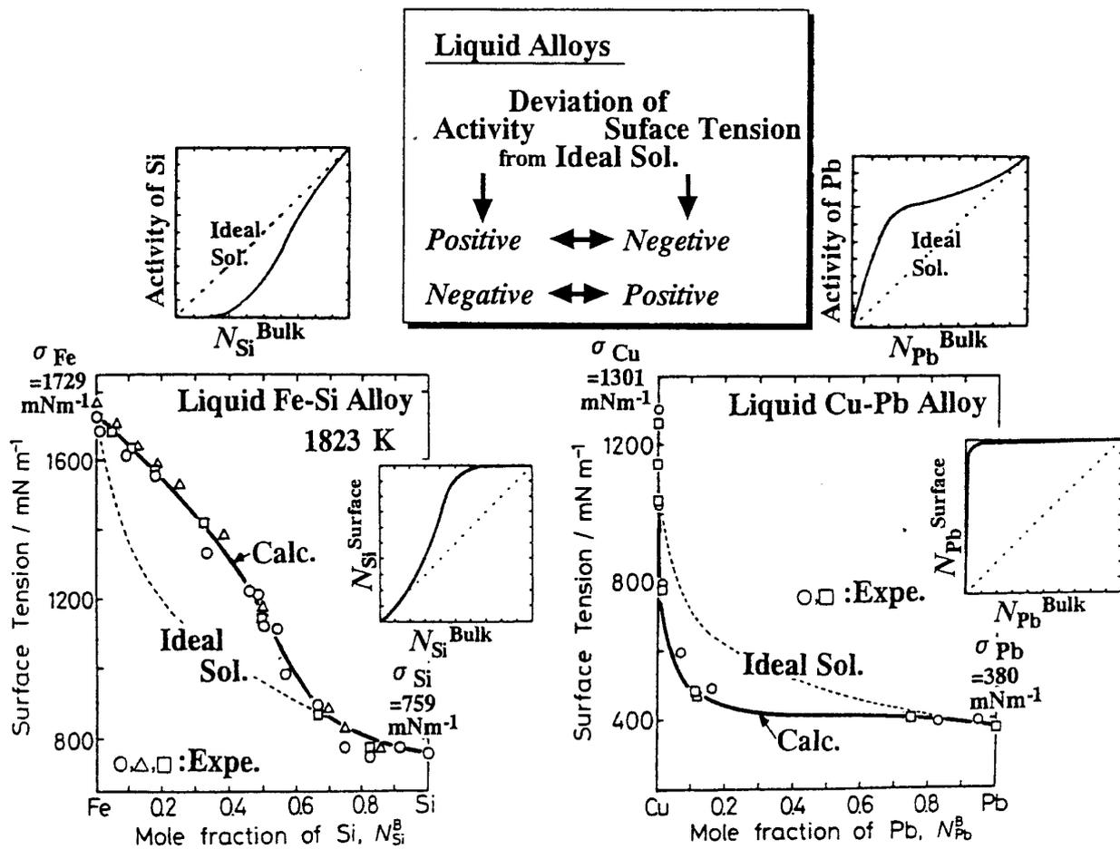
Figure 10 Example of agreement between calculated and experimental values of surface tension for Fe-Si alloys and Cu-Pb alloys.
