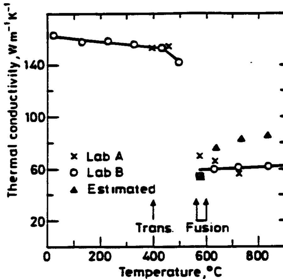
Figure 7 Thermal conductivity of an Al-Si alloy as a function of temperature; solid curve, x, o, measured values; ▲, estimated by Equations 26, 27, ■ estimated by Equation 28.
