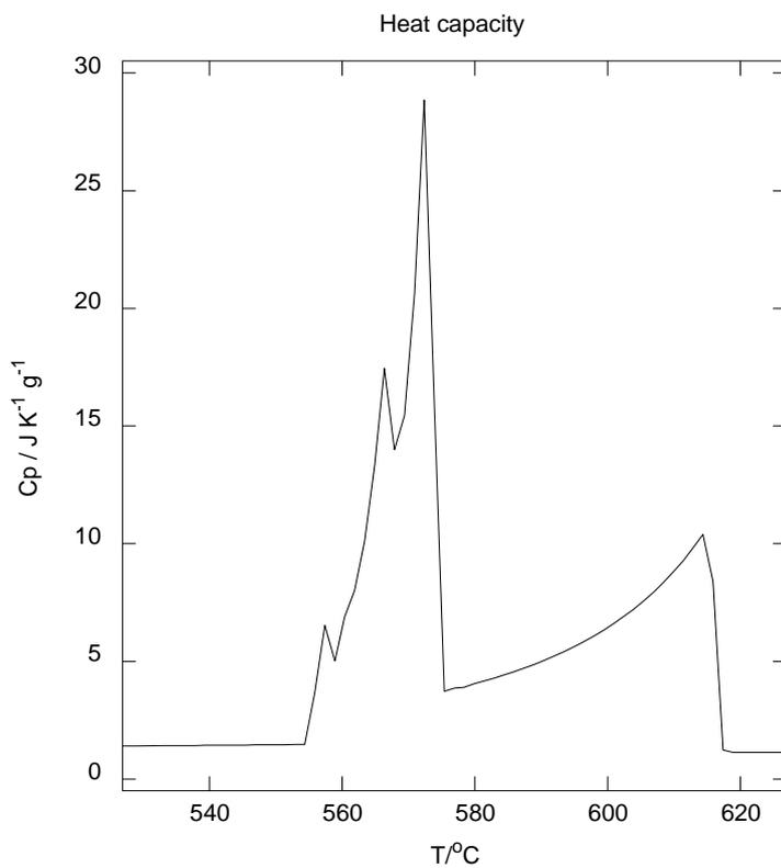
Figure 3 Calculated heat capacity during the fusion of a multicomponent alloy
