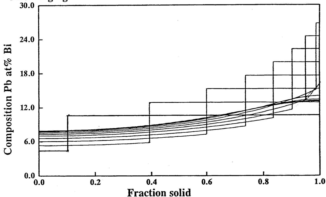
Fig A4 Example run of composition in the solid and liquid in the BiPb system.
