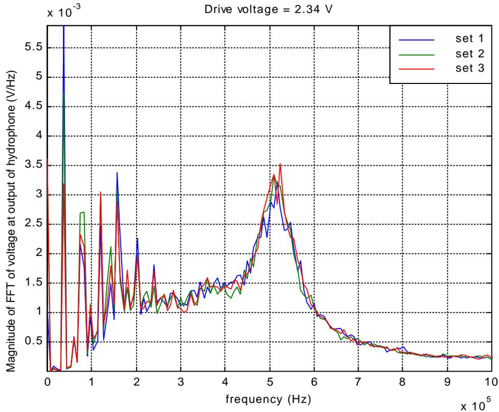
**Figure 5.20:** Hydrophone spectra at centre of tank for 3 sets of measurements, 2.34 V drive voltage
