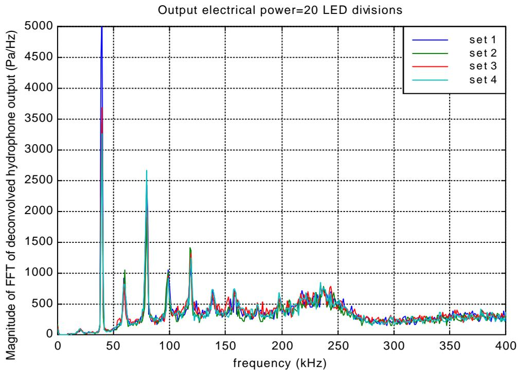
**Figure 5.9:** Spectra adjusted for hydrophone response at centre of tank for 4 sets of measurements; 100% of maximum output electrical power from generator
