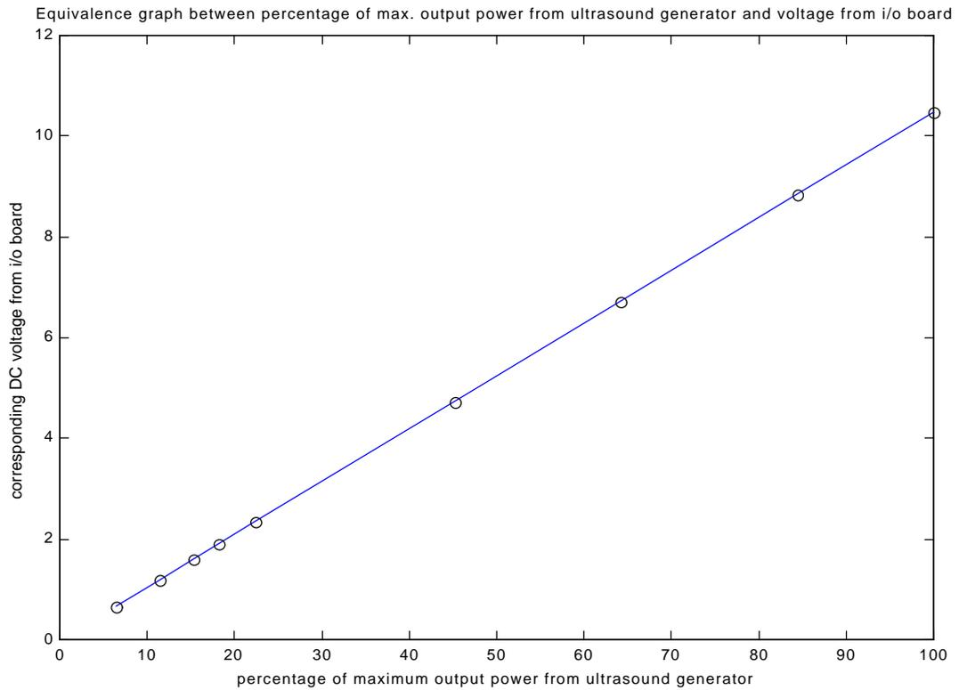
**Figure 5.19:** Equivalence graph between percentage of maximum output electrical power from the ultrasound generator and the DC voltage at the I/O board
