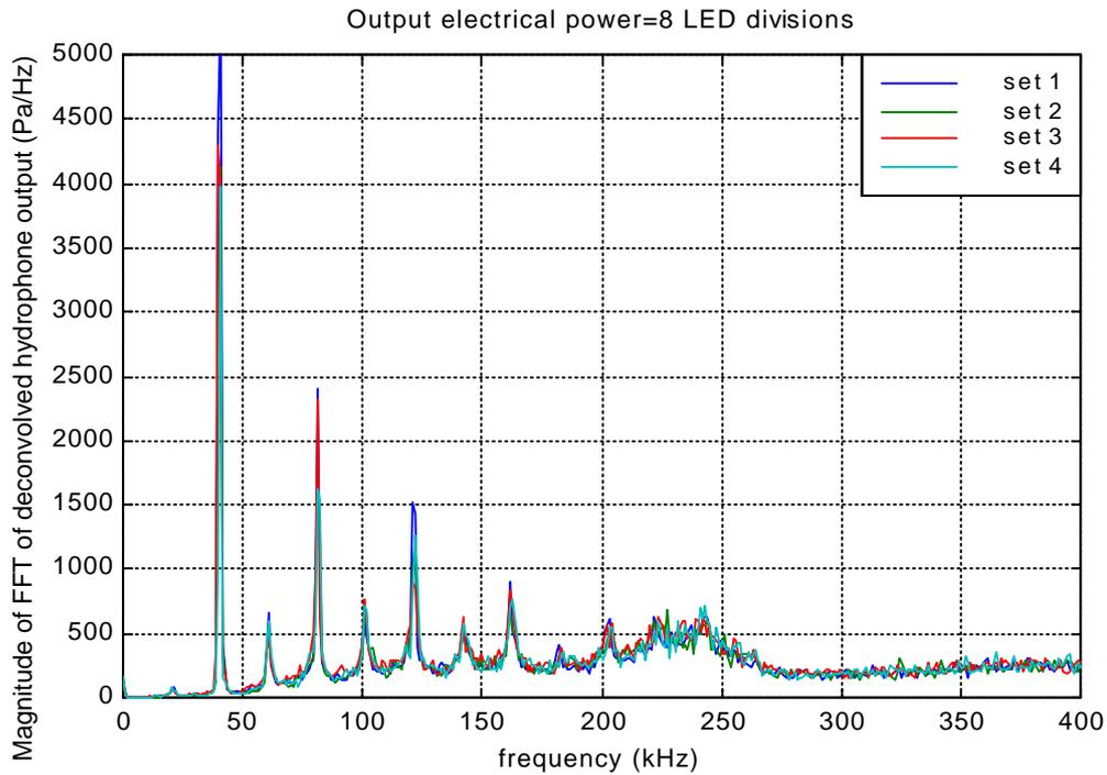
**Figure 5.7:** Spectra adjusted for hydrophone response at centre of tank for 4 sets of measurements; 40% of maximum output electrical power from generator
