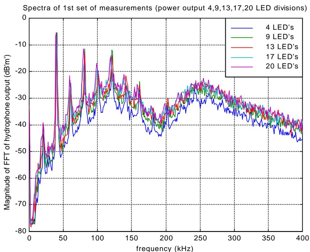
**Figure 5.5:** Hydrophone spectra at centre of tank for first set of measurements. 20%, 45%, 65%, 85% and 100% of maximum output electrical power from generator
