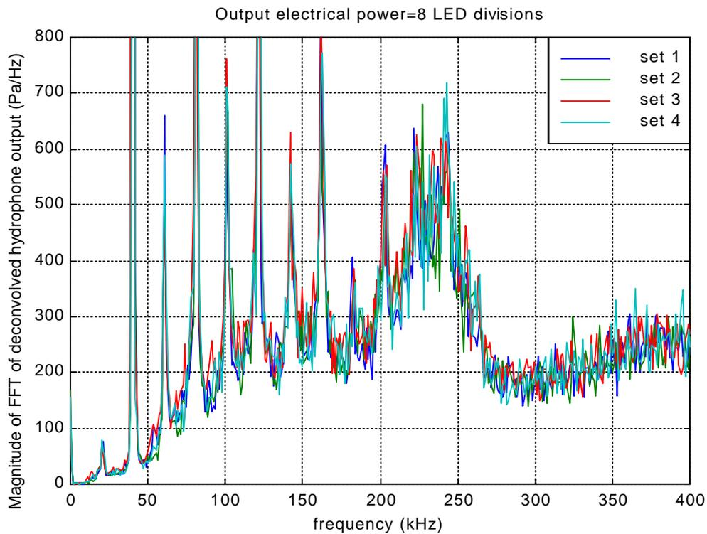
**Figure 5.14:** Spectra adjusted for hydrophone response at centre of tank for 4 sets of measurements in degassed water; 40% of maximum output electrical power from generator
