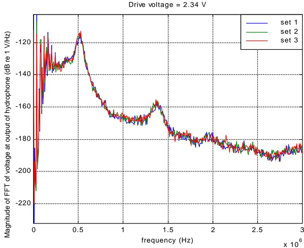
**Figure 5.22:** Hydrophone spectra at centre of tank for 3 sets of measurements plotted on a dB scale, 2.34 V drive voltage
