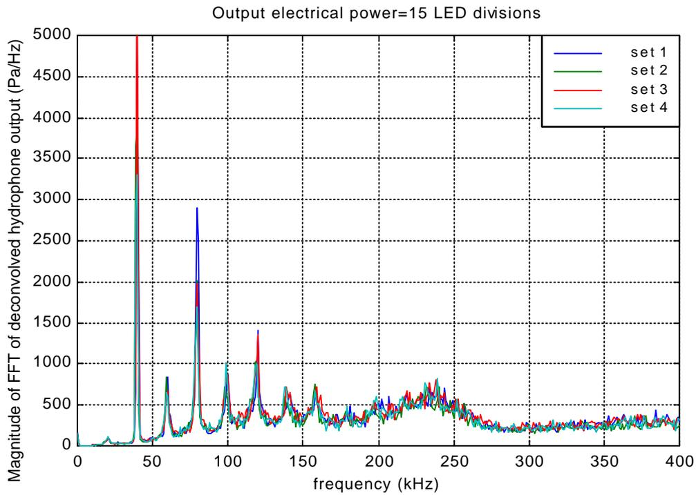
**Figure 5.8:** Spectra adjusted for hydrophone response at centre of tank for 4 sets of measurements; 75% of maximum output electrical power from generator
