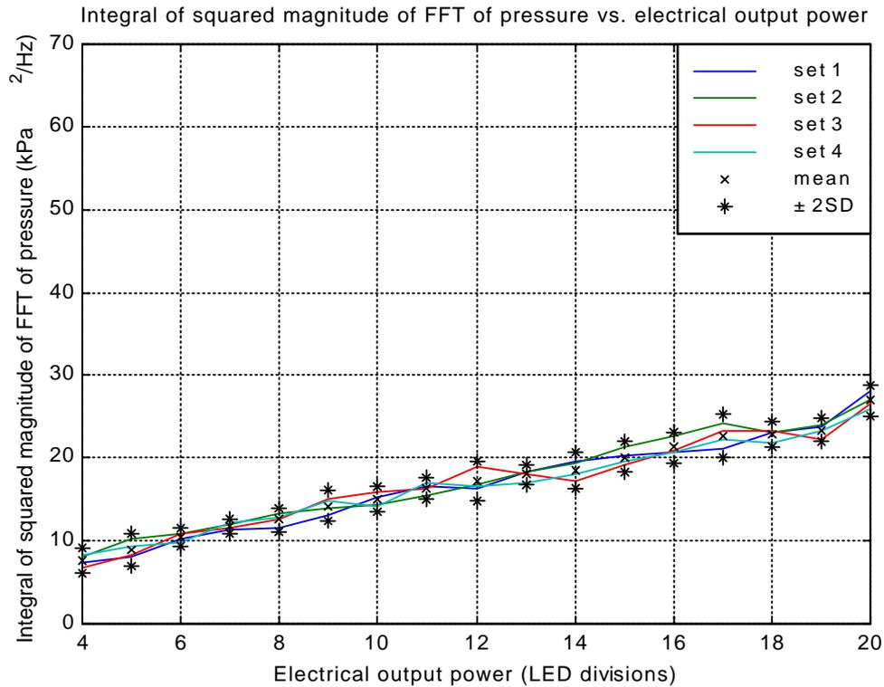
**Figure 5.16:** Energy contained in envelope of spectra: SD denotes the standard deviation
