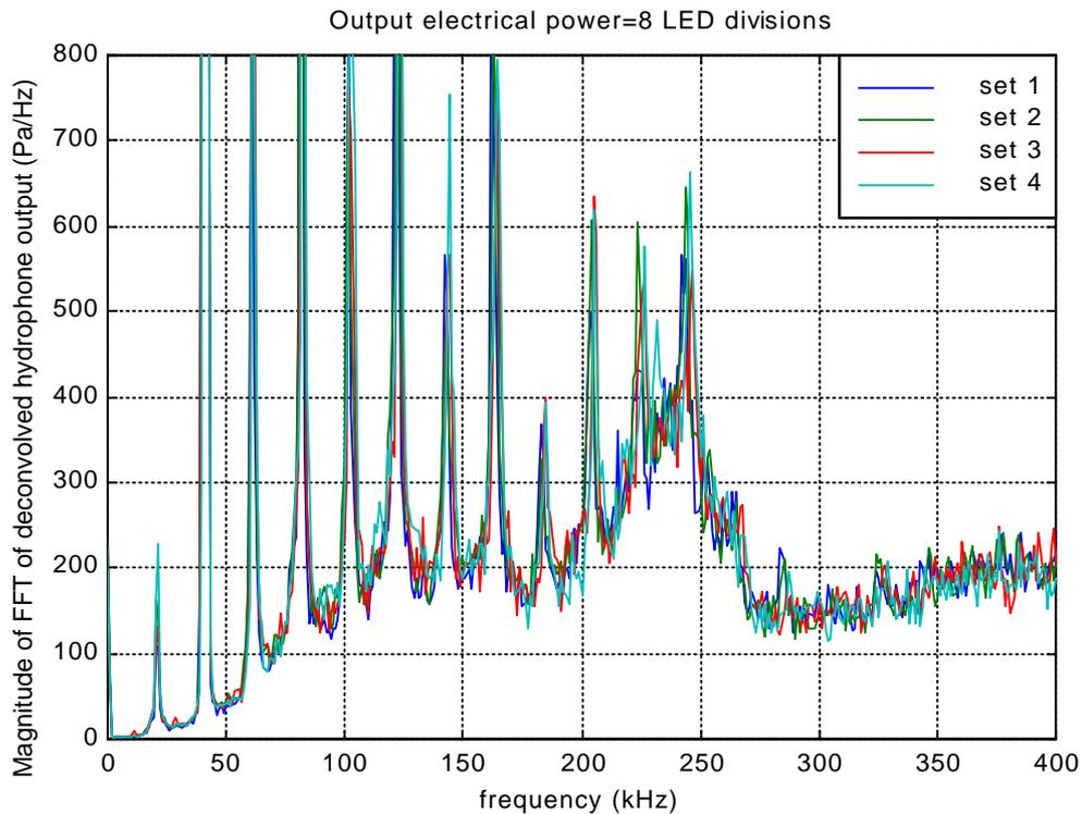
**Figure 5.15:** Spectra adjusted for hydrophone response at centre of tank for 4 sets of measurements in degassed water with surfactant added; 40% of maximum output electrical power from generator
