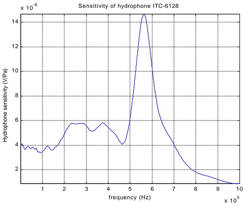
**Figure 5.18:** Hydrophone response obtained from fine-frequency calibration data.
