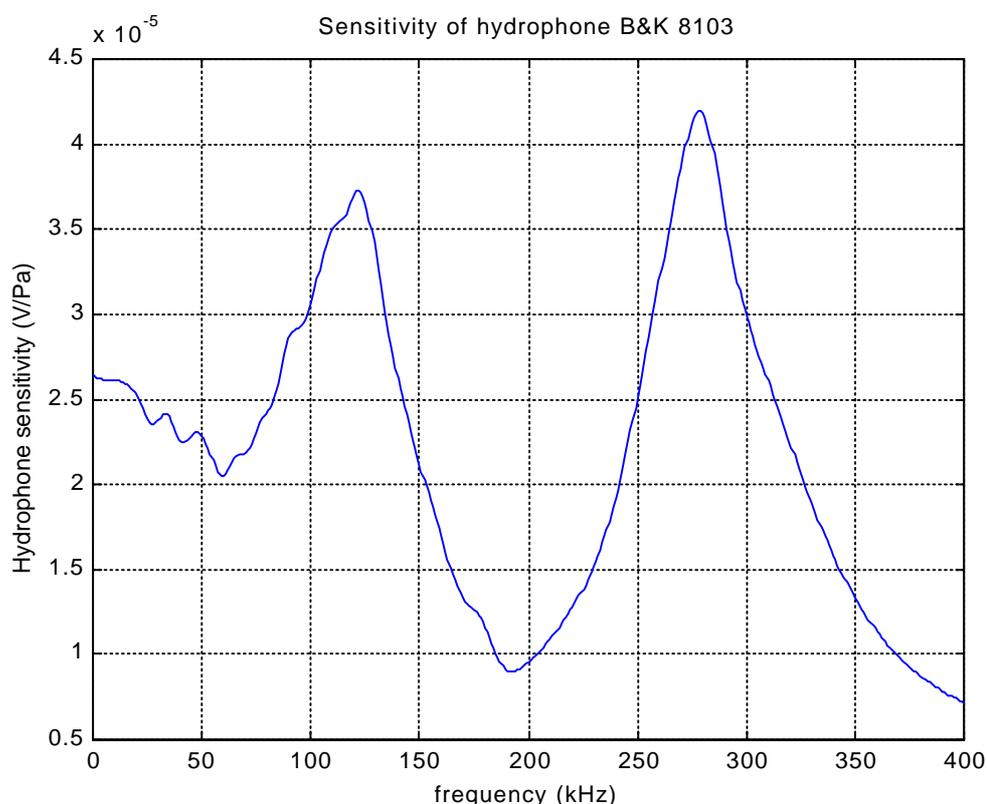
**Figure 5.6:** Hydrophone response obtained from fine-frequency calibration data.
