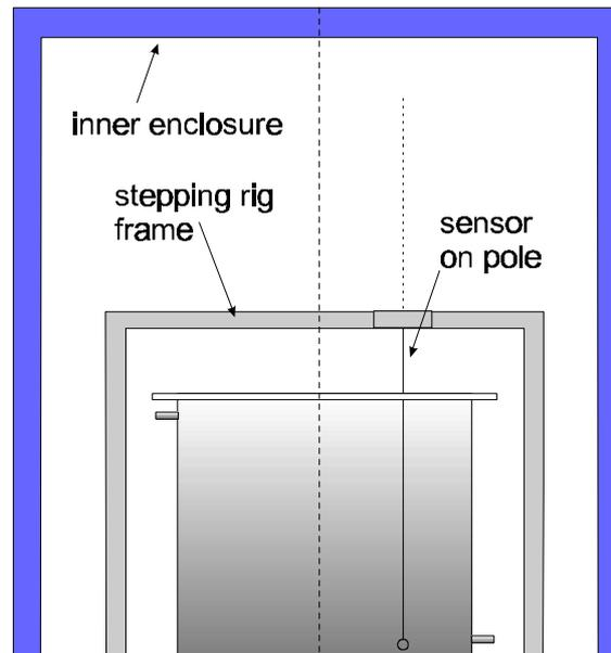
**Figure 3.1:** Schematic representation of bath, scanning rig and enclosure
