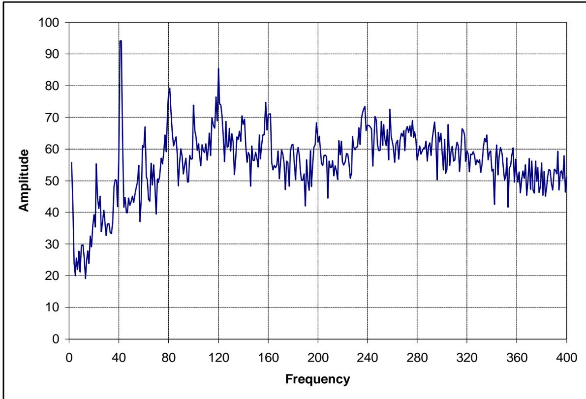
**Figure 5.1:** Typical acoustic spectrum produced by a cavitating bubble field
