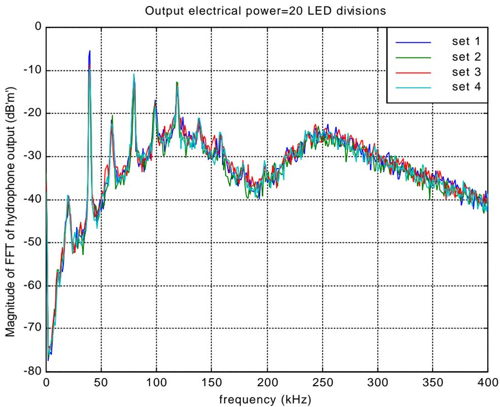
**Figure 5.4:** Hydrophone spectra at centre of tank for 4 sets of measurements. 100% of maximum output electrical power from generator
