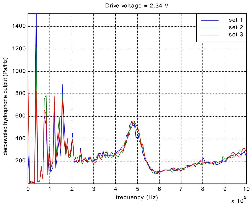
**Figure 5.21:** Spectra adjusted for hydrophone response at centre of tank for 3 sets of measurements, 2.34 V drive voltage
