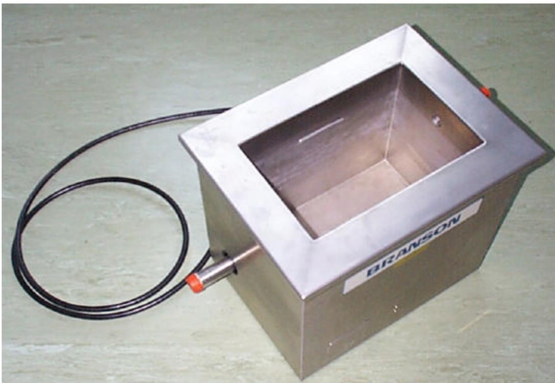
**Figure 3.1:** Branson Ultrasonics cleaning vessel
