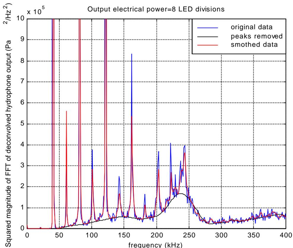
**Figure 5.10:** Squared spectrum, smoothed squared spectrum and estimated envelope. 40% of maximum electrical power output. First set of measurements
