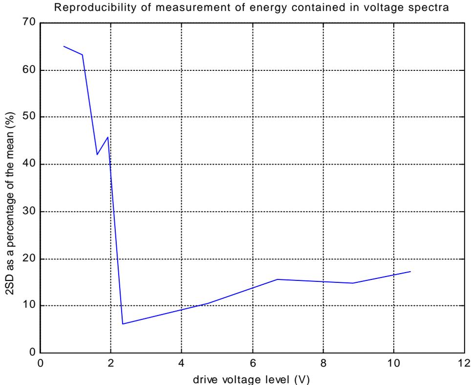
**Figure 5.24:** Reproducibility of measurement of energy contained in voltage spectra between 750 kHz and 3 MHz
