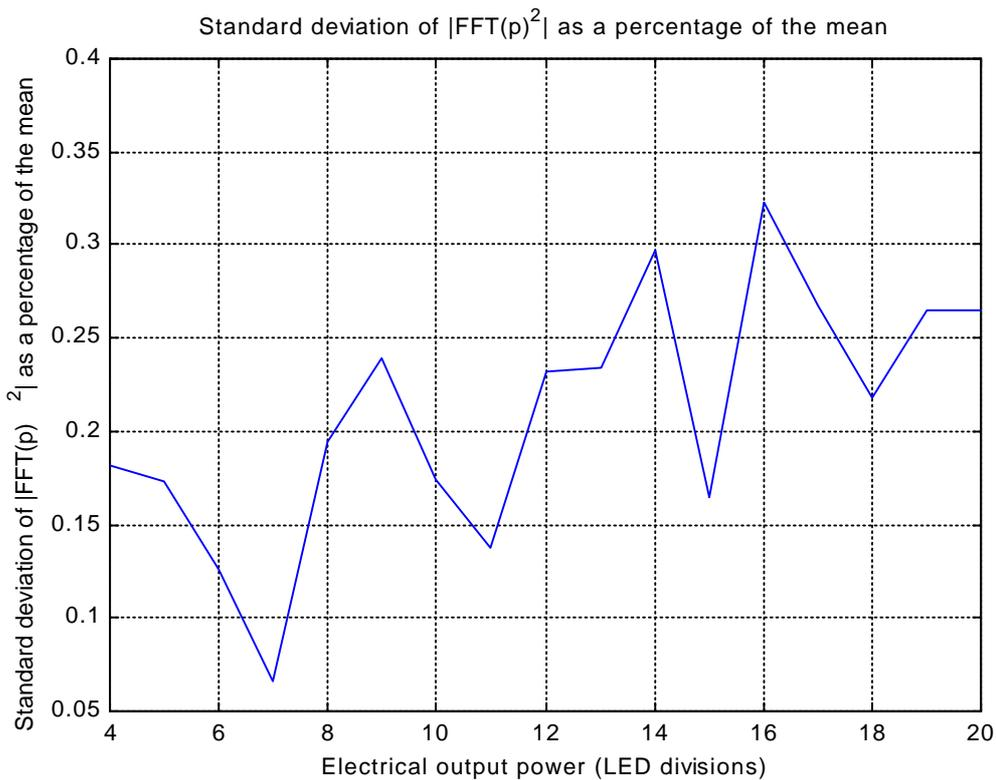
**Figure 5.12:** Reproducibility of measurement of energy contained in pressure spectrum between 0 and 400 kHz
