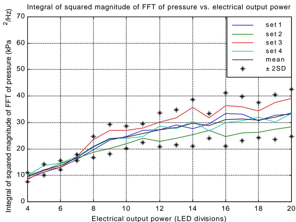
**Figure 5.11:** Energy contained in spectral envelope: SD denotes the standard deviation
