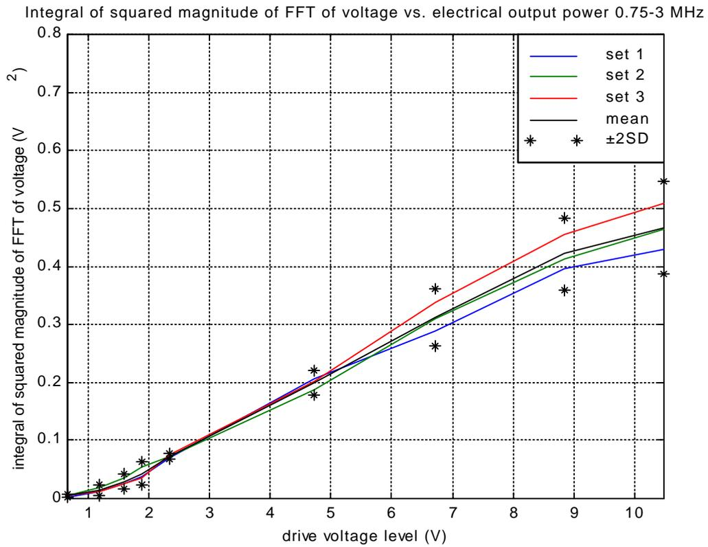
**Figure 5.23:** Energy contained in voltage spectra between 750 kHz and 3 MHz: SD denotes the standard deviation
