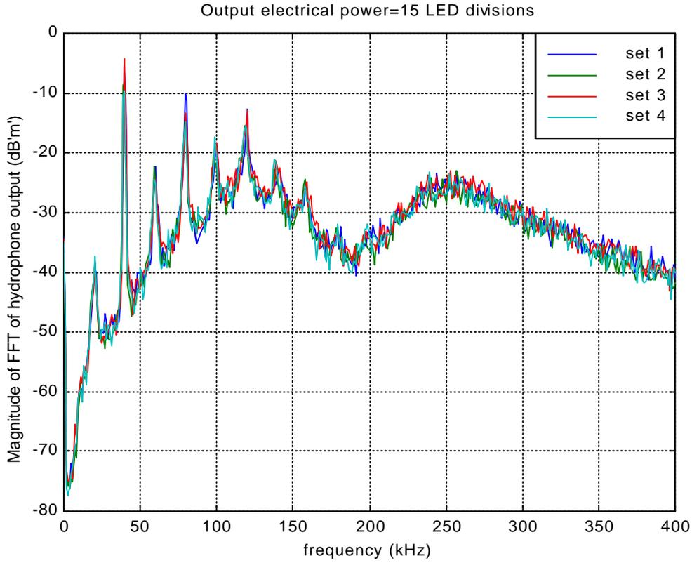
**Figure 5.3:** Hydrophone spectra at centre of tank for 4 sets of measurements. 75% of maximum output electrical power from generator
