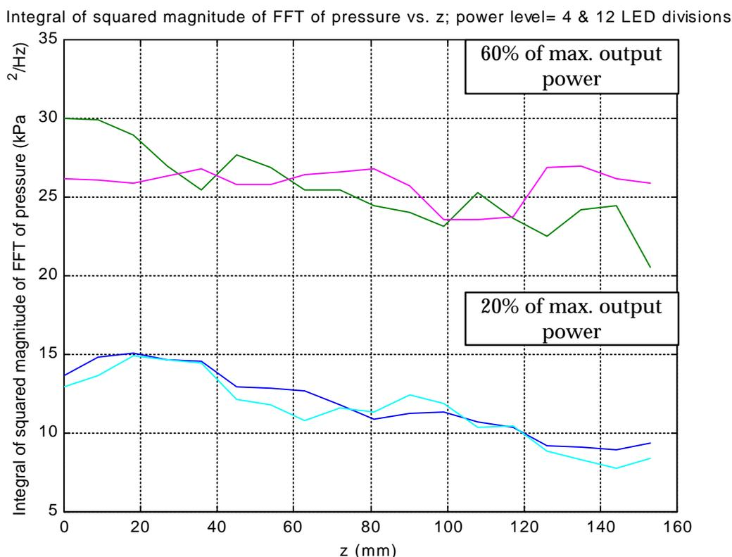
**Figure 5.13:** Energy in spectral envelope as a function of depth, with the cleaning vessel operating at 20% and 60% of maximum output electrical power. Position  $z=0$  corresponds to the centre of the hydrophone active element being level with the water surface
