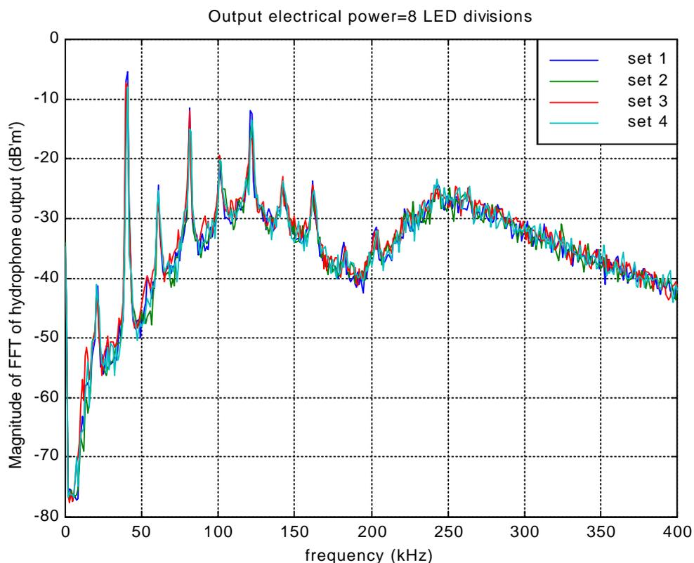
**Figure 5.2:** Hydrophone spectra at centre of tank for 4 sets of measurements. 40% of maximum output electrical power from generator
