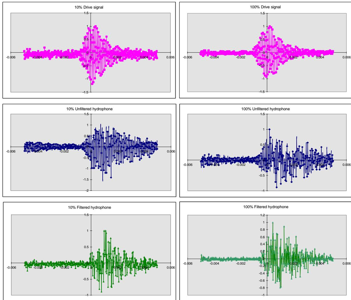
**Figure 5.25:** Three sets of time-domain waveforms, measured using an ITC hydrophone, for power settings of 10% and 100%
