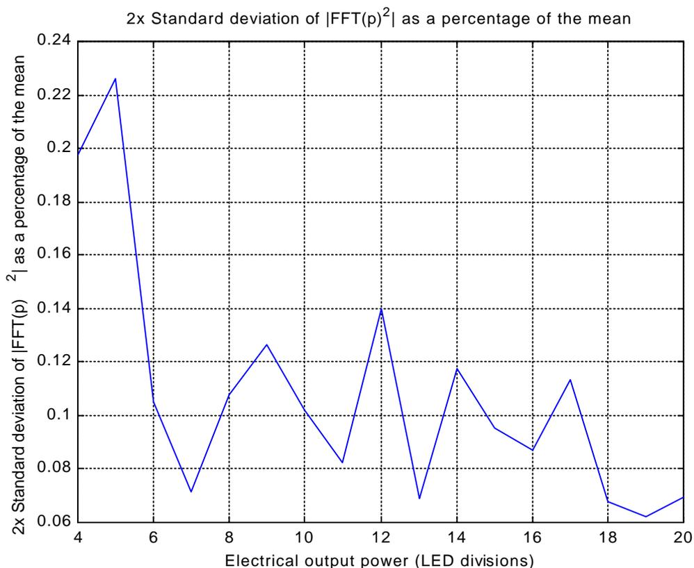
**Figure 5.17:** Reproducibility of measurement of energy contained in pressure spectra between 0 and 400 kHz
