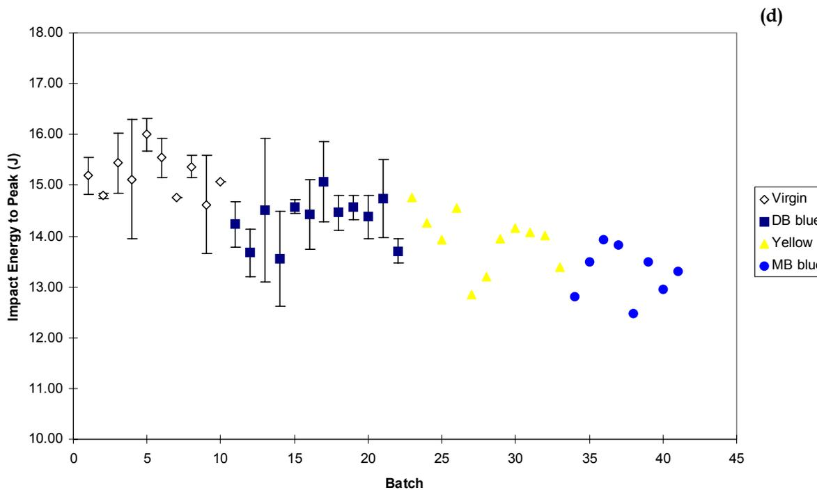
Figure 4 – Average batch results and standard errors for (c) failure strain and (d) peak impact energy (direct blend and masterbatch blue labelled DB and MB blue respectively).
