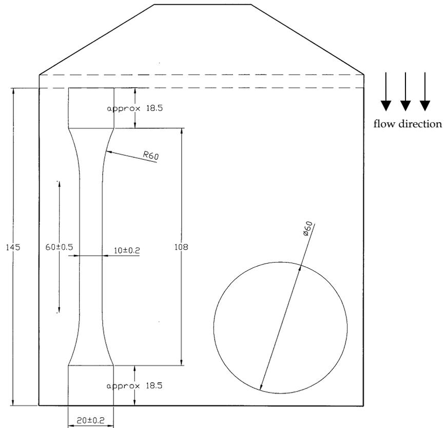
Figure 2 – Schematic diagram of the location and orientation of test-pieces machined from each moulded plate (dimensions marked in mm).
