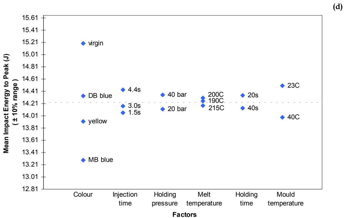
Figure 5 – ANOM result for (c) failure strain and (d) peak impact energy (dashed lines represent the global average).
