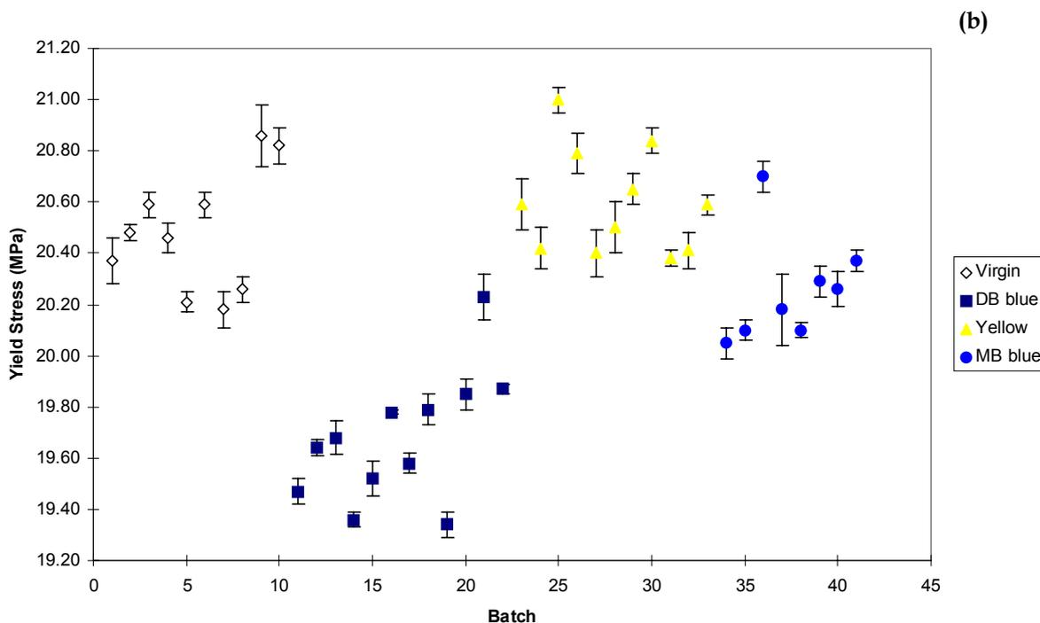
Figure 4 – Average batch results and standard errors for (a) Young’s modulus and (b) maximum yield stress (direct blend and masterbatch blue labelled DB and MB blue respectively).
