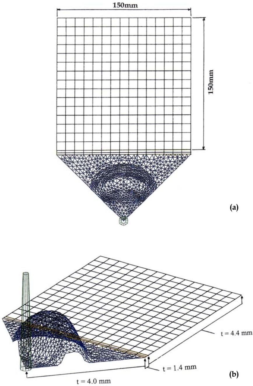
Figure 1 – Design and dimensions of moulding cavity; (a) in-plane and (b) thickness.
