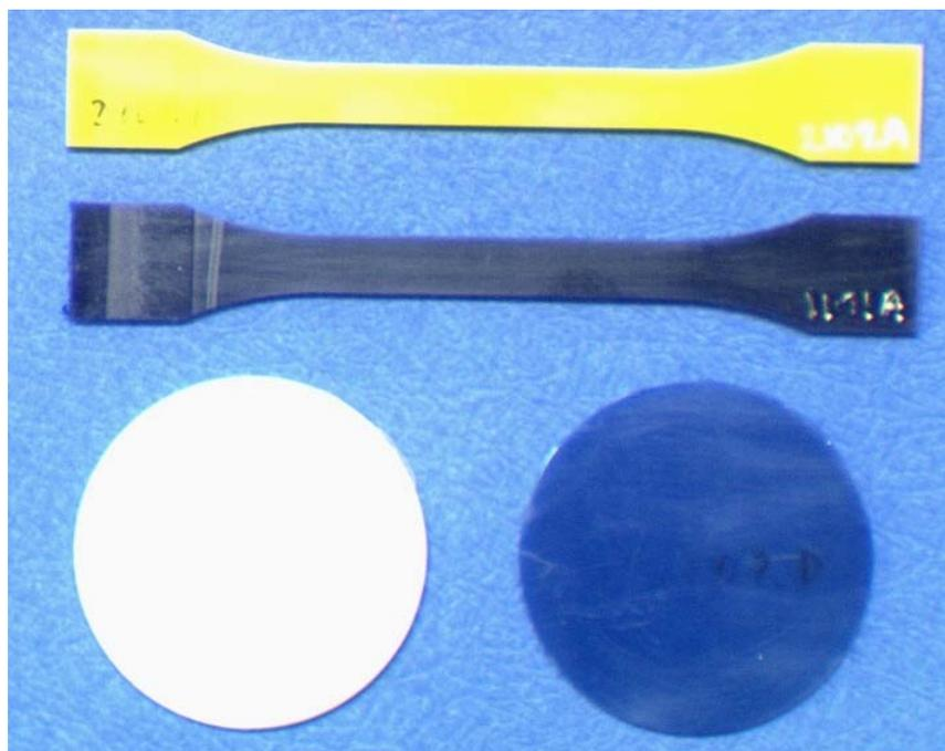
Figure 3 - Typical tensile and impact specimens; from the top: masterbatch yellow, direct blend blue, virgin and masterbatch blue.
