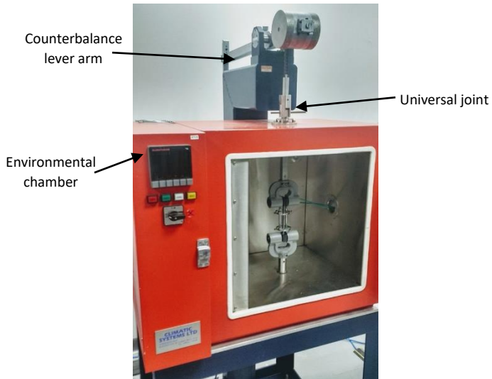
Figure 4 NPL over-slung tensile testing machine for measuring the creep of plastics.
