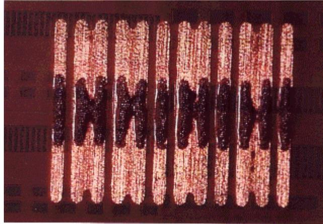
D Aperture showing bridges where pads are connected
