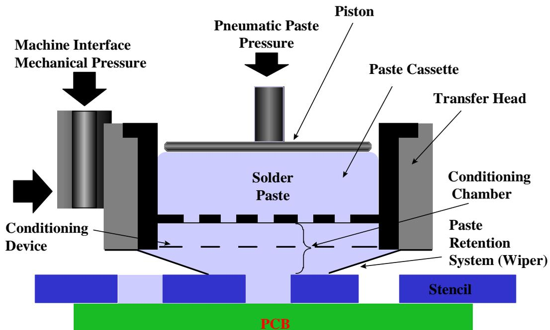
Figure 1 : Schematic of enclosed print head (source : DEK Printing Machines)
