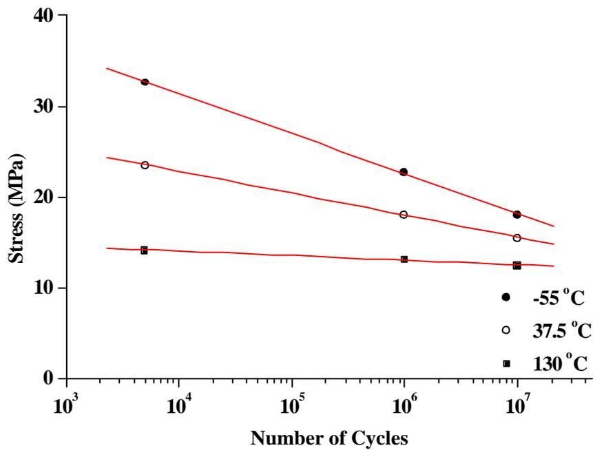
Figure 3 **S-N** data for hot/wet conditioned titanium/FM 350NA joints.
