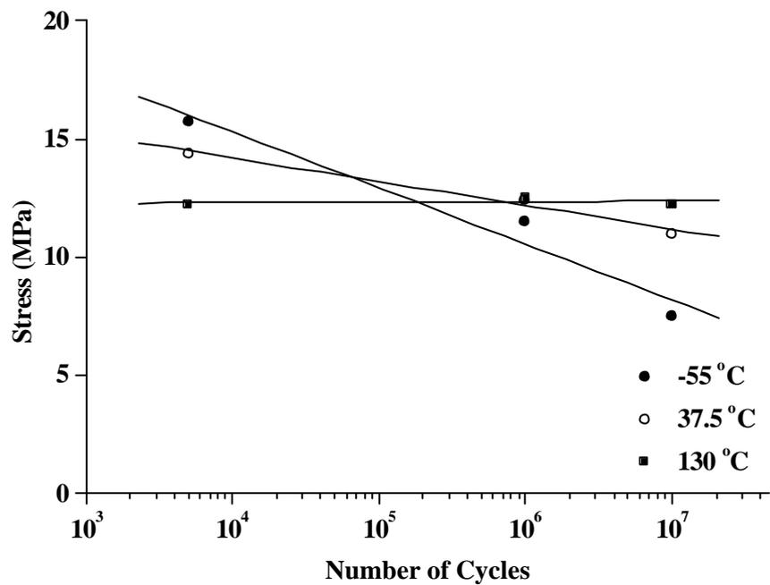
Figure 5 S-N data for hot/wet conditioned titanium/HP655 joints.
