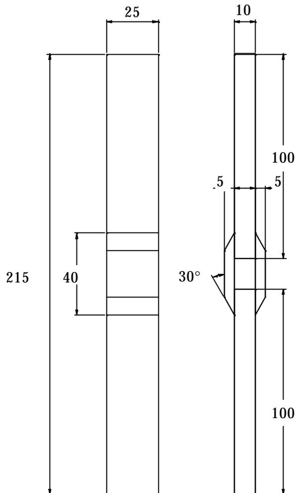
Figure 7 Schematic of tapered-strap joint (dimensions in mm).
