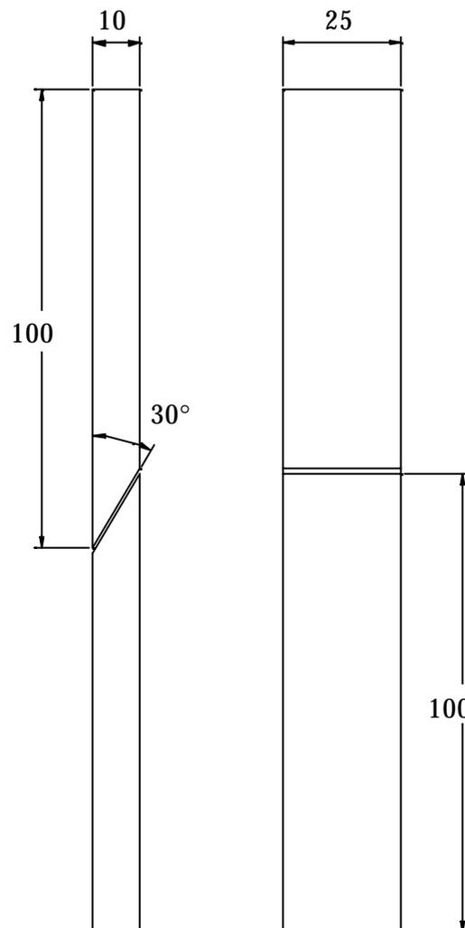
Figure 9 Schematic of scarf joint with taper angle of  $30^\circ$ .
