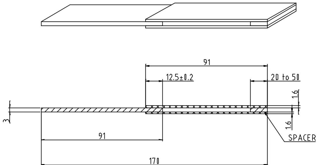
Figure 1 Schematic of fatigue specimen.
