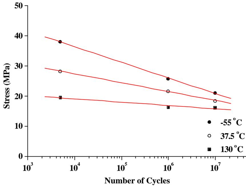
Figure 2 **S-N** data for unconditioned (dry) titanium/FM 350NA joints.
