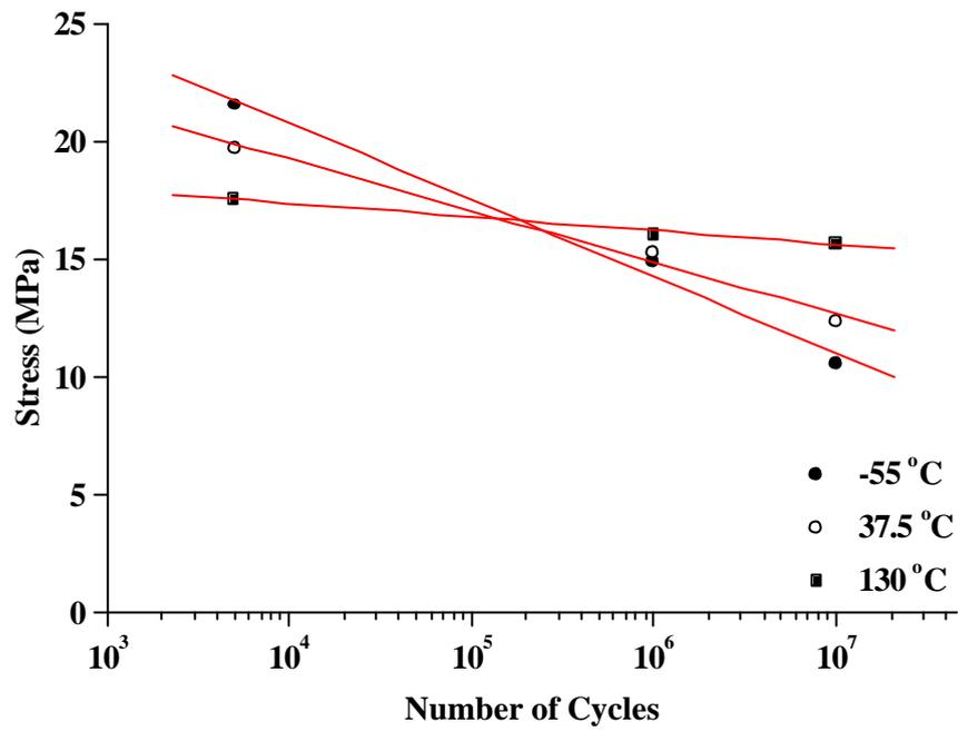
Figure 4 S-N data for unconditioned titanium/HP655 joints.
