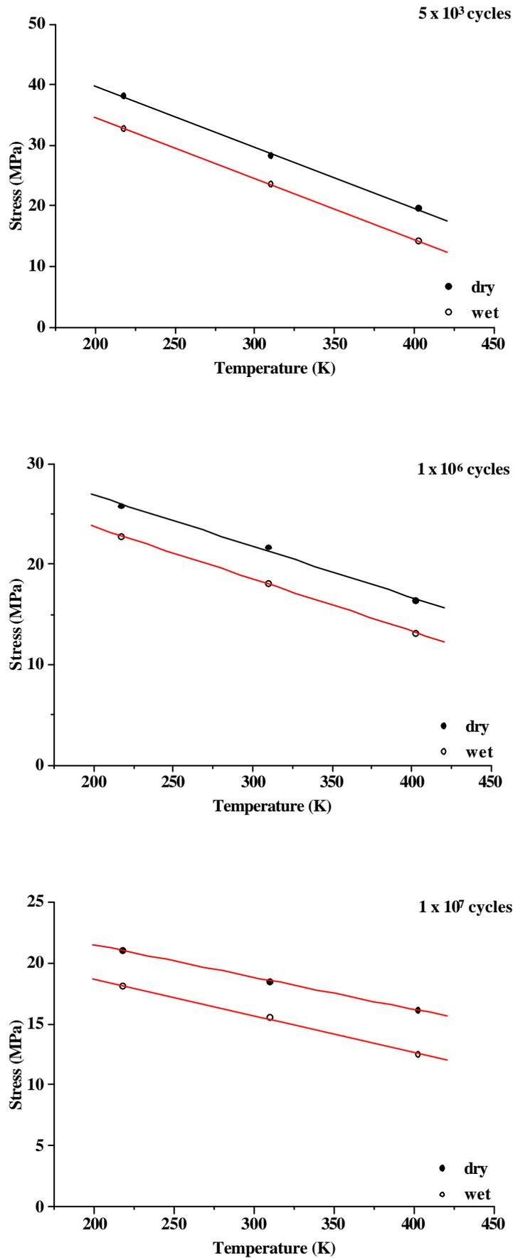
Figure 6 Stress versus temperature for titanium/FM 350NA joints.
