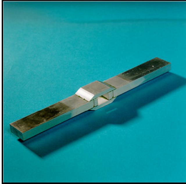
Figure 8 A 5251 aluminium alloy/AF126-2 tapered-strap joint.
