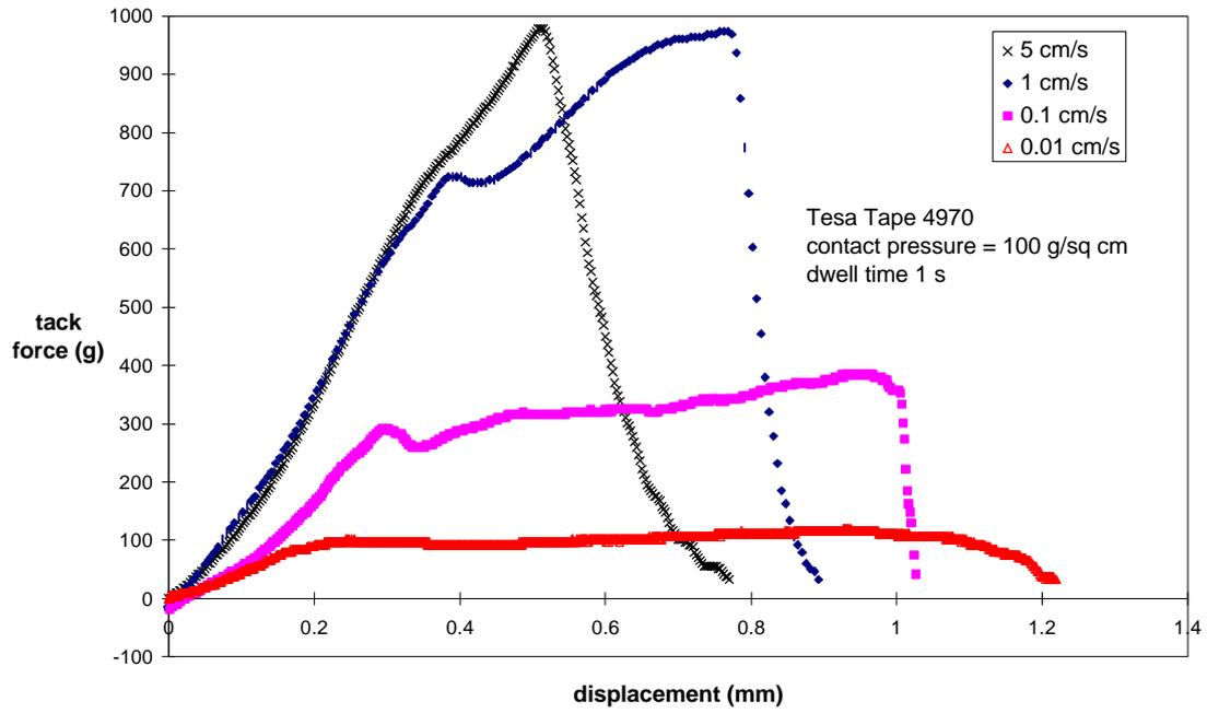
**Figure 11: Tape 4970, Tack Force-Deformation at Different Set Separation Speeds**
