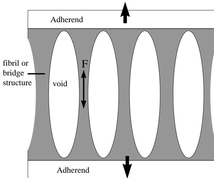
Figure 14: Schematic of Fibril Structures
