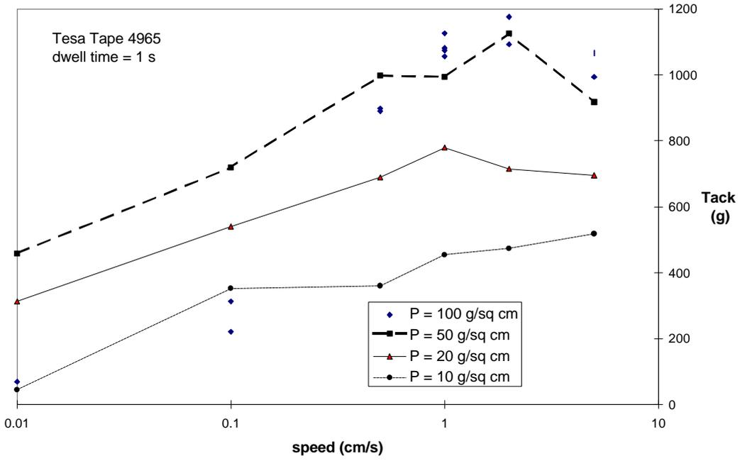
Figure 5: Tape 4965, Tack at Different Contact Pressures (P)
