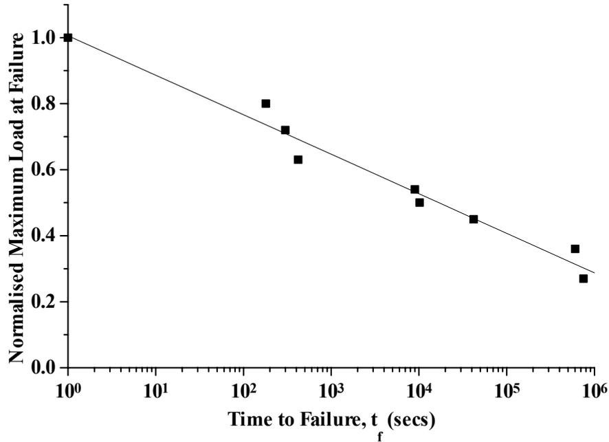
Figure 6 Stress rupture of E-glass fibres in air.
