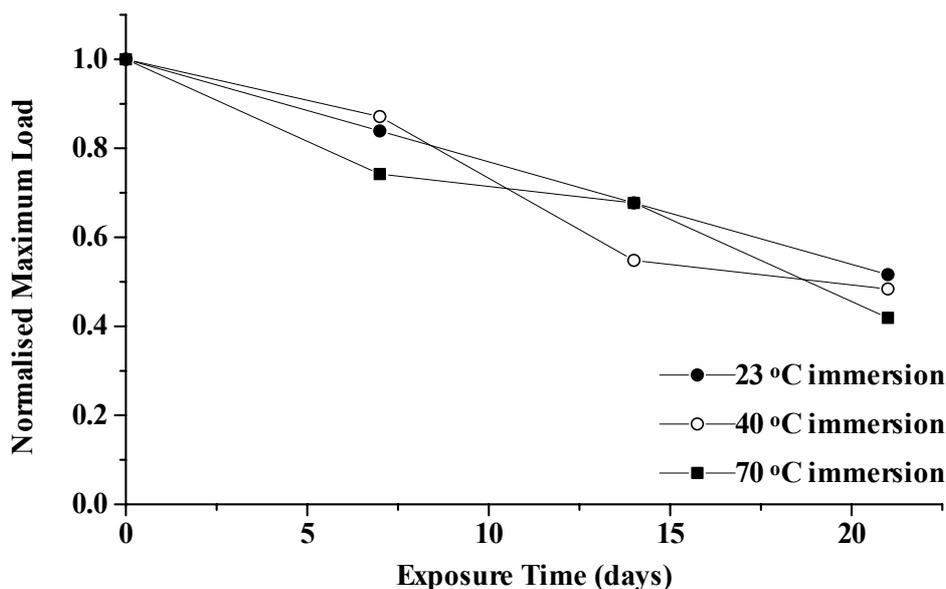
Figure 3 Maximum load at failure for moisture pre-conditioned E-glass fibre tows.
