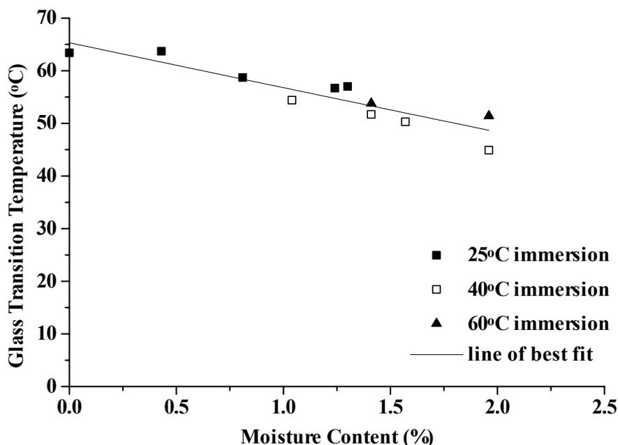
Figure 5 Glass transition temperature for moisture conditioned Crystic 196 polyester.
