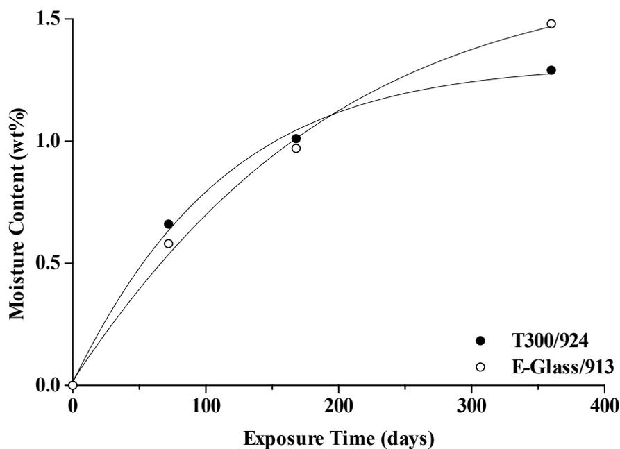
Figure 11 Moisture absorption of longitudinal E-glass/913 and T300/924 specimens.
