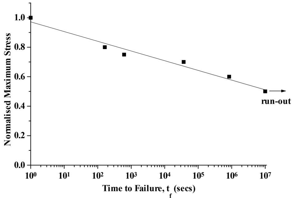
Figure 7 Failure stress of glass/polyester rods in air.
