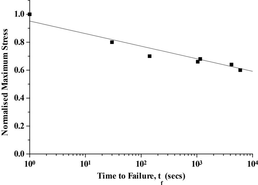
Figure 9 Failure stress of 3 mm wide unidirectional E-glass/F922 laminate in air.
