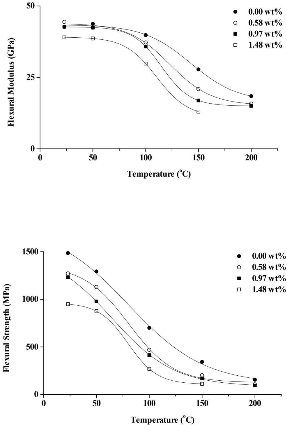
Figure A1 Longitudinal flexural properties of conditioned E-glass/913 with temperature.
