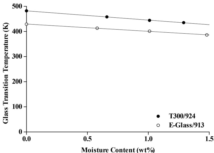
Figure 12 Glass transition temperature for moisture conditioned E-glass/913 and T300/924.
