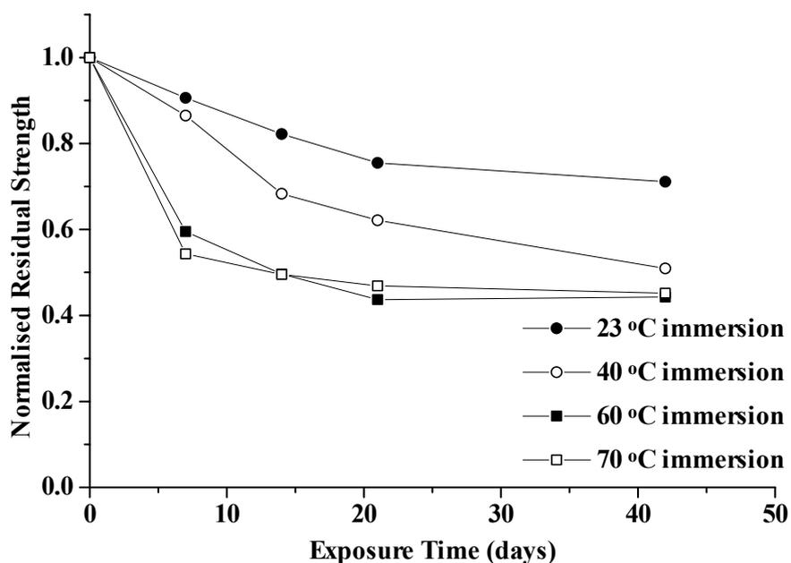
Figure 4 Tensile strength of glass/polyester for different preconditioning temperatures.
