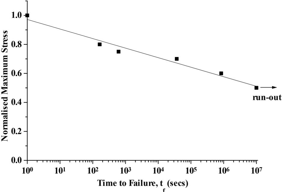
Figure 8 Failure stress of 15 mm wide unidirectional E-glass/F922 laminate in air.
