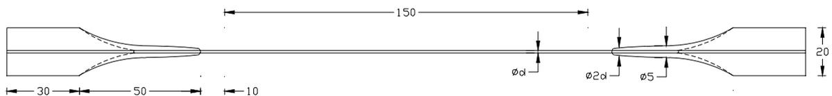
Figure 1 Fibre tow test specimen (mm).
