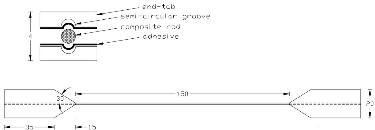
Figure 2 Composite rod specimen and end tab (mm).
