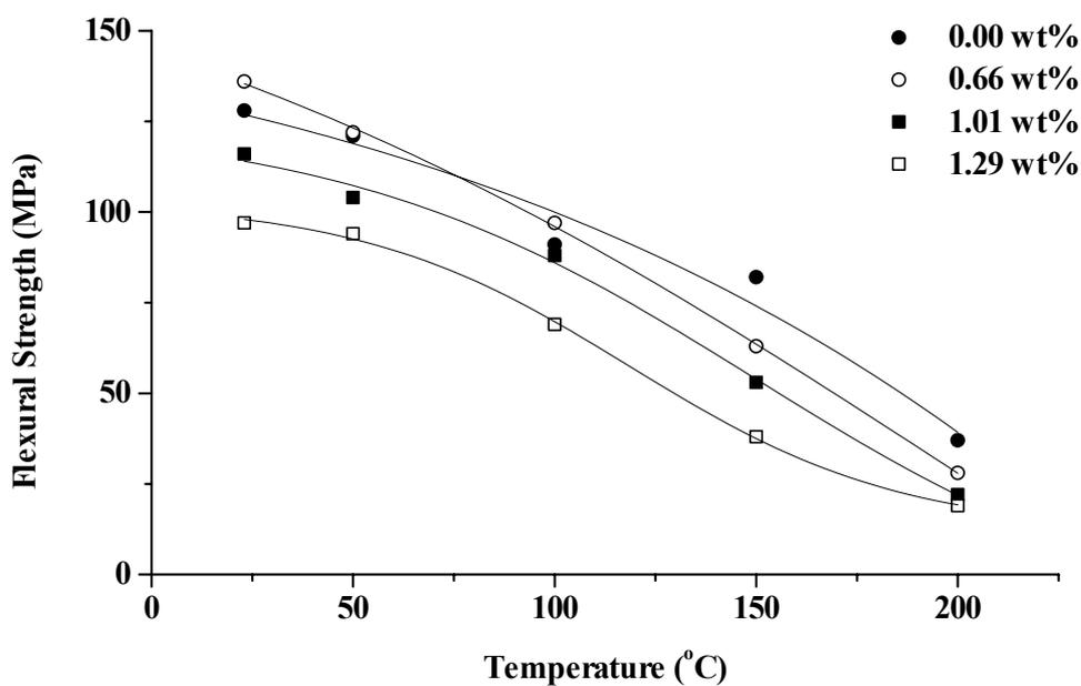
Figure A4 Transverse flexural properties of conditioned T300/924 with temperature.
