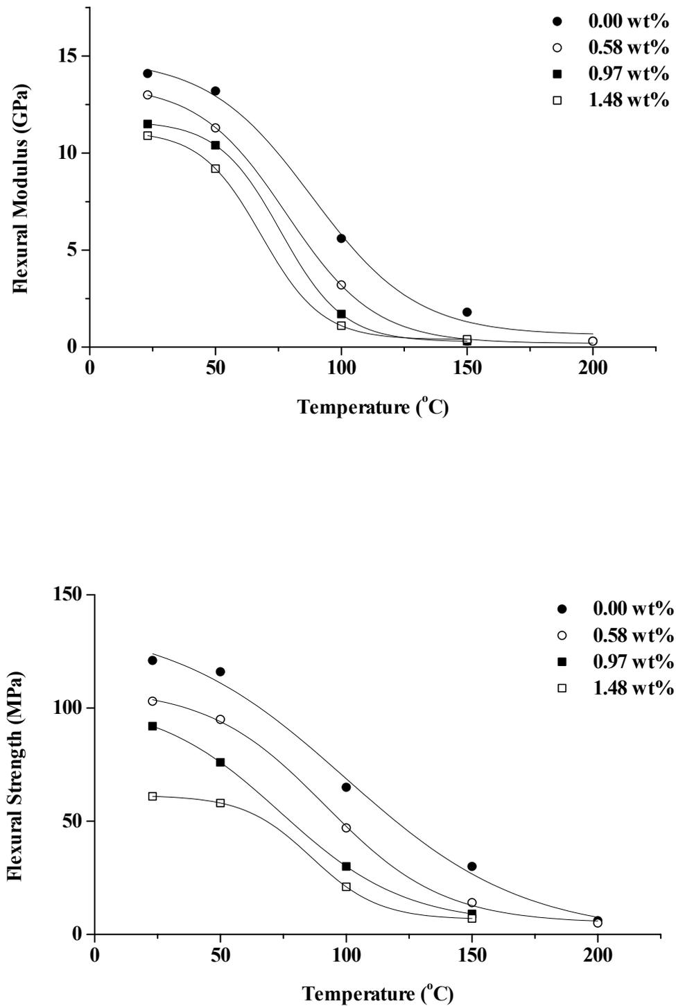
Figure A2 Transverse flexural properties of conditioned E-glass/913 with temperature.
