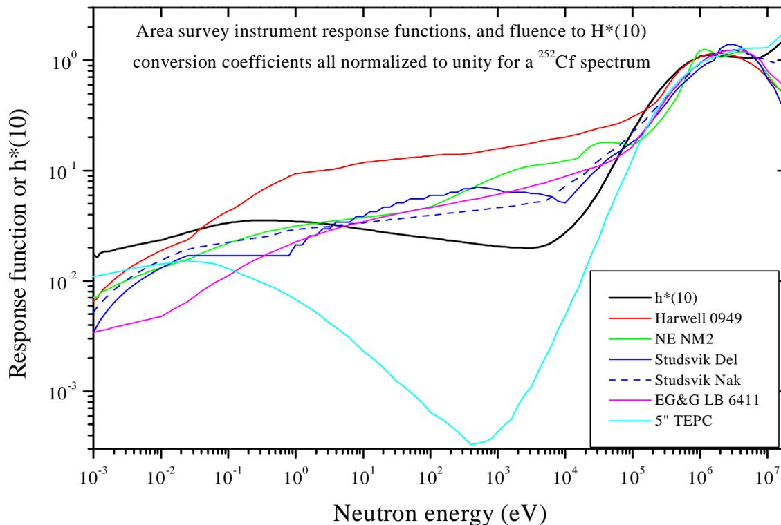
**Figure 10.** Fluence response functions for area survey instruments compared with the fluence to ambient dose equivalent coefficient curve.
