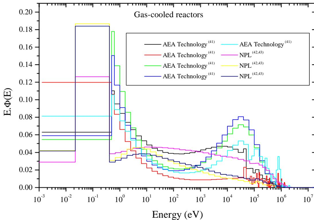
**Figure 15a.** Group of spectra typical of those found in workplaces around gas-cooled reactors in the UK.
