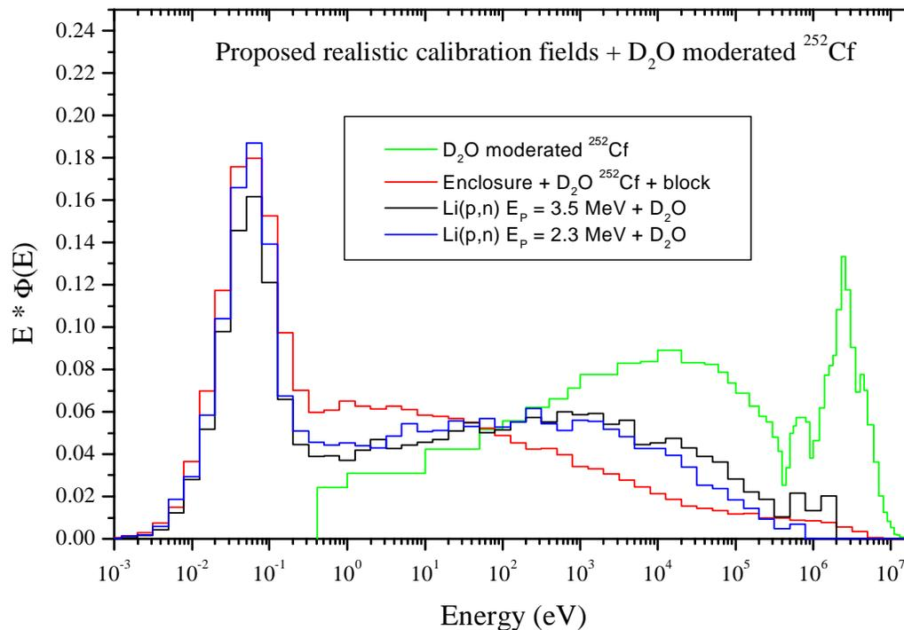
**Figure 8.** Spectra of the three proposed new realistic neutron calibration fields, plus D<sub>2</sub>O moderated <sup>252</sup>Cf spectrum for comparison.
