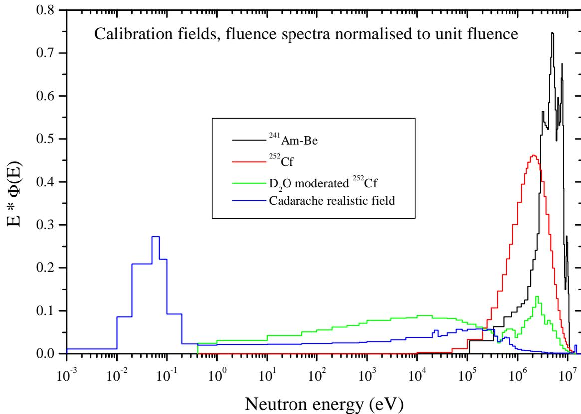
**Figure 3.** Spectra of conventional radionuclide source based calibration fields, plus that of the Cadarache realistic calibration field.
