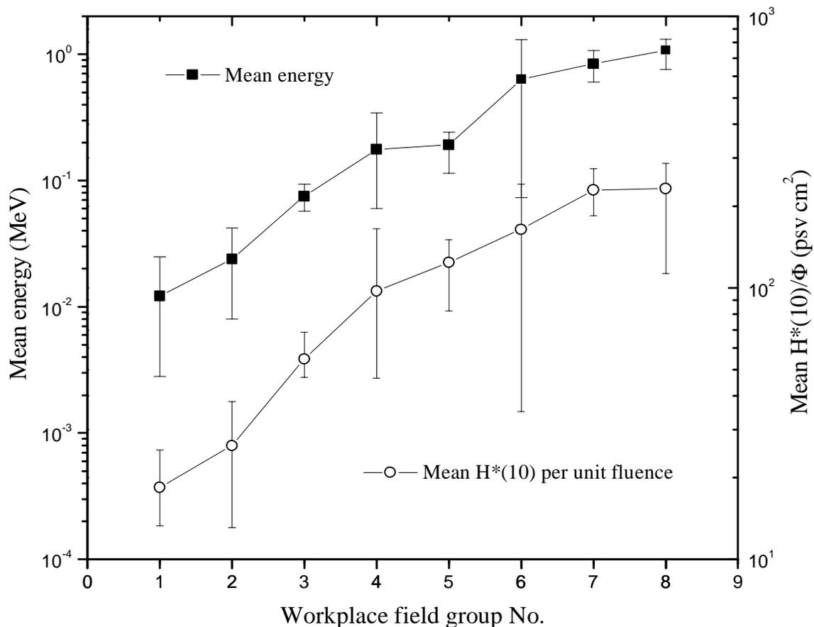
**Figure 2.** The mean energy and the mean  $H^*(10)$  per unit fluence for the workplace field groups. Symbols represent mean values for the group, and the vertical lines through the symbols show the range of values, the top of the line indicating the maximum value and the bottom the minimum.
