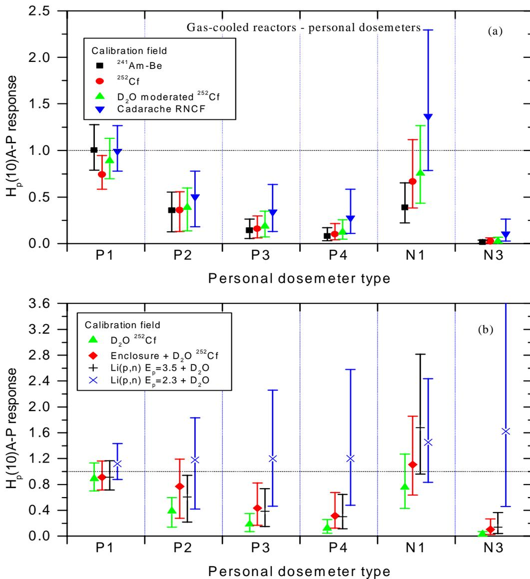
**Figure 15c.** Responses for personal dosimeters P1, P2, P3, P4, N1, and N3 for a group of spectra typical of those found in workplaces around gas-cooled reactors. Symbols represent mean values of the responses for the group, after calibration in one of the seven chosen fields, and the vertical lines through the symbols show the range of response values, the top of the line indicating the maximum value and the bottom the minimum.
