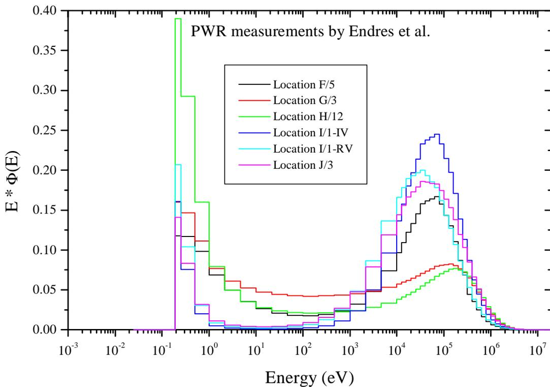
**Figure 17a.** Group of spectra measured by Endres et al.<sup>(46)</sup> at various PWR stations in the US.
