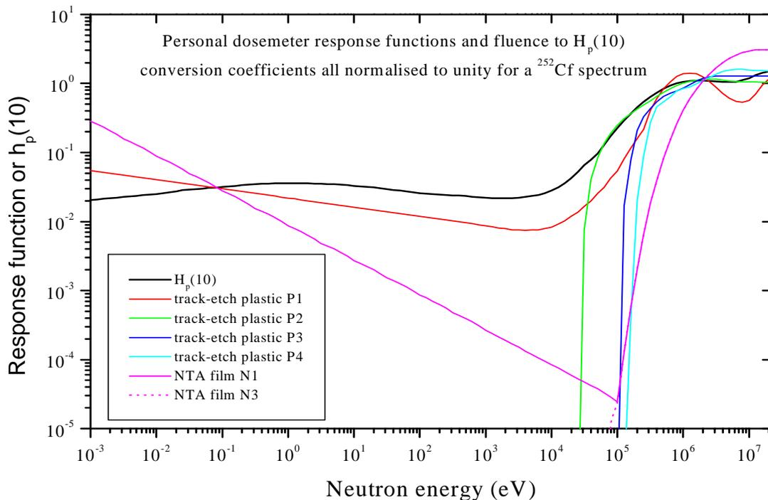
**Figure 11.** Fluence response functions for personal dosimeters compared with the fluence to personal dose equivalent (A-P) conversion coefficient curve.
