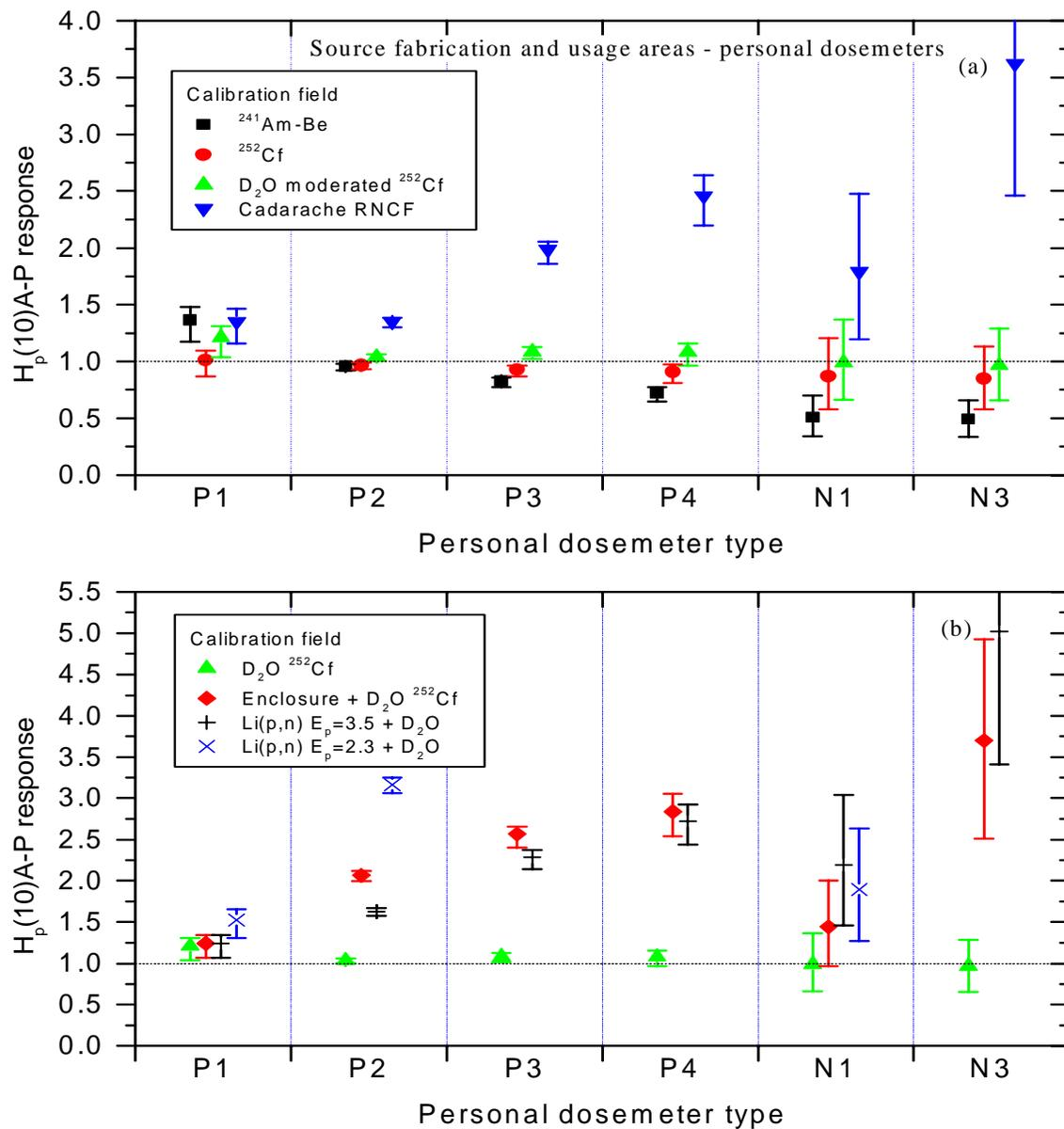
**Figure 21c.** Responses for personal dosimeters P1, P2, P3, P4, N1, and N3 for a group of spectra typical of those found in areas where radionuclide sources are fabricated or where they are used. Symbols represent mean values of the responses for the group, after calibration in one of the seven chosen fields, and the vertical lines through the symbols show the range of response values, the top of the line indicating the maximum value and the bottom the minimum.
