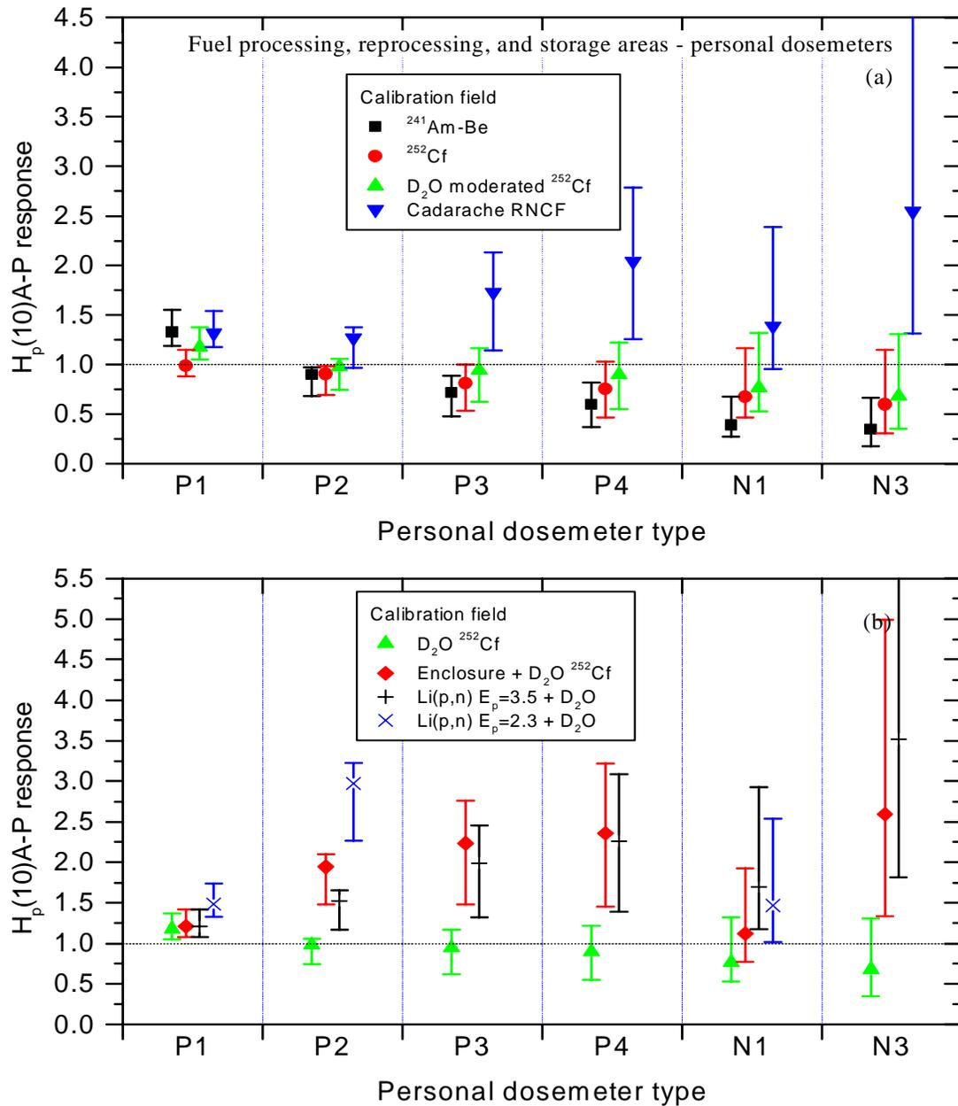
**Figure 19c.** Responses for personal dosemeters P1, P2, P3, P4, N1, and N3 for a group of spectra typical of those found in workplaces around fuel processing, reprocessing, and storage areas. Symbols represent mean values of the responses for the group, after calibration in one of the seven chosen fields, and the vertical lines through the symbols show the range of response values, the top of the line indicating the maximum value and the bottom the minimum.
