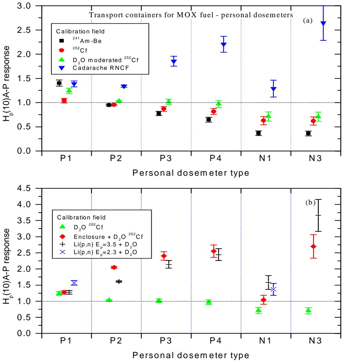
**Figure 20c.** Responses for personal dosimeters P1, P2, P3, P4, N1, and N3 for a group of spectra typical of those found around transport containers for MOX fuel elements. Symbols represent mean values of the responses for the group, after calibration in one of the seven chosen fields, and the vertical lines through the symbols show the range of response values, the top of the line indicating the maximum value and the bottom the minimum
