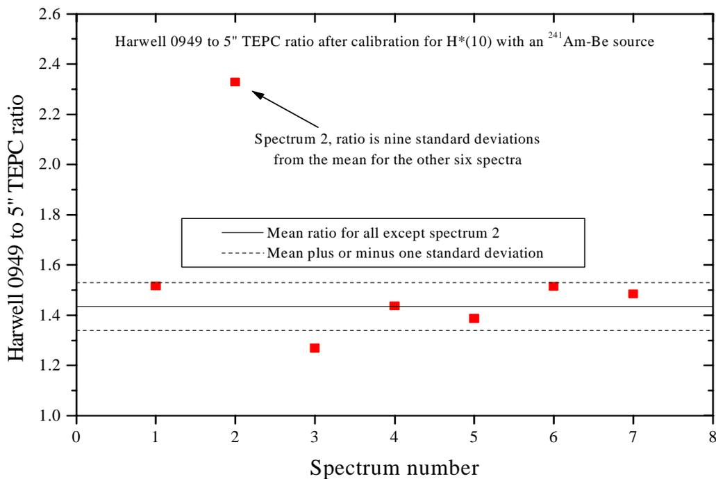
**Figure 22.** Ratio of Harwell 0949 response to a 5" TEPC response for the spectra of group 6, all measured in fuel processing, reprocessing, or storage areas.
