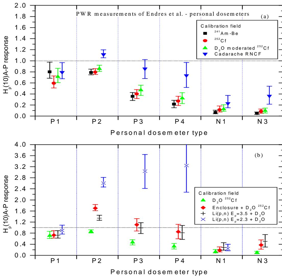
**Figure 17c.** Responses for personal dosemeters P1, P2, P3, P4, N1, and N3 for a group of spectra measured inside containment of PWRs by Endres et al. Symbols represent mean values of the responses for the group, after calibration in one of the seven chosen fields, and the vertical lines through the symbols show the range of response values, the top of the line indicating the maximum value and the bottom the minimum.
