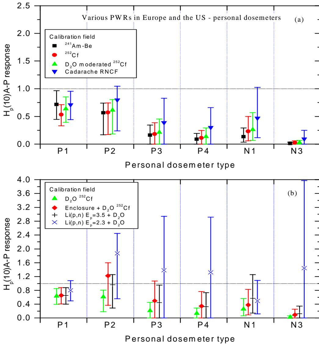
**Figure 16c.** Responses for personal dosimeters P1, P2, P3, P4, N1, and N3 for a group of spectra typical of those found in workplaces around various PWR stations. Symbols represent mean values of the responses for the group, after calibration in one of the seven chosen fields, and the vertical lines through the symbols show the range of response values, the top of the line indicating the maximum value and the bottom the minimum.
