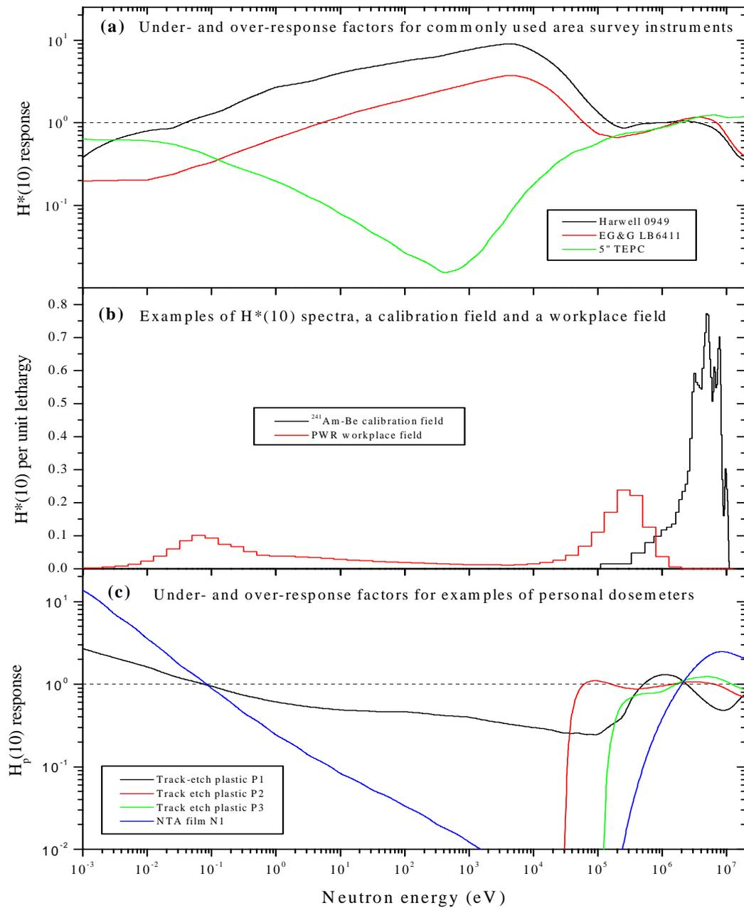
**Figure 1.** Examples of typical under- and over-response factors for area survey instruments (a) and personal dosimeters (c), compared with the ambient dose equivalent spectral distributions for a typical calibration field and a soft workplace field (b).
