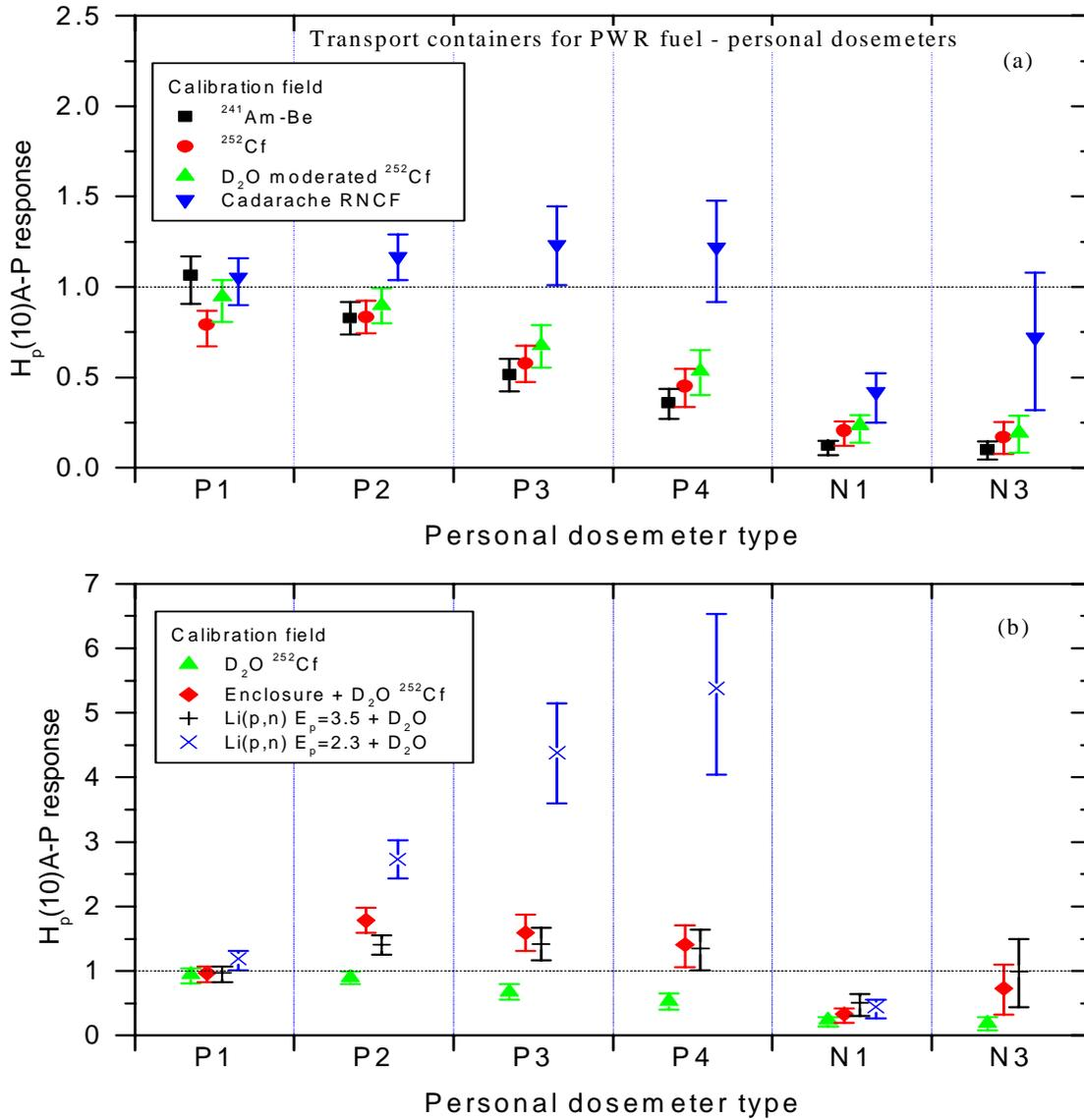
**Figure 18c.** Responses for personal dosimeters P1, P2, P3, P4, N1, and N3 for a group of spectra typical of those found around transport containers for PWR fuel. Symbols represent mean values of the responses for the group, after calibration in one of the seven chosen fields, and the vertical lines through the symbols show the range of response values, the top of the line indicating the maximum value and the bottom the minimum.
