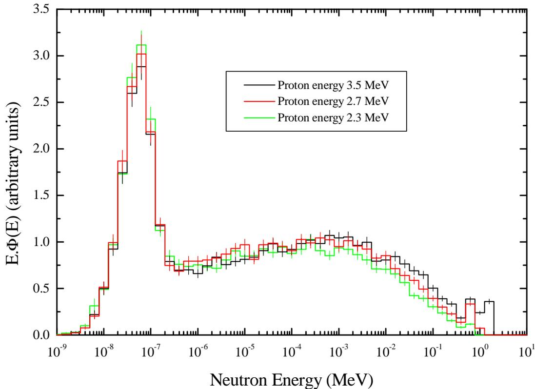
**Figure 7.** Comparison between spectra produced by varying the incident proton energy for the  ${}^7\text{Li}(p,n)$  reaction moderated by a 40 cm diameter sphere of  $\text{D}_2\text{O}$ .
