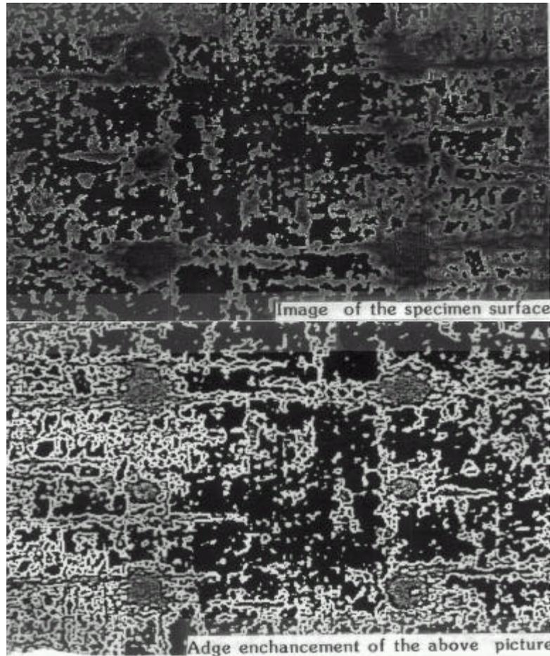
**Figure 15: Example of optical deformation measurement and microcracking activity investigation with the computer vision system.**
