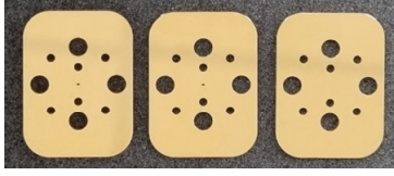
Fig. 1. WM-570 calibration standards. Long line (left), short line (center), and flush short (right).
