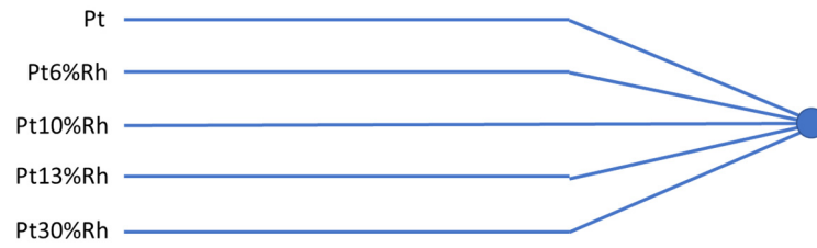
Figure 5. Schematic of a five-wire thermocouple assembly. The voltage can be measured across any two wires to make an individual thermocouple. All thermocouples are measuring the same temperature because they share a common measurement junction. (The pure platinum wire Pt0%Rh is labelled as Pt).
