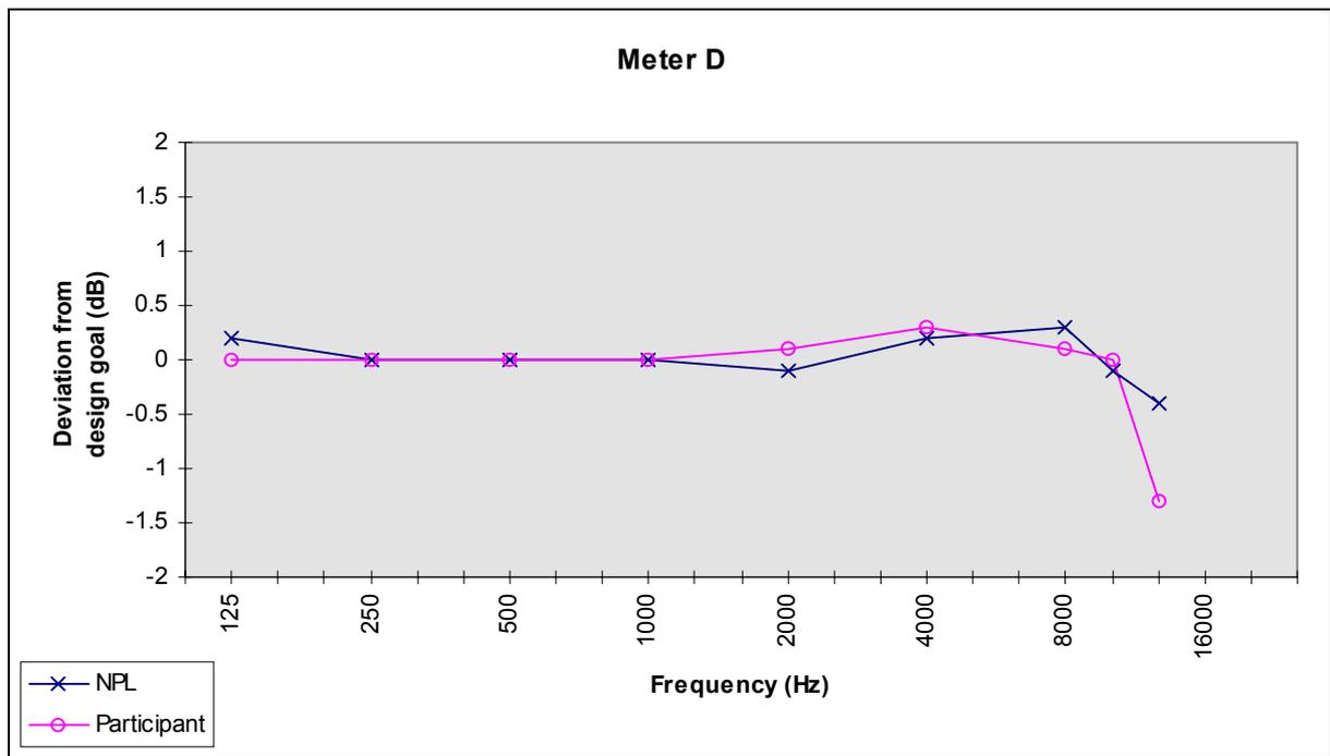
Figure 3 Deviations from design goal for sound level meter D for frequency weighting C (NPL) and for frequency response Lin. (participant) normalised to 1 kHz
