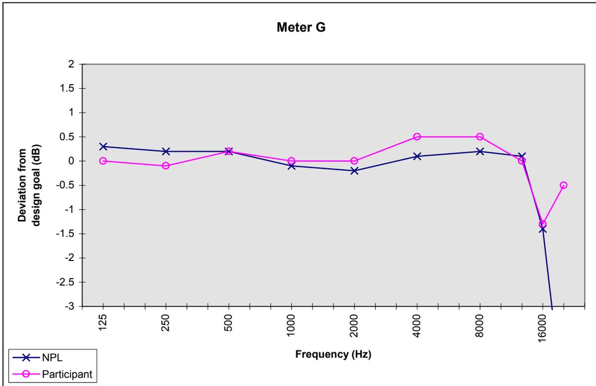
Figure 5 Deviations from design goal for sound level meter G for frequency weighting A
