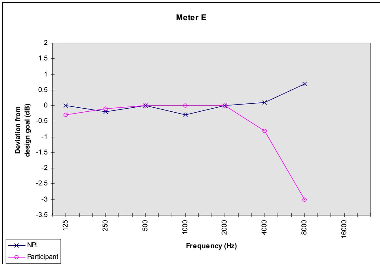
Figure 4 Deviations from design goal for sound level meter E for frequency weighting C
