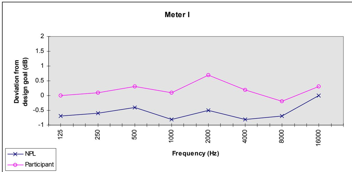
Figure 7 Deviations from design goal for sound level meter I for frequency weighting C
