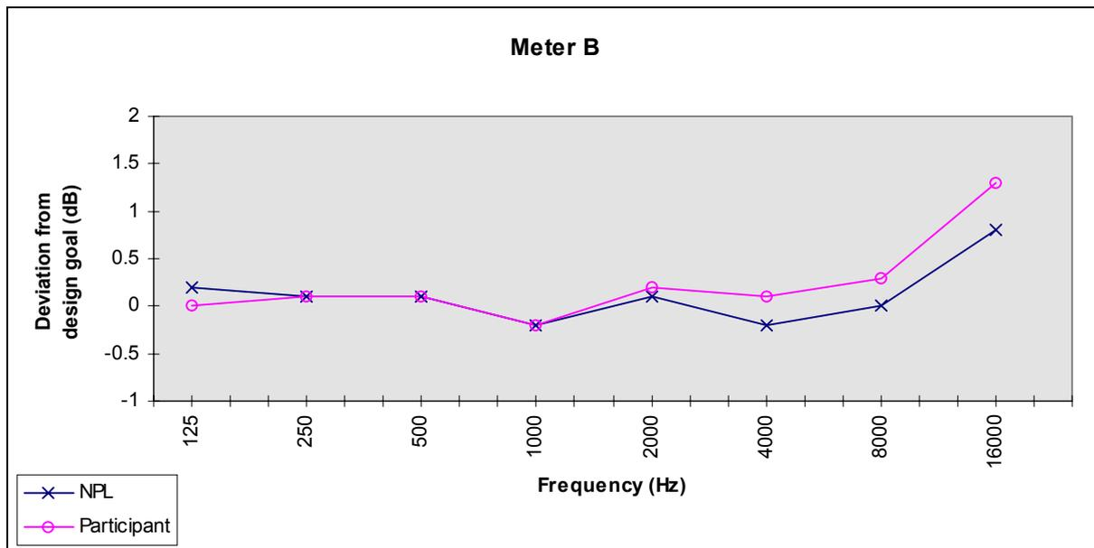
Figure 1 Deviations from design goal for sound level meter B for frequency response 'LIN'
