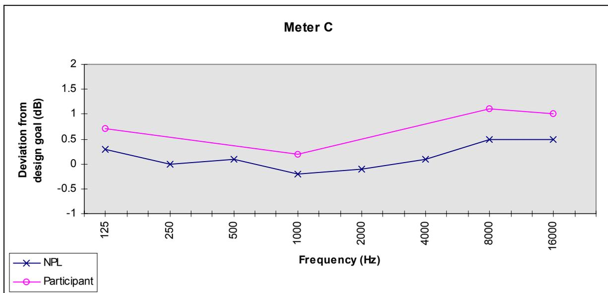
Figure 2 Deviations from design goal for sound level meter C for frequency weighting C (NPL) and for frequency weighting A (participant)
