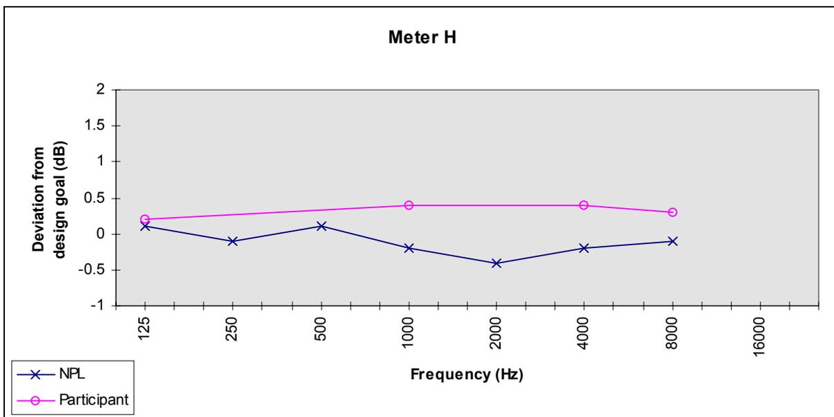
Figure 6 Deviations from design goal for sound level meter H for frequency weighting C (NPL) and for frequency weighting A (participant)
