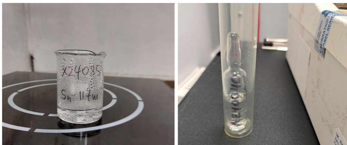
Figure 3: Photographs from the radiochemistry suite at NPL. The left picture shows the tin foil dissolving in 10 mL of 6M hydrochloric acid on a warming plate. The right picture shows the 5 mL ISO glass ampoule.
