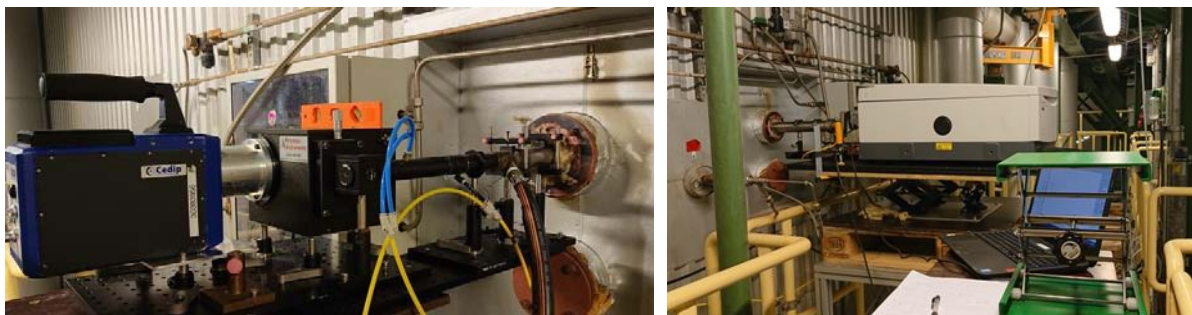
Figure 9. Parallel fast IR emission measurements with IR spectrometer and CEDIP IR camera (left panel: left boiler side) and FTIR spectrometer with sweeping probe (right panel: right boiler side). Both systems are viewing the same axis.
