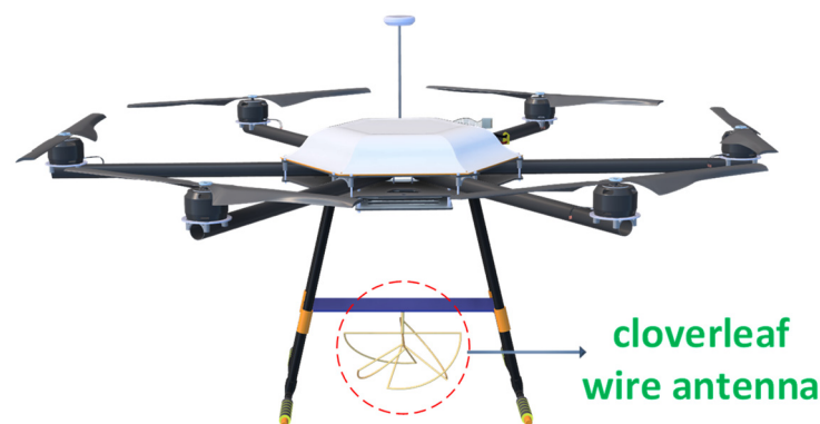
Figure 15. Hexacopter carrying cloverleaf wire antenna.
