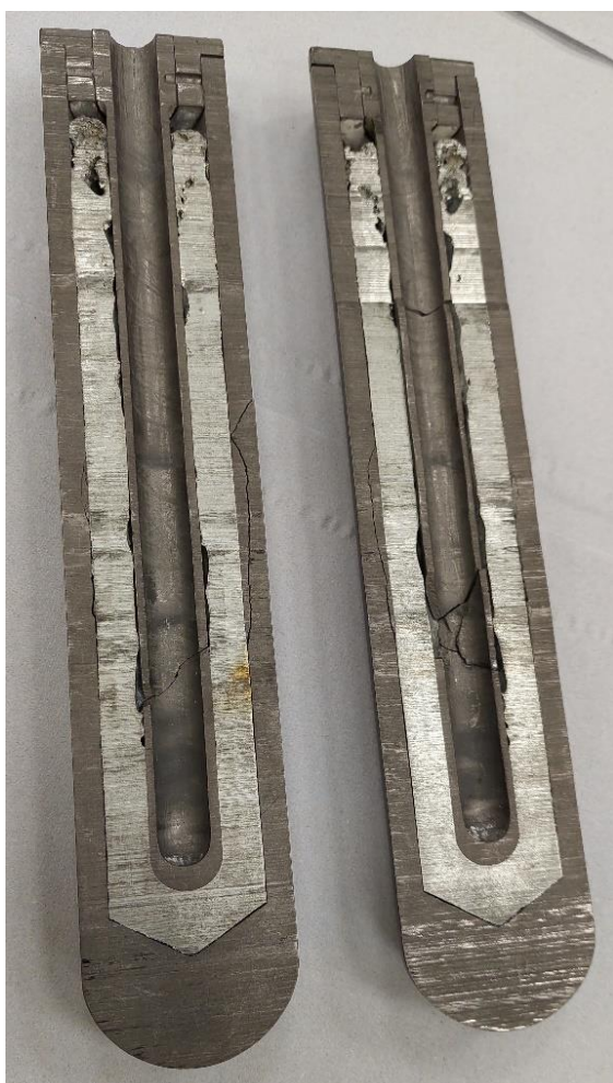
Figure 8. Section through a modern metallic (in this case tin) fixed point. The pure metal is contained within a graphite crucible. The thermometer being calibrated is inserted down the central well – courtesy of National Physical Laboratory.
