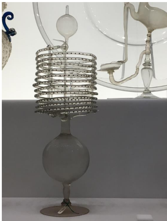
Figure 2. Photograph of spiral thermometer, the scale indicated by blue enamel markers, – courtesy of Museo Galileo Istituto e Museo di Storia della Scienza, Firenze.
