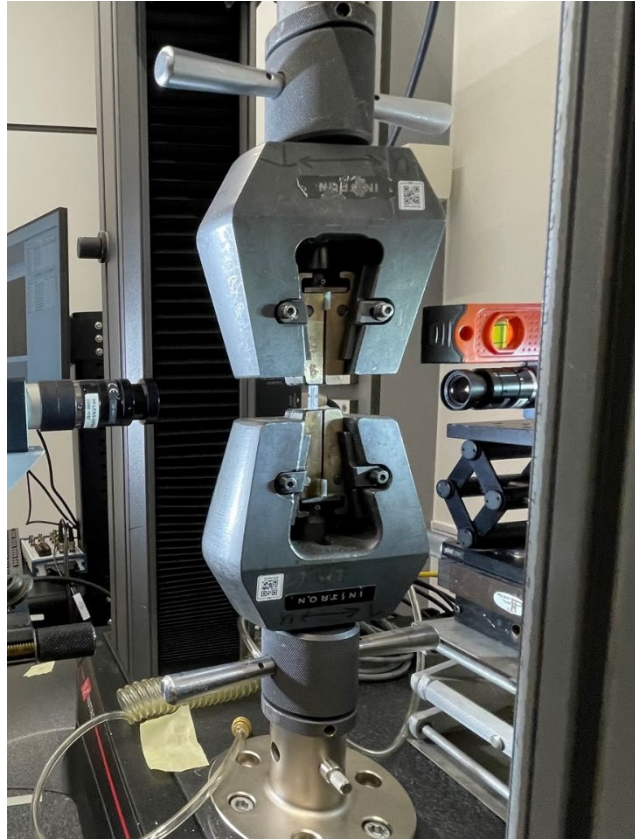
Figure 7 Instron universal test machine setup used for testing with cameras imaging front and back faces of the test piece simultaneously for strain measurement
