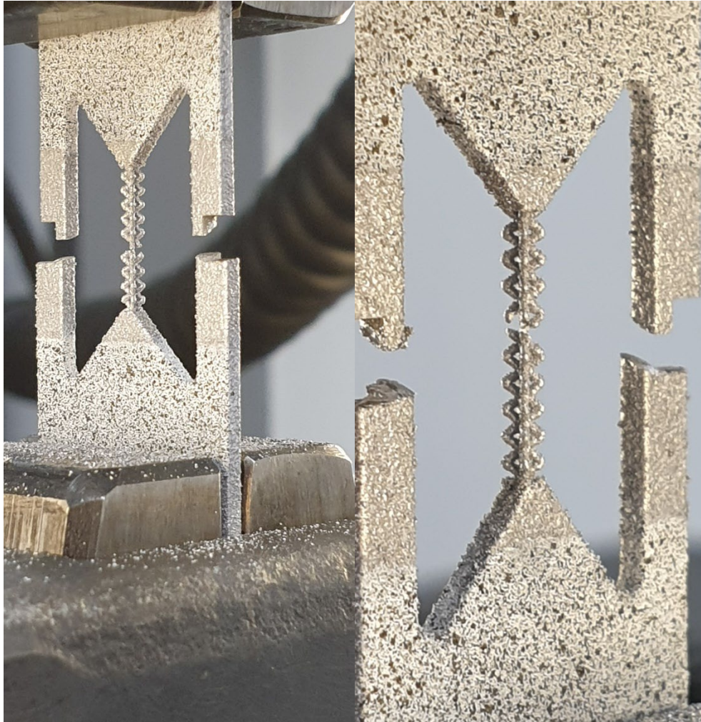
Figure 26 0.40 mm 1 x1 x 9 lattice test pieces after testing
