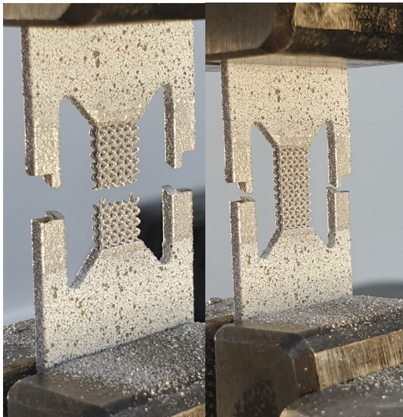
Figure 32 0.40 mm 5 x 1 x 9 lattice test pieces after testing
