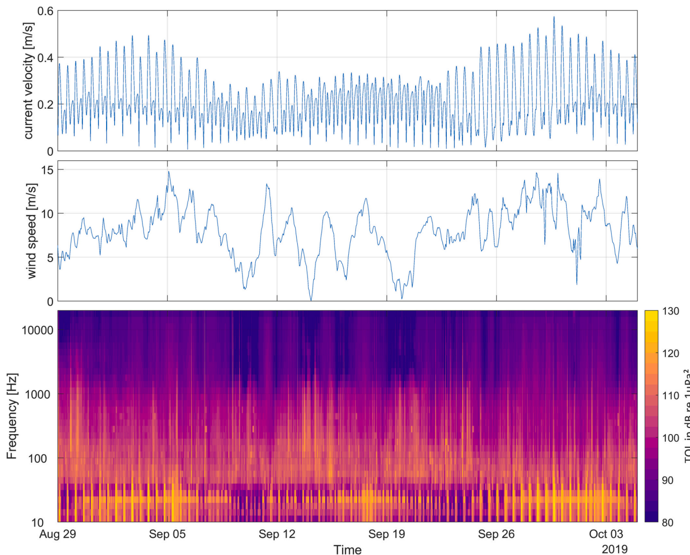
Fig. 3. Bottom current velocities (top), wind speeds (middle) and spectrogram of measurements (bottom); lower frequencies (< 50 Hz) are distorted by tidal flow noise; two-weekly neap-and spring tide is visible, dominated by semi-diurnal tidal constituents; TOLs for frequencies above 1 kHz can be found to increase with higher wind speeds (example from August–October 2019 at location 07-NL-TEX).
