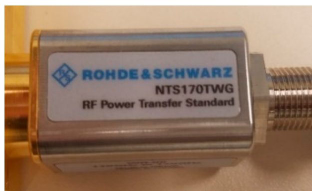
Figure 1. The thermoelectric power sensor manufactured by Rohde & Schwarz, designed to operate from 110 GHz to 170 GHz.
