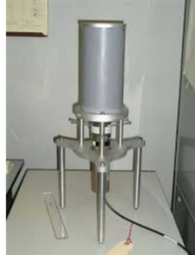
Figure 2. The international reference system for short-lived gamma-emitting radionuclides (SIRTI). The instrument comprises a NaI(Tl) detector in a lead shield, mounted on a tripod. Samples for measurement are placed in a well in the detector (not visible in the photograph).
