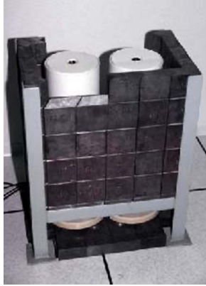
Figure 1. The ionization chambers used for the international reference system for gamma-emitting radionuclides (the SIR) at the BIPM. The photograph was taken during construction of the instrument with the lead shield partially completed and it shows two re-entrant ionization chambers (the second chamber is a back-up in case of problems with the main instrument). NMIs send a sample of the radionuclide in solution in a glass ampoule; the ampoule is placed in a holder and lowered into the well in the chamber (the hole can be seen at the top of the chambers). The current produced in the chamber is proportional to the activity of the radionuclide in the sample.
