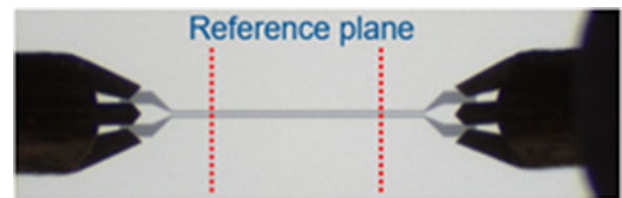
Figure 8. Microscopic image of an on-wafer S-parameter measurement of a CPW transmission line.
