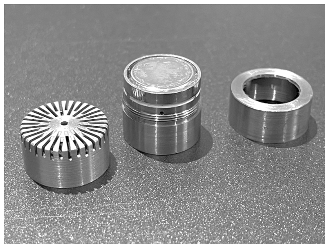
Figure 8. The Brüel and Kjær type 4134 microphone with its regular protection grid (left), and UA0825 adapter (right) for converting to laboratory standard configuration. The microphone pressure-equalisation vent outlet is visible just above the thread.
