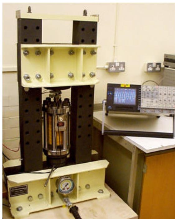
***Figure 22: Photograph of Plint rig and magnetostrictive actuator set up for fatigue measurements***
