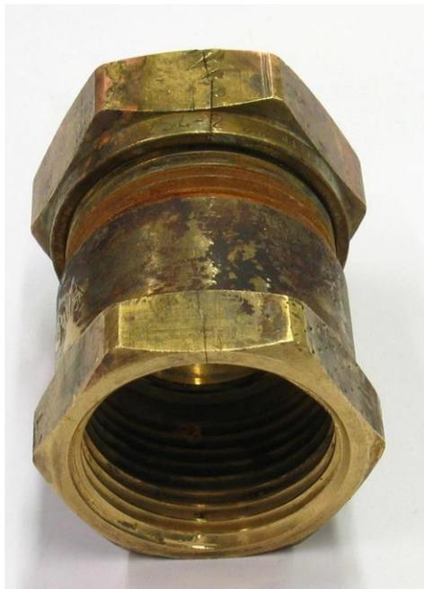
**Figure 7.** *Stress corrosion cracking in a brass fitting.*
