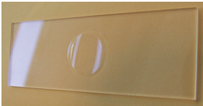
Figure 2 - Single well glass microscope slide used to calibrate SAM ToF thickness methodology.
