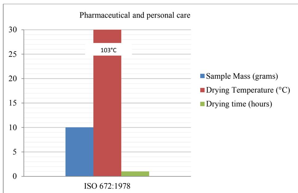
Figure 6 Comparison of measurement conditions for pharmaceutical and personal care
