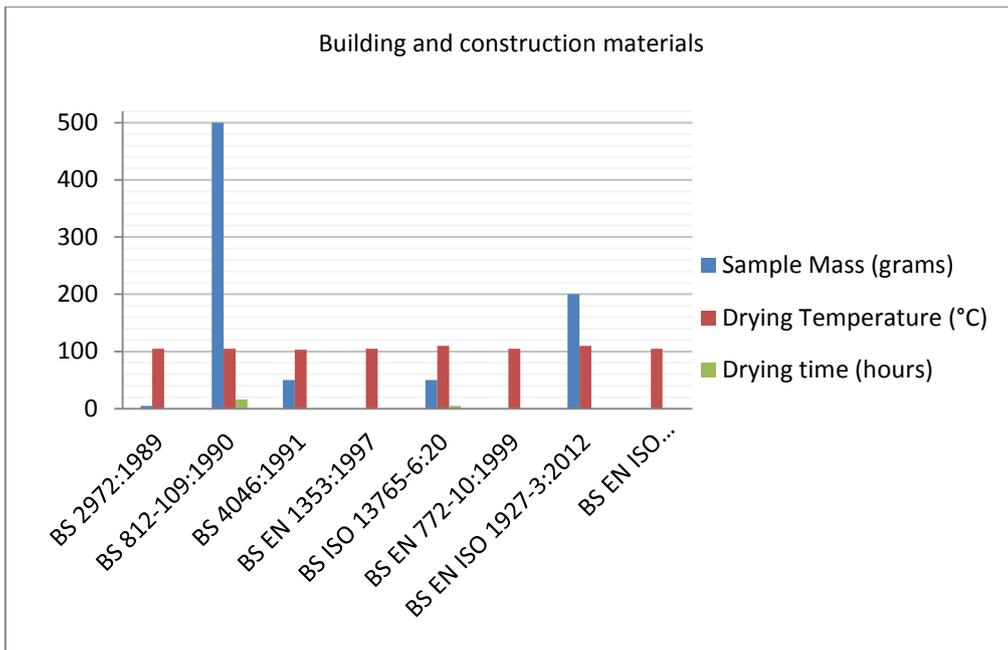
Figure 4 Comparison of measurement conditions for building and construction materials
