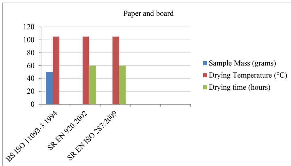
Figure 1 Comparison of measurement conditions for paper and board
