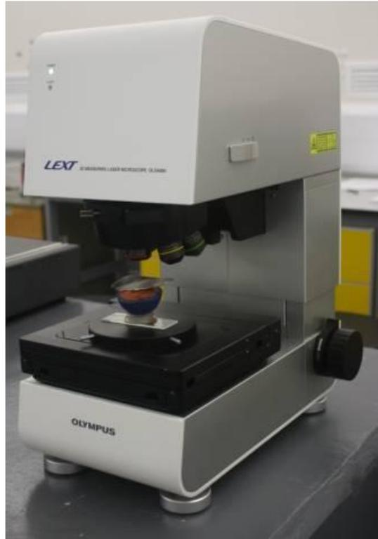
**Figure 2 Imaging confocal microscope used (Olympus OLS 4000)**
