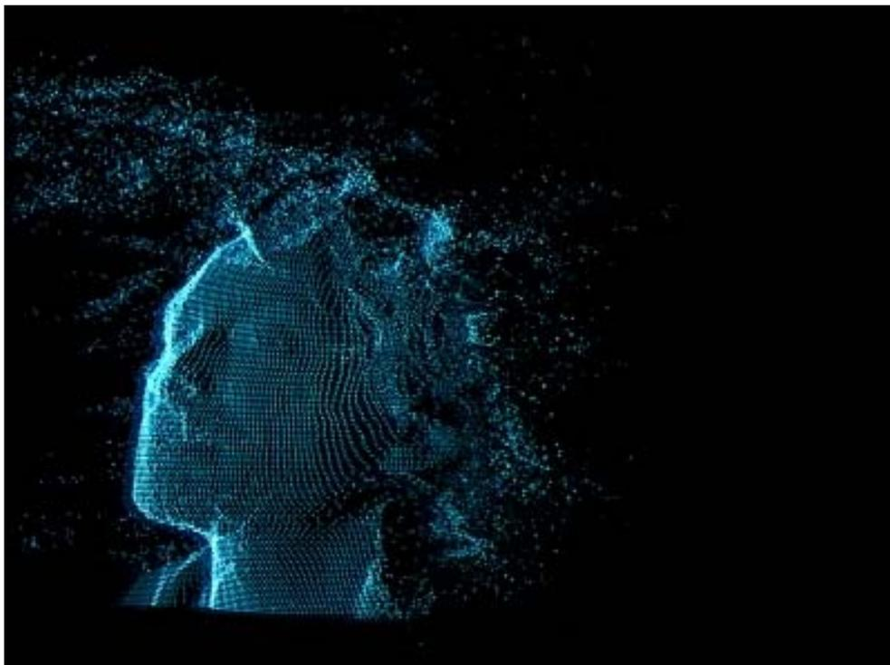
**Figure 7. A point cloud captured in real time using a structured light scanner**
