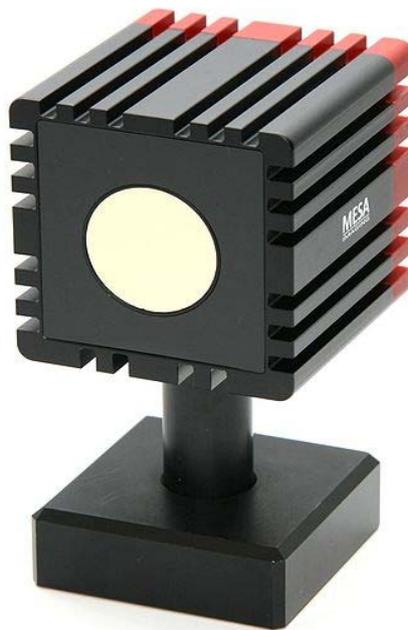
Figure 8. The Mesa time-of-flight camera
