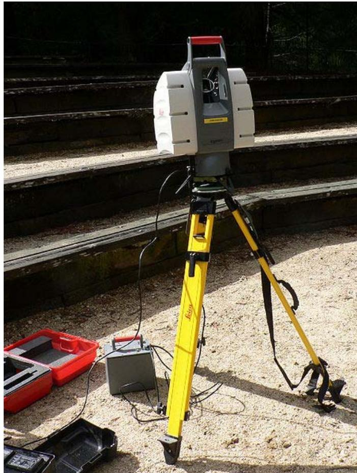
Figure 6. A commercial laser scanner
