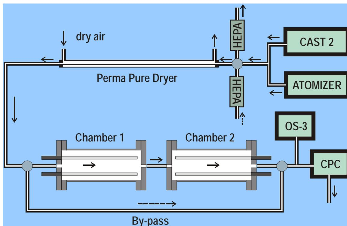
**Figure 1: Schematics for testing of UV/ozone cleaning prototype, in order to distinguish from background (particularly carbon) particles**
