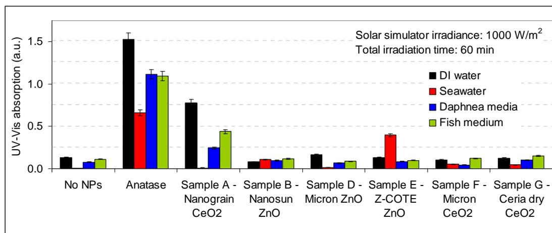
**Figure 4. Absorbance readings at 352 nm, of PROSPECT NMs in 4 different media (DI water, seawater, daphnia and fish media) after being irradiated with solar simulator at  $1000 \text{ W/m}^2$ , for 60 minutes. Anatase NM dispersed in the four different media was used as positive control; media with no NMs were used as a negative control. The values are normalized to the absorption measured for the negative control in DI water.**
