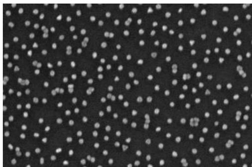
Fig 1. Scanning electron microscopy (SEM) image of 20 nm Au NPs mounted onto Si surface
