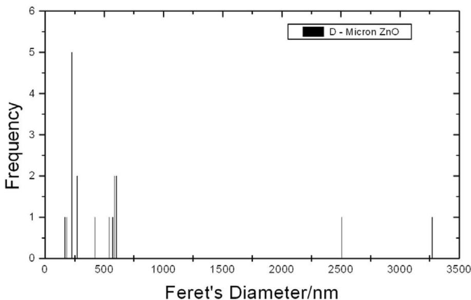
**Figure 1. Distribution of primary particle size (Feret's diameter) measured using image analysis of SEM micrographs for Micron ZnO.**
