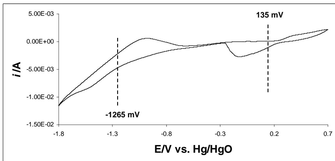
**Figure 5.** A typical cyclic voltammogram of PROSPeCT Z-COTE ZnO electrode (BASF, Germany), batch number ZC250#37#RP.
