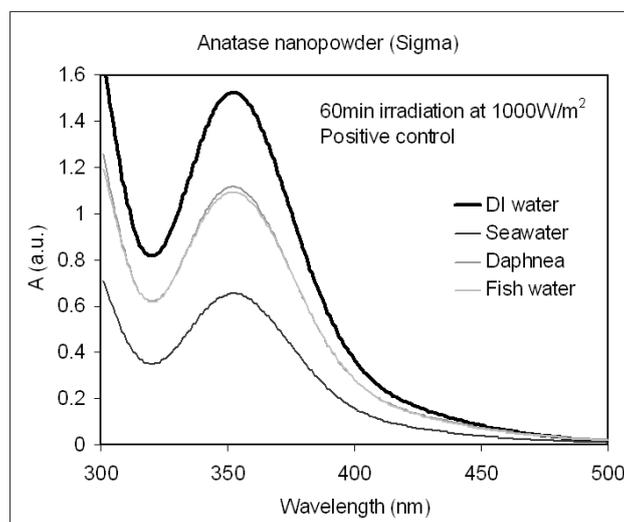
**Figure 3. UV-Visible absorption spectra of Anatase NM (positive control) in 4 different media (DI water, seawater, daphnia and fish media) after being irradiated with solar simulator at  $1000 \text{ W/m}^2$ , for 60 minutes.**
