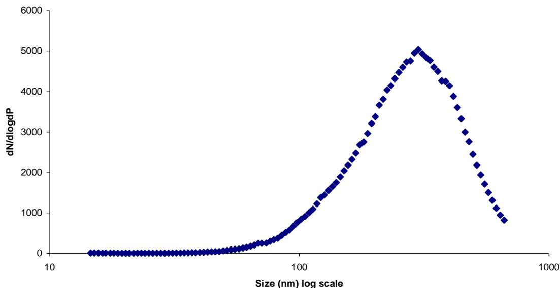
**Figure 6. SMPS spectrometer data of Z-COTE ZC250#56#01. Normalised concentration vs. particle diameter data, taken from stable 51-hour segment of sampling time. The powder sample was aerosolised using a fluidised bed aerosol generator prior to SMPS analysis. Data was taken from a stable 51-hour segment of sampling time; this plot thus display the mean size distribution of the aerosolised powder over this time.**
