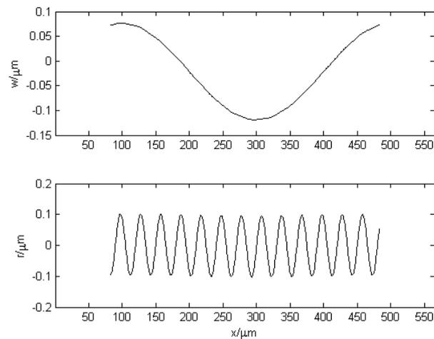
Figure 2: Waviness profile (top) and roughness profile (bottom) after application of a  $\lambda_c$  filter to the primary profile.
