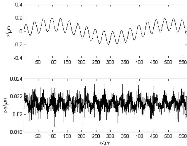
Figure 1: Simulated measured profile (top) and the differences between the measured and primary profiles (bottom) after mean centering and application of a  $\lambda_s$  filter to the measured profile when  $\rho_z = 0$ .
