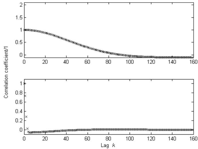
Figure 7: Correlation coefficients, as a function of lag  $k$ , associated with the ordinate values defining the waviness (top) and roughness (bottom) profiles, determined using the GUM uncertainty framework.
