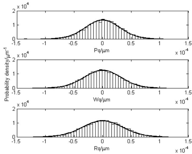
Figure 9: Approximations to the PDFs for the quantities  $P_q - p_q$  (top),  $W_q - w_q$  (middle) and  $R_q - r_q$  (bottom), where  $p_q$ ,  $w_q$  and  $r_q$  are the estimates of, respectively,  $P_q$ ,  $W_q$  and  $R_q$  obtained using the GUM uncertainty framework. The results provided by the GUM uncertainty framework are shown as continuous Gaussian PDFs, and those provided by a Monte Carlo method as scaled frequency distributions (histograms).
