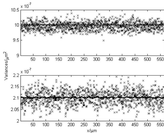
Figure 25: Variances associated with the  $x$ -coordinates (top) and  $z$ -coordinates defining the primary profile. The variances determined using the GUM uncertainty framework are shown as the black continuous line; those determined using a Monte Carlo method are shown as crosses.
