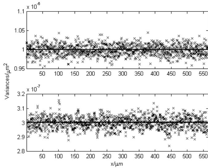
Figure 3: Variances associated with the ordinate values defining the measured (top) and primary (bottom) profiles. The variances determined using the GUM uncertainty framework, which are the same for each ordinate value, are shown as the horizontal line; those determined using a Monte Carlo method are shown as crosses.
