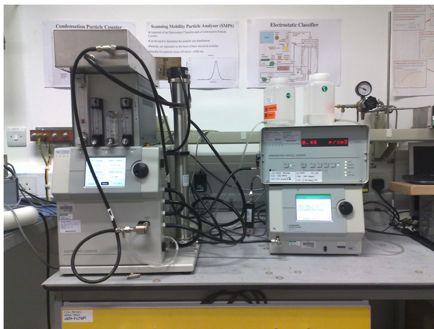
Figure 6: A production SMPS drier system during calibration at NPL.
