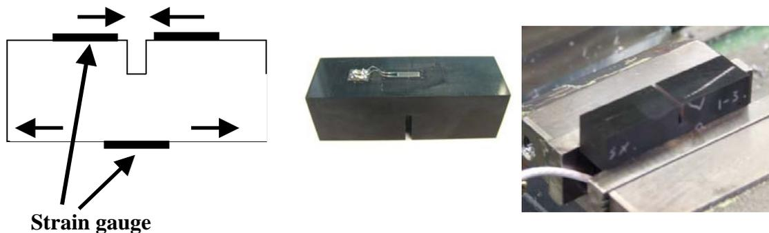
**Figure 6** *Incremental slitting method*
