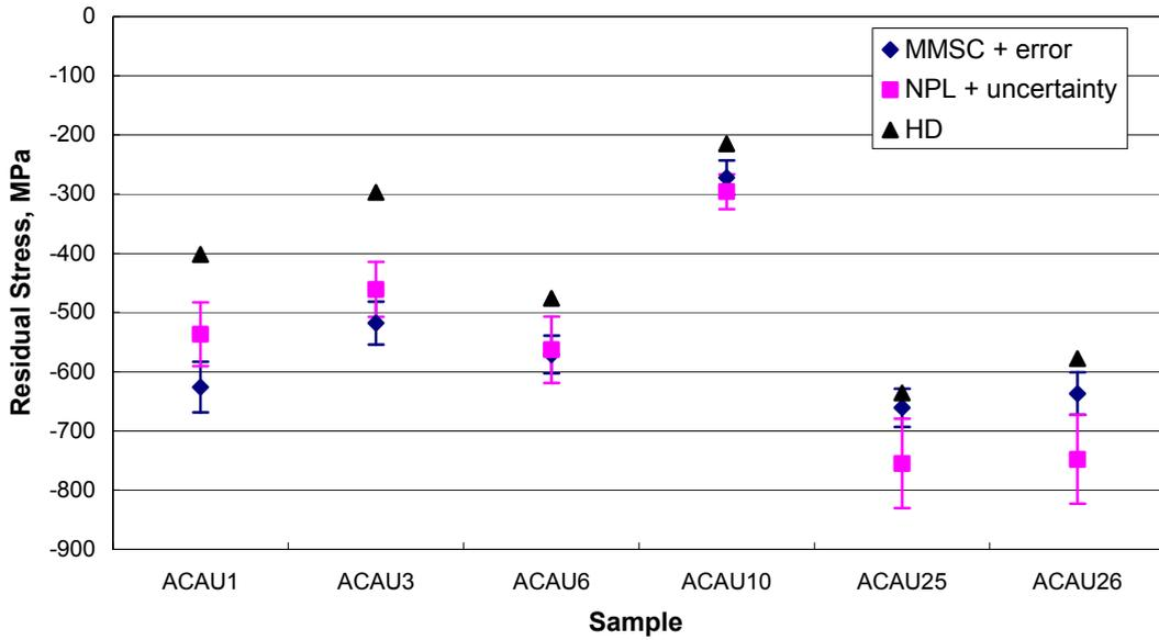
**Figure 1.** Comparison of axial residual stress values in shot-peened 300 M steel determined from XRD measurements from MMSC and NPL and from incremental hole-drilling data (at a depth of 8  $\mu\text{m}$  in this case).
