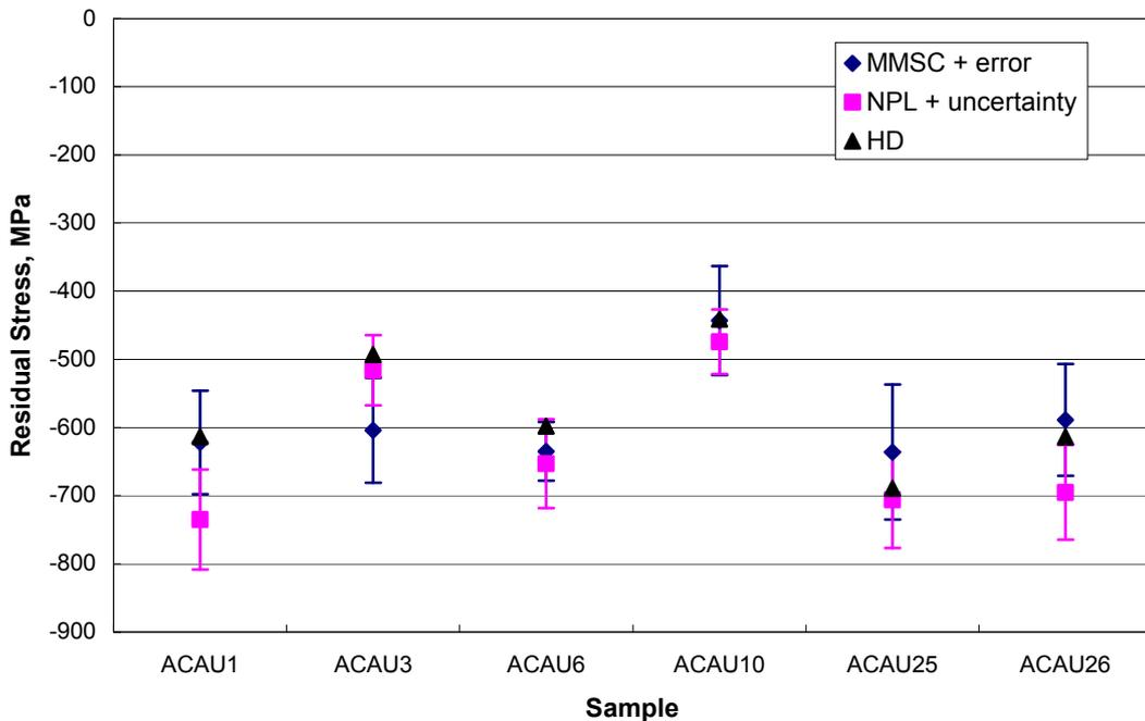
**Figure 2.** Comparison of circumferential residual stress values in shot-peened 300 M steel determined from XRD measurements from MMSC and NPL and from incremental hole-drilling data (at a depth of 8  $\mu\text{m}$  in this case).
