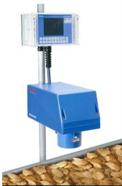
**Figure 6: NIR reflectance used to measure moisture content in crisps**
