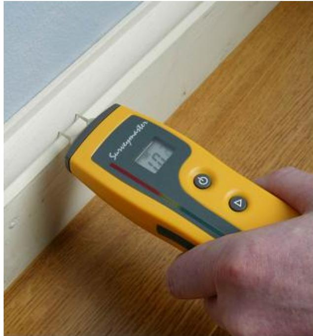
**Figure 5: Measuring the moisture content of wood with resistance probes**
