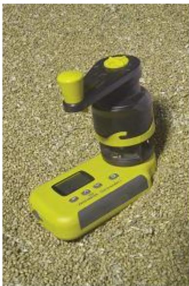
**Figure 7: Grain moisture meter with grinder**
