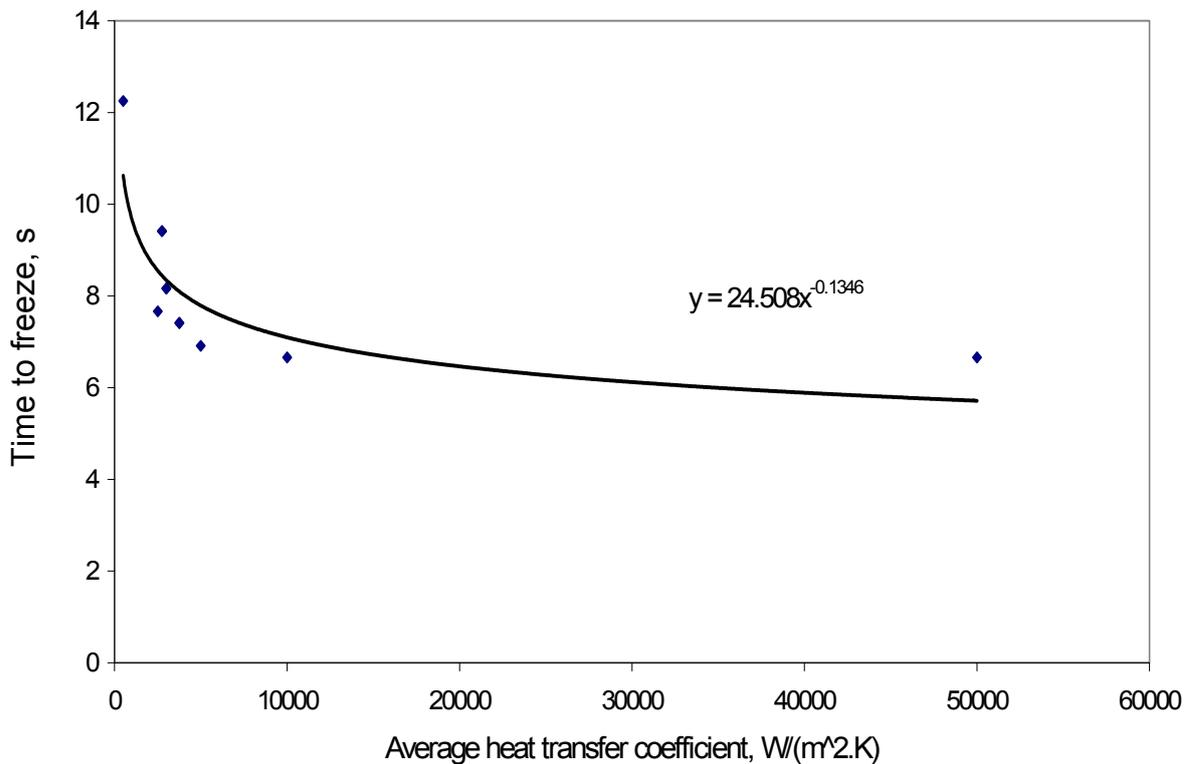
**Figure 3. Effect of average of symmetric and asymmetric core and cavity heat transfer coefficients on time to freeze for a 2 mm thick 10 mm diameter disc.**
