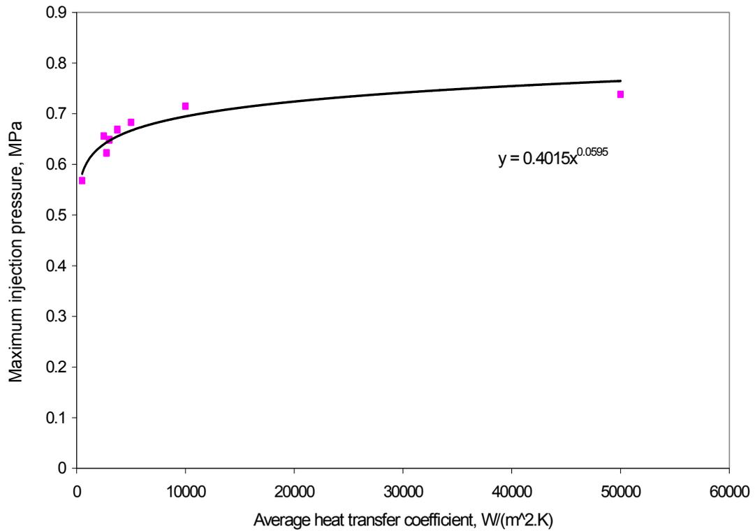
**Figure 5. Effect of average of symmetric and asymmetric core and cavity heat transfer coefficients on maximum injection pressure for a 2 mm thickness, 10 mm diameter disc.**
