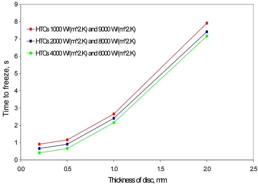
**Figure 6. Effect of asymmetric values of core and cavity heat transfer coefficients totalling  $10,000 \text{ W}/(\text{m}^2 \cdot \text{K})$  on time to freeze for 10 mm diameter discs of varying thicknesses.**
