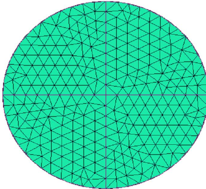
**Figure 1. Midplane mesh model of 10 mm disc.**
