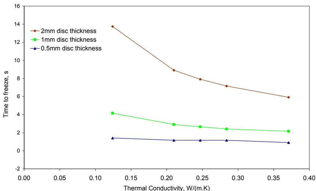
**Figure 8. The effect of varying thermal conductivity of HDPE on the time to freeze of moulded discs of different thicknesses.**
