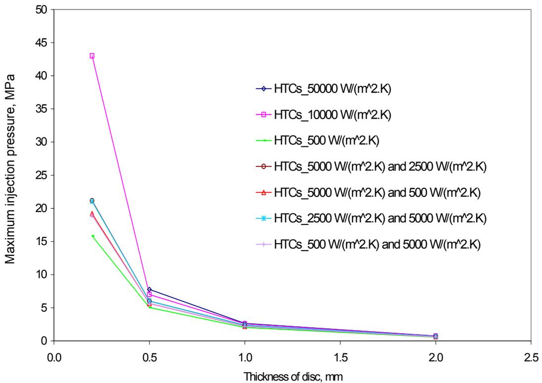
**Figure 4. Effect of asymmetric and symmetric values of core and cavity heat transfer coefficients on maximum injection pressure for 10 mm diameter discs of varying thicknesses.**
