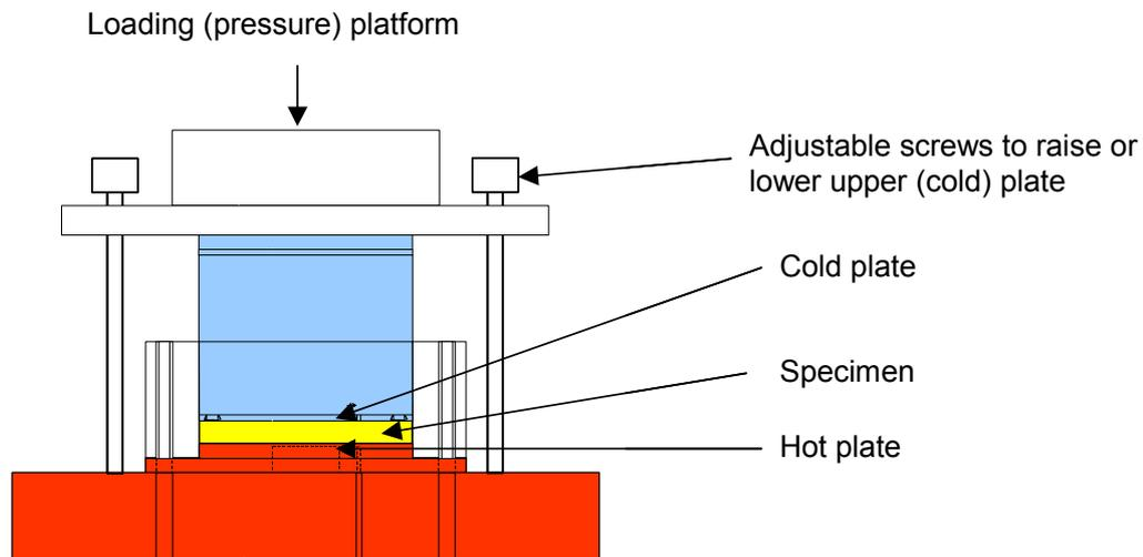
**Figure 1: Heat transfer coefficient apparatus.**
