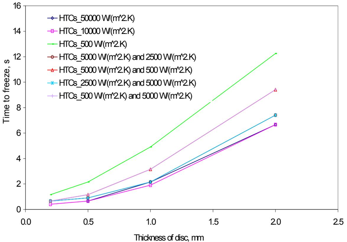
**Figure 2. Effect of asymmetric and symmetric values of core and cavity heat transfer coefficients on time to freeze for 10 mm diameter discs of varying thicknesses.**
