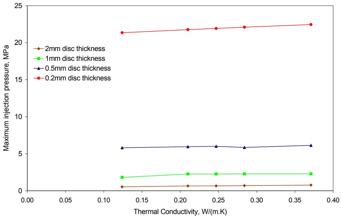
**Figure 7. The effect of varying thermal conductivity of HDPE on the maximum injection pressure of moulded discs of different thicknesses.**
