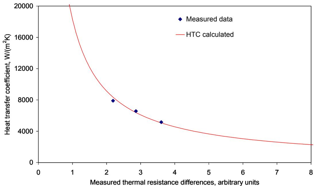
**Figure 9: Effect of errors on derived heat transfer coefficients**
