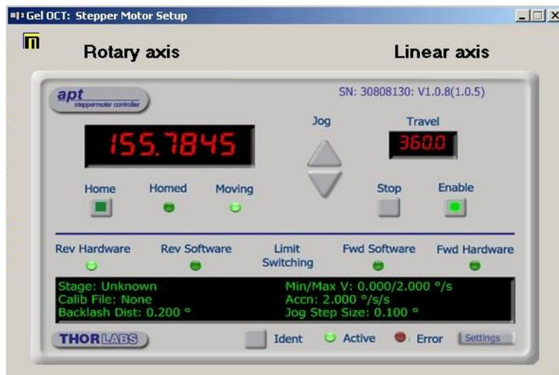
Figure B2. The stepper motor set-up
