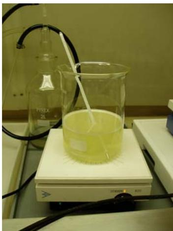
Figure A1. Stirring the heated gelatin/H<sub>2</sub>SO<sub>4</sub> solution
