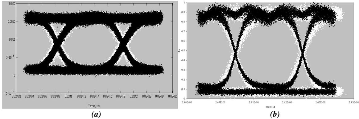
**Figure 1, (a) IQ improvement: Eye diagram with raw data (white) and IQ corrected data (black). The black data has 50% less jitter than the white data; (b) Pulse-Carving improvement: Eye diagram with normal optical signal (white) and retimed optical signal (black), the black data has 68% less jitter the white data.**
