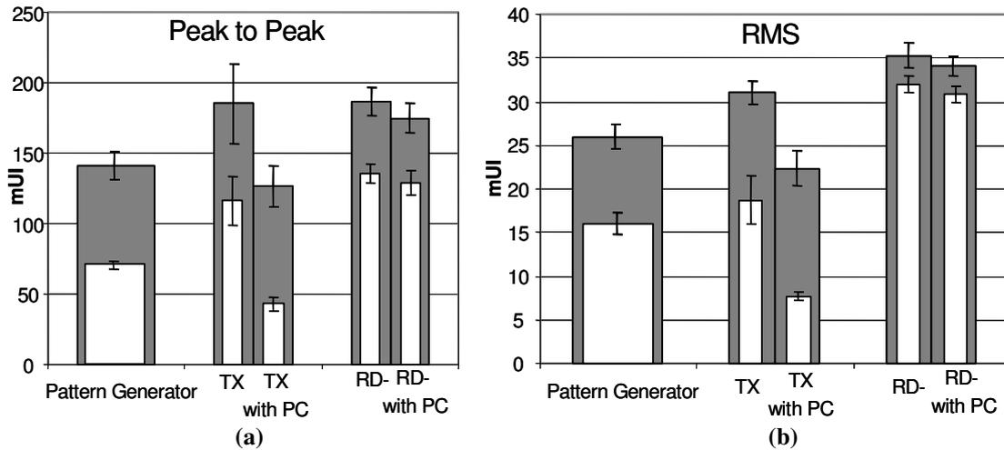
Figure 3, (a) Peak to Peak and (b) RMS jitter. Grey histograms are jitter without IQ correction, white histograms are jitter with IQ correction.
