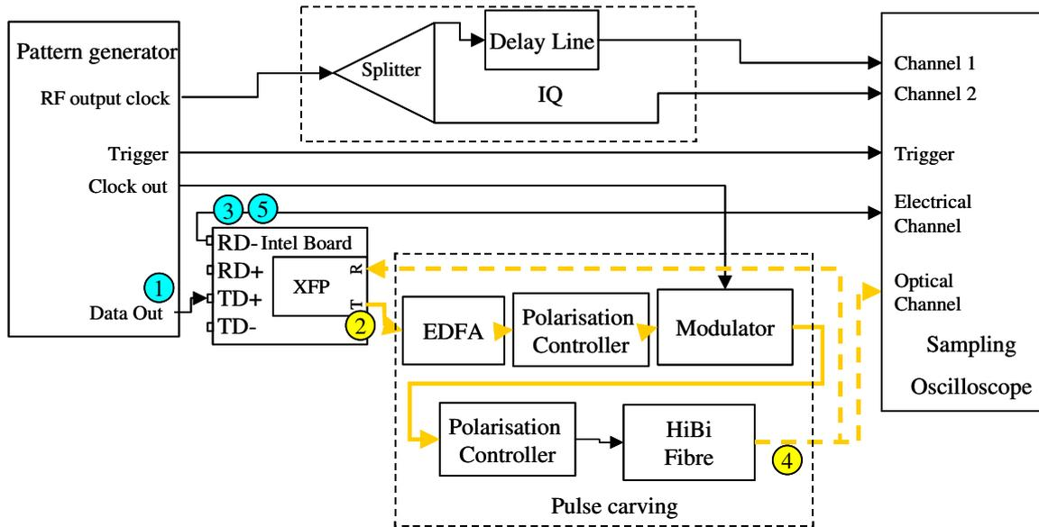
Figure 2, Experimental set-up. Jitter have been measured at different points in the system (1-5).
