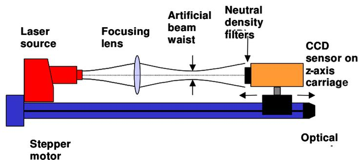
Figure 1.  $M^2$  System layout.
