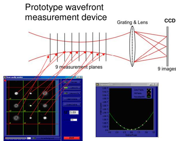
**Figure 3.** Prototype wavefront sensor utilising a multiple distorted diffraction grating
