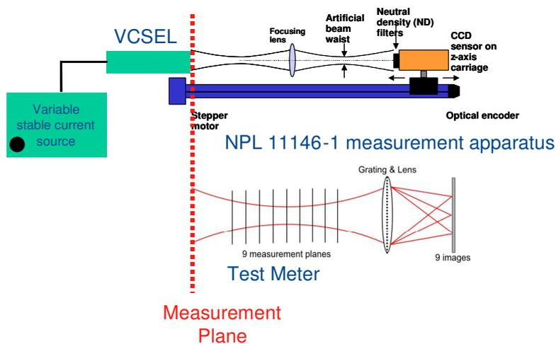
**Figure 4.** Comparative measurement of test meter vs. NPL ISO 11146 system.
