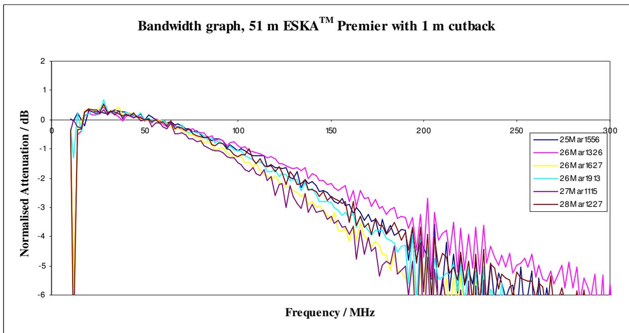
**Figure 3** Graph showing normalised transmission plot through a length of 51 m ESKA™ step index fibre with an estimated bandwidth of 145 MHz. A reference of 50 MHz was chosen arbitrarily as this represented the lowest frequency at which signal levels were stable.
