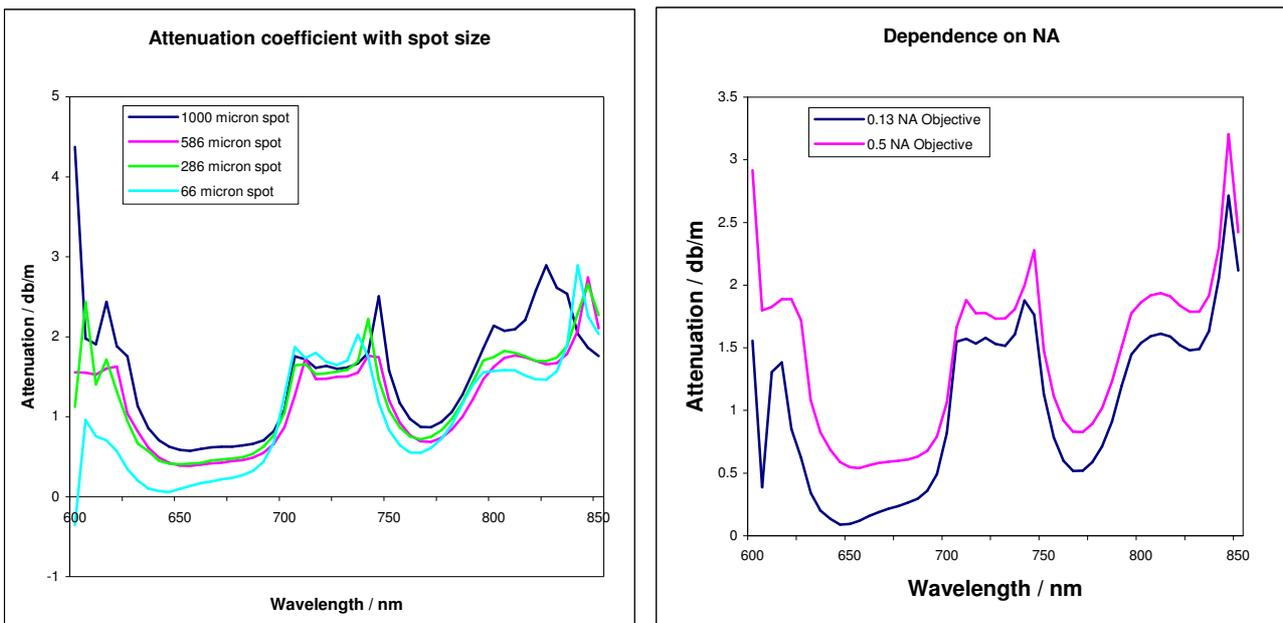
**Figure 2** Graphs showing variations in attenuation with NA and spot size using a multistep index OM-GIGA fibre with fibre lengths of  $\sim 11$ -12 m. NAs quoted are the design NA of the objectives used.
