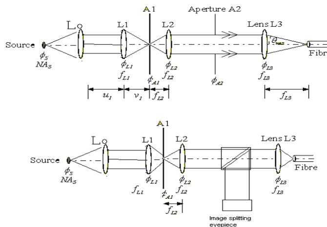
**Figure 1** Optical design of launch module with pinhole at A1 for spot size selection. An aperture A2 provides control of  $NA$  at low values. High  $NA$  requires appropriate selection of lenses L2 and L3. The use of a beamsplitter between L2 and L3 facilitates viewing and measurement of the end face of the fibre under test.
