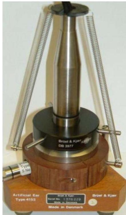
*Figure 2. Transmitter microphone coupled to the ear simulator*
