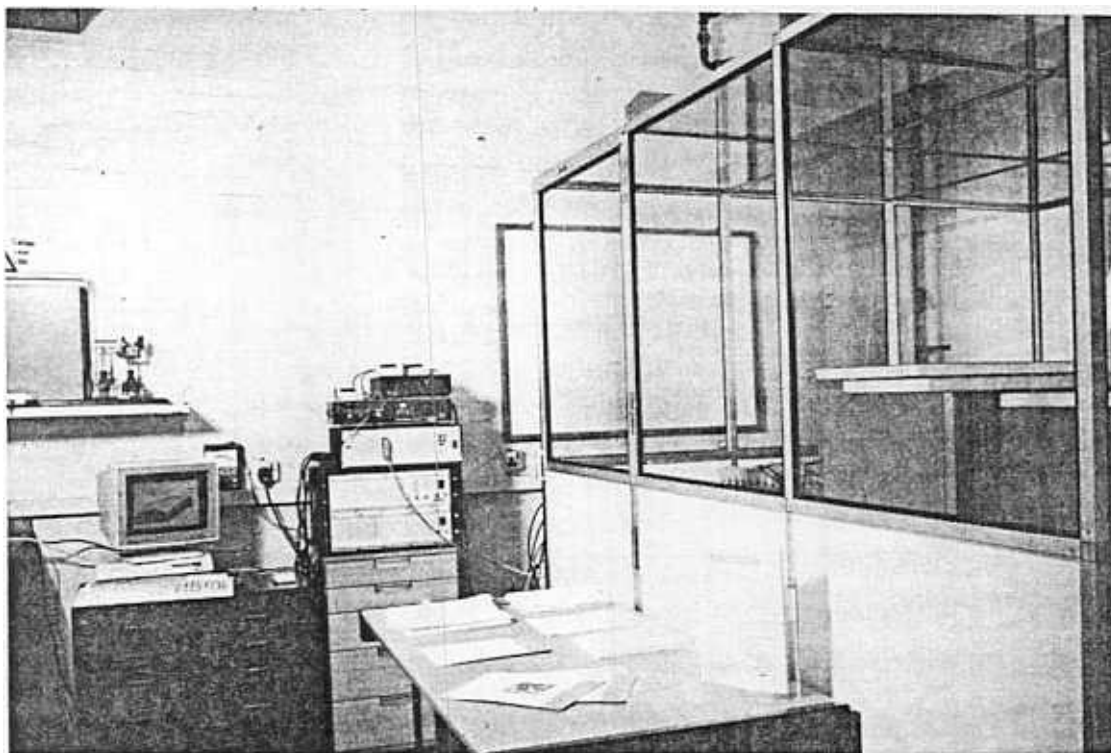
Figure 2(a). Shows enclosures to overcome acoustic noise and temperature instability. Ancillary control equipment is placed outside the main enclosure.
