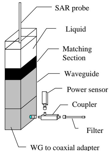
Figure 1: Waveguide system
