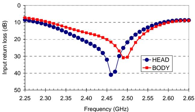
Figure 2: Measured input return loss of waveguide system with liquid.
