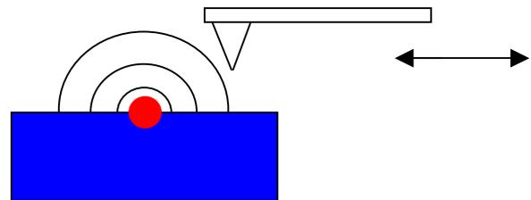
Figure 1. Magnetic field distribution generated by current carrying conductor and imaged by the scanning tip.
