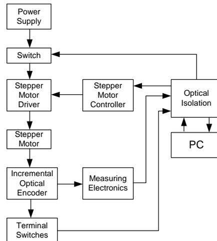
the stepper motor is measured relevant to a known initial position using an incremental encoder. From the in-phase and the quadrature-phase signals of the incremental optical encoder, the incremental position and the direction of motion can be determined by using one counter and one D-type flip-flop.
