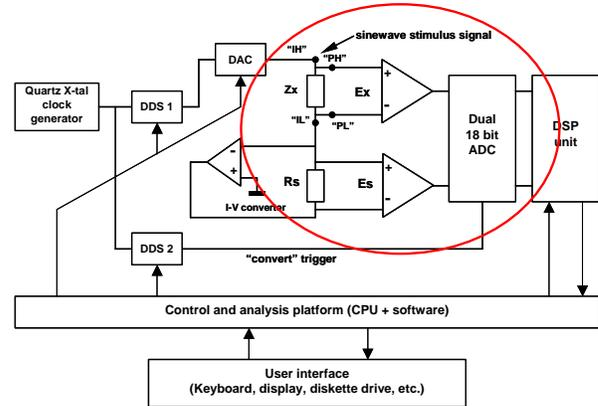
Figure 2: Schematic diagram of the LCR meter, with the core measurement part indicated by the circle.
