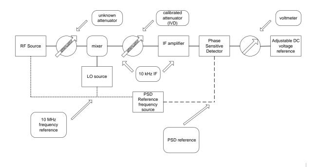
Figure 1: AF Series Substitution System For clarity, impedance matching and RF isolation components have been omitted from the diagram.
