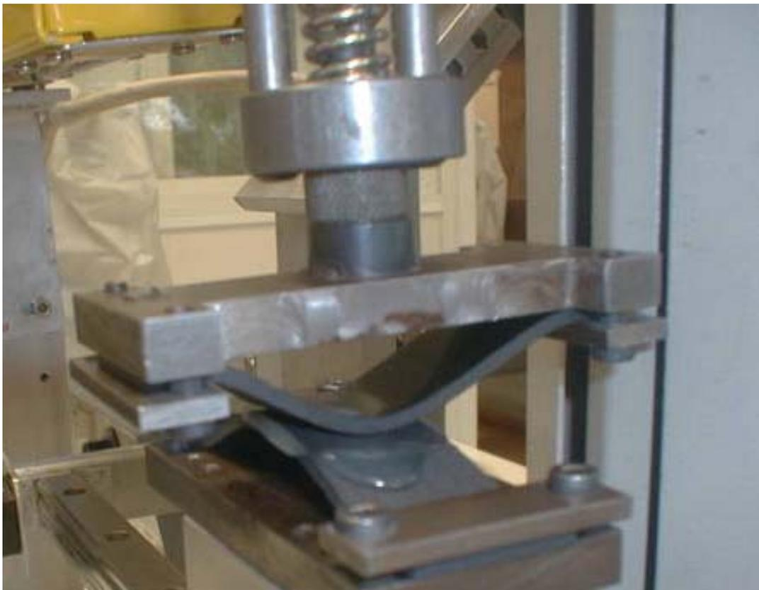
**Figure 6: Bond strength tack testing**
