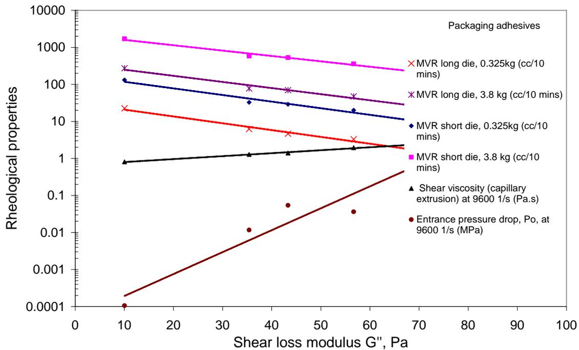
**Figure 9: Correlation of melt flow rate and capillary extrusion results with shear loss modulus results (for units of rheological properties see legend)**
