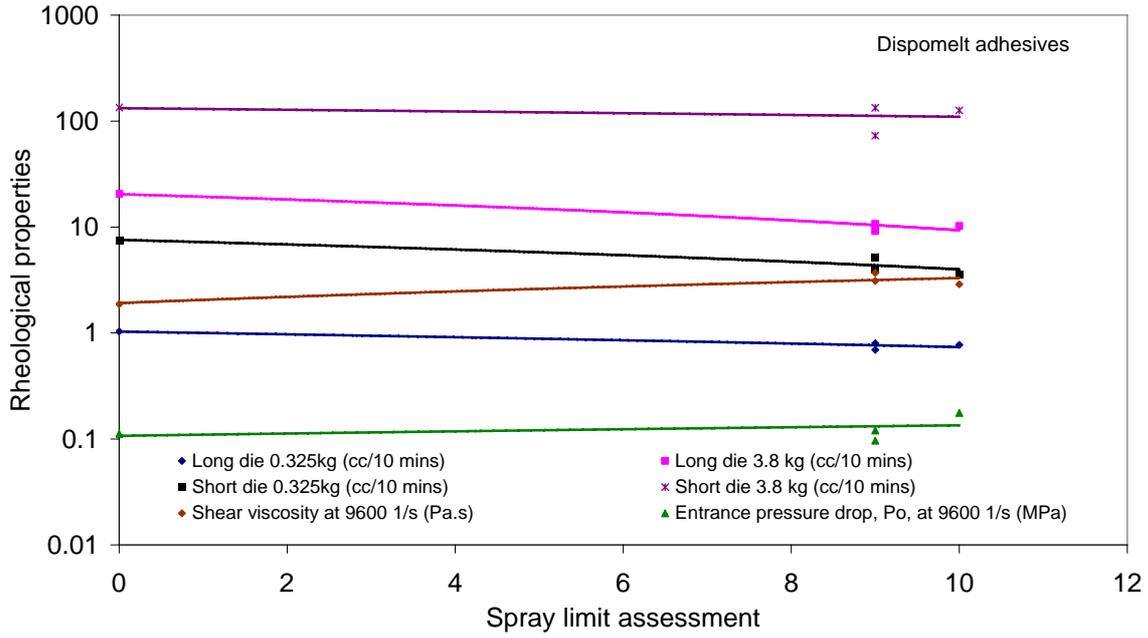
**Figure 19: Correlation of spray limit assessment with rheological properties (for units of rheological properties see legend)**
