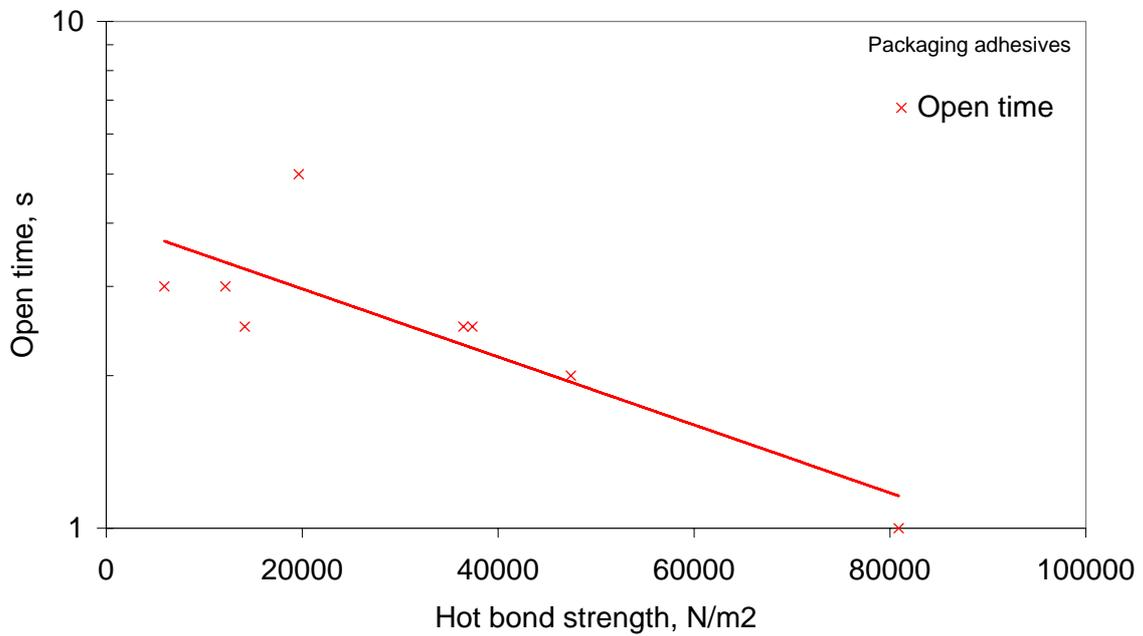
**Figure 13: Correlation of open time with hot bond strength (tack)**
