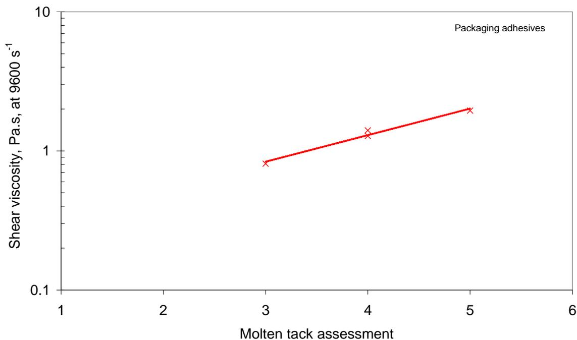
Figure 18: Correlation of molten tack assessment with shear viscosity
