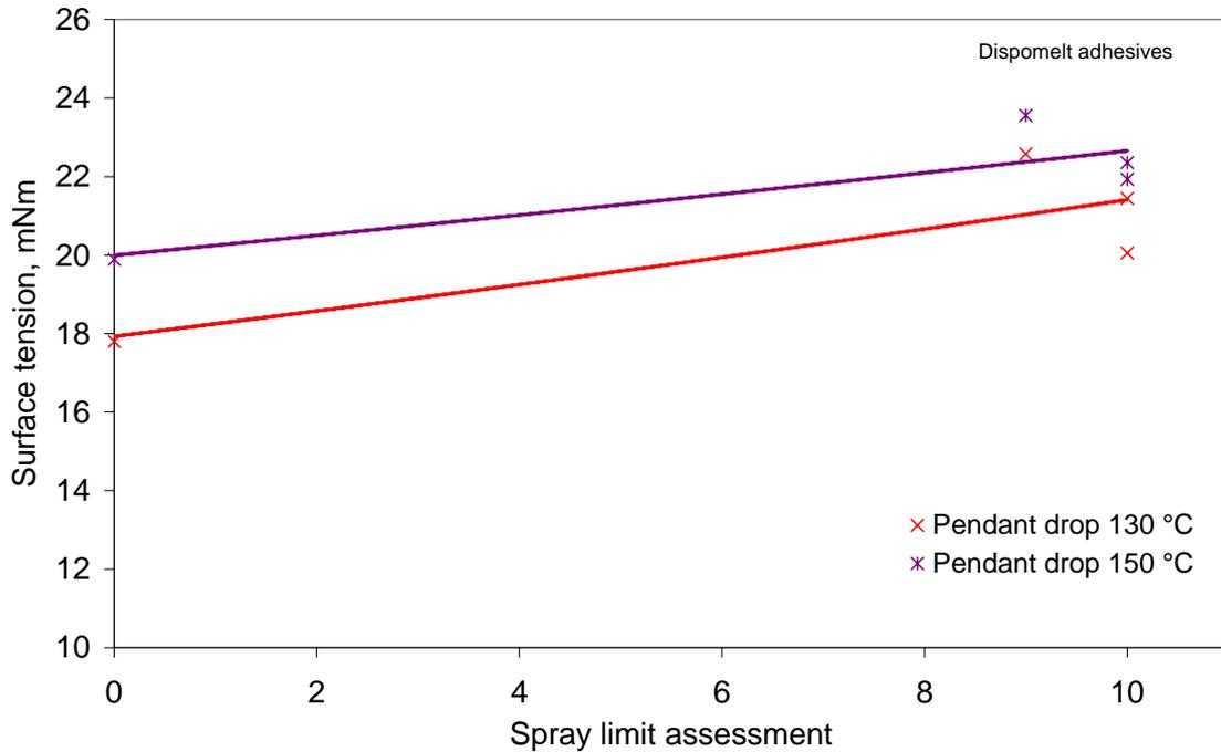
**Figure 20: Correlation of surface tension and spray limit evaluation**
