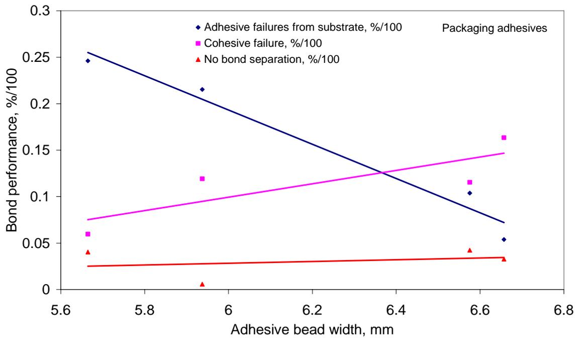
**Figure 15: Correlation of bond performance with adhesive bead width**
