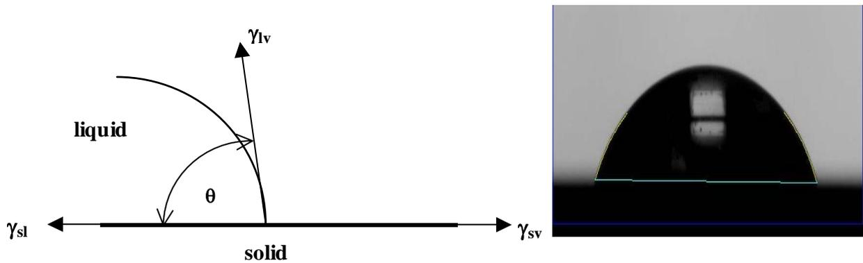
**Figure 5: Contact angle of a liquid on a solid surface**
