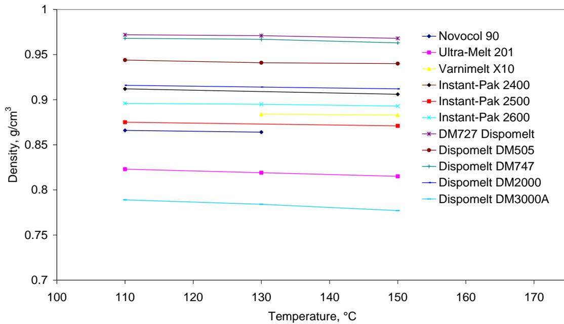
**Figure 2: Density values for packaging and Dispomelt hot melt adhesives**
