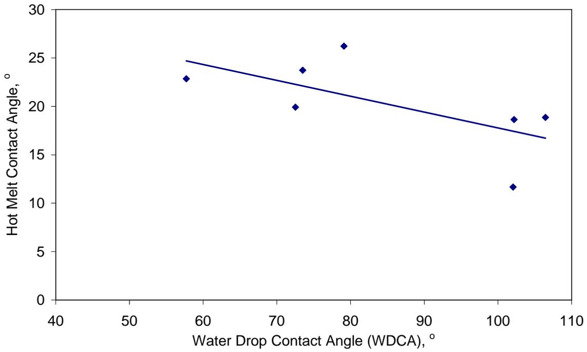
**Figure 10a: Relationship between the measured contact angles of a molten hot melt adhesive on a selection of packaging surfaces and the water drop contact angle (room temperature)**
