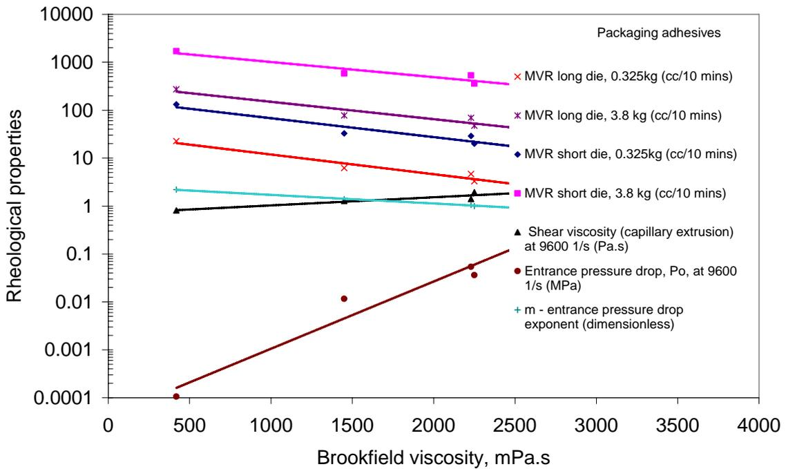
Figure 8: Correlation of melt flow rate and capillary extrusion results with the Brookfield viscosity (for units of rheological properties see legend)
