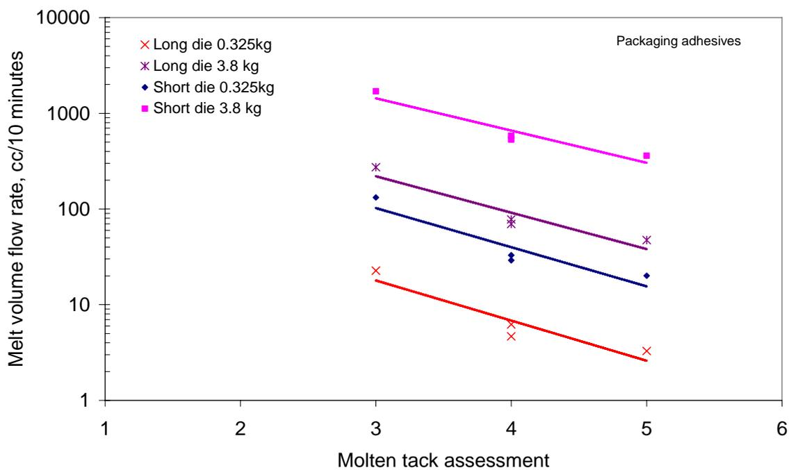
Figure 17: Correlation of molten tack assessment with melt volume flow rate parameters
