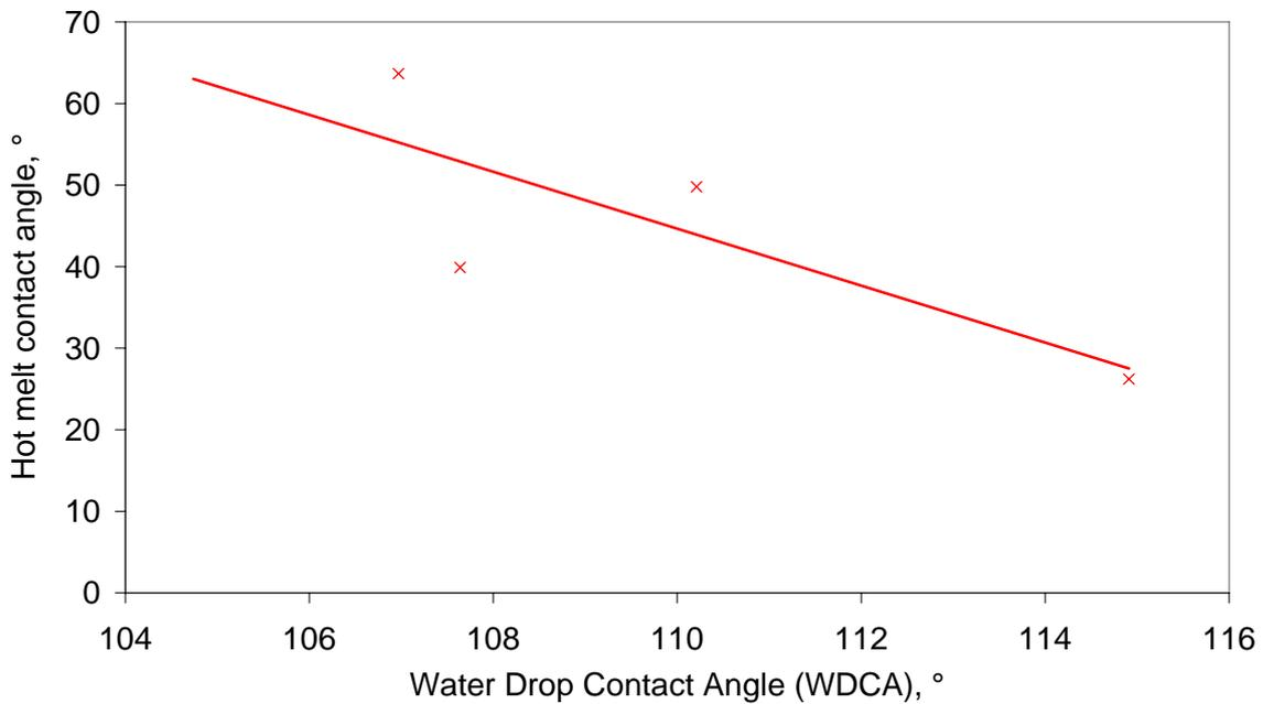
**Figure 10b: Relationship between the measured contact angles of several hot melt adhesives on a PET surface at 100 °C with water drop contact angle (room temperature)**
