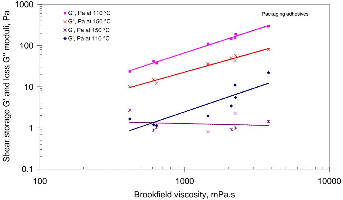
Figure 7: Correlation of rheological properties with the Brookfield viscosity
