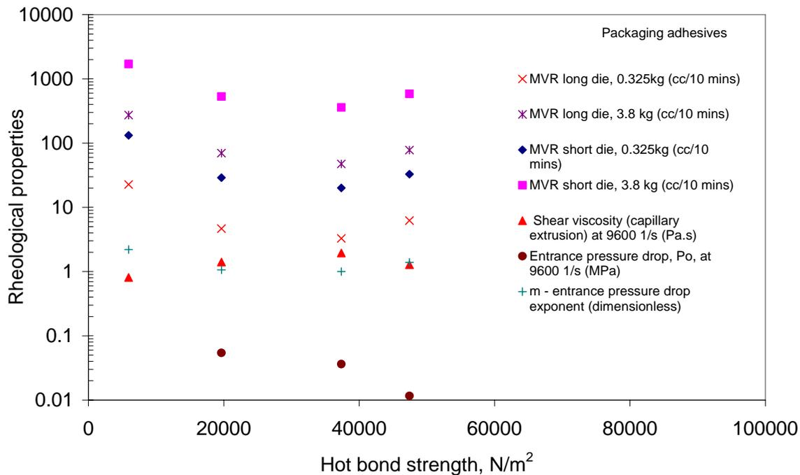
**Figure 14: Correlation of rheological properties with hot bond strength (tack)**
