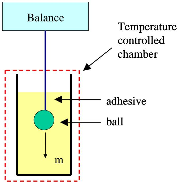
**Figure 1: Density measurement by Archimedes' principle**
