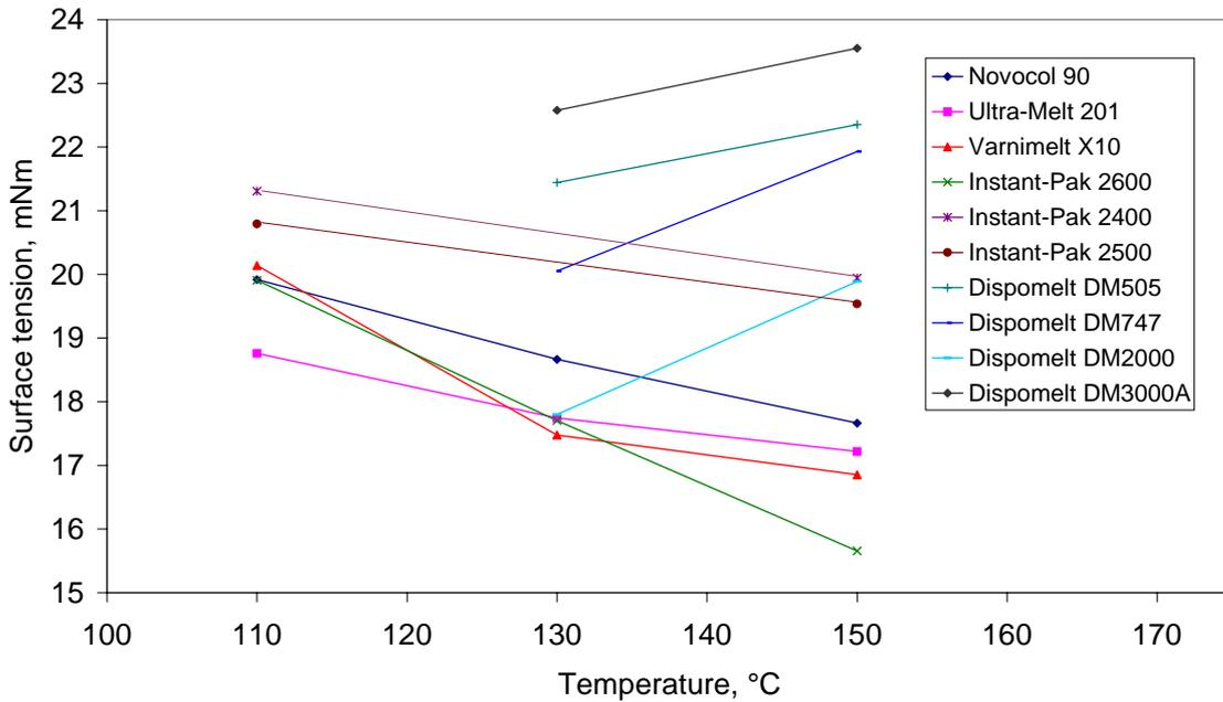
**Figure 4: Surface tension results for packaging and Dispomelt adhesives**
