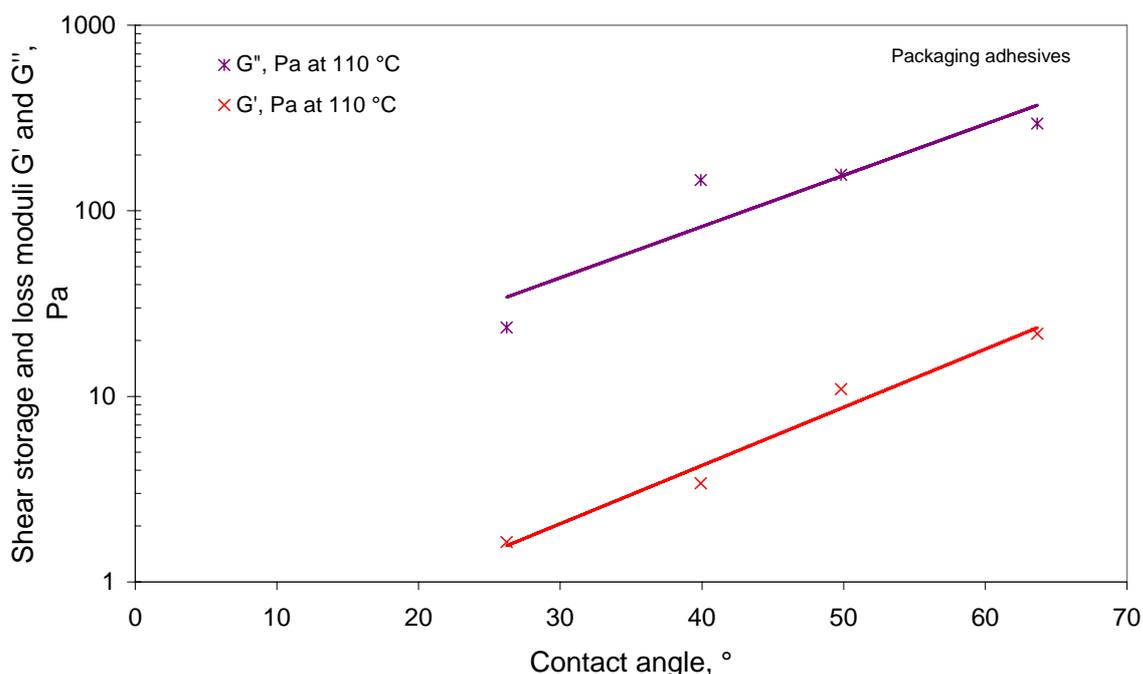
**Figure 11: Apparent correlation between wetting (hot melt contact angle) and viscoelastic properties**
