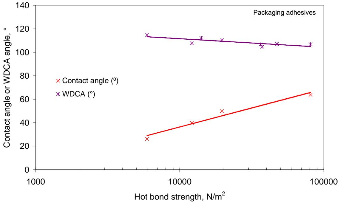
**Figure 12: Correlation of hot melt contact angle and WDCA angle with hot bond strength (tack)**
