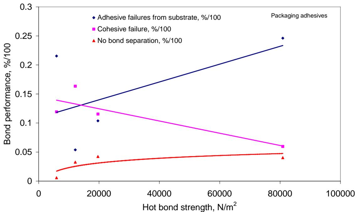
**Figure 16: Correlation of bond performance with hot bond strength (tack)**
